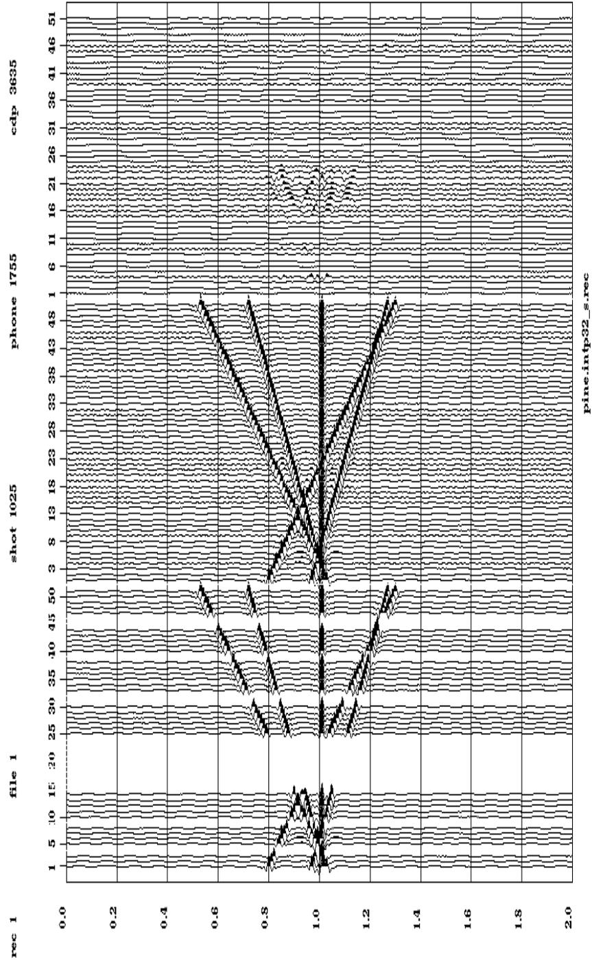
Fig. 8. Missing trace interpolation with the least-squares f-x prediction. The figure is this same as in Figure 7, except the second record is the result of applying the least-squares prediction, and the last record is the least-square prediction.
