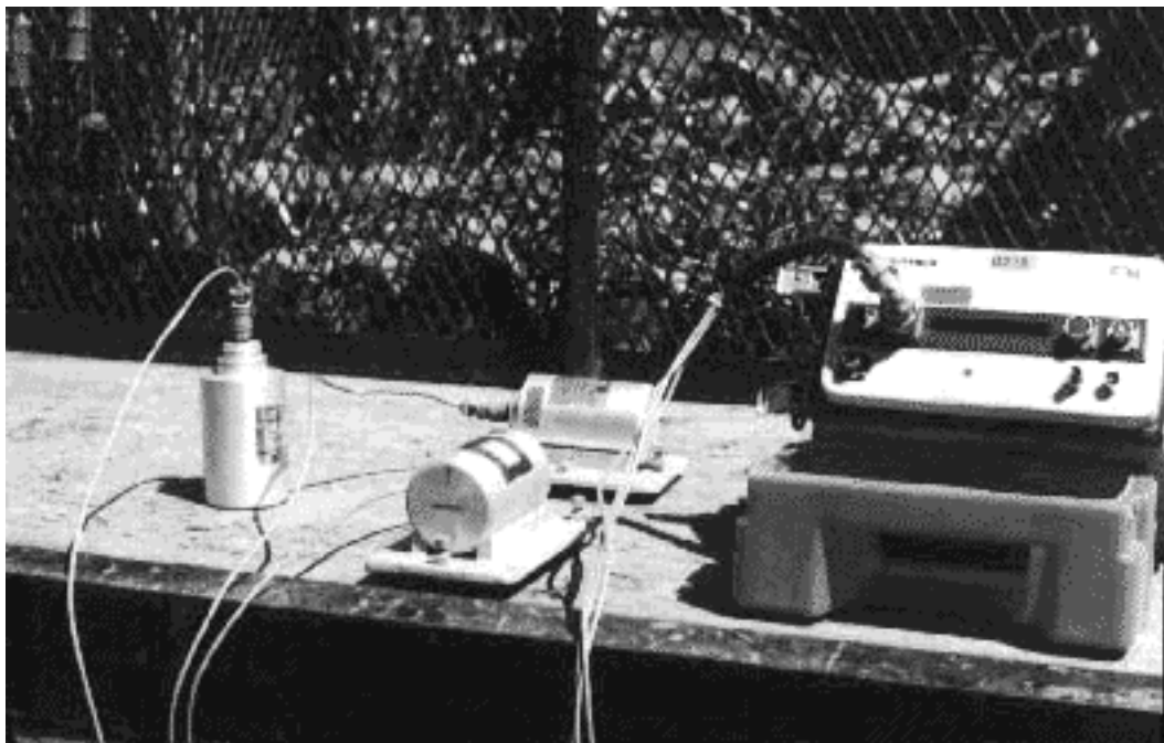
Fig 7. This photo shows the L-4A 2 Hz geophones, set up in a 3-component configuration. The phones are beside a Scintrex 3 channel recorder.
