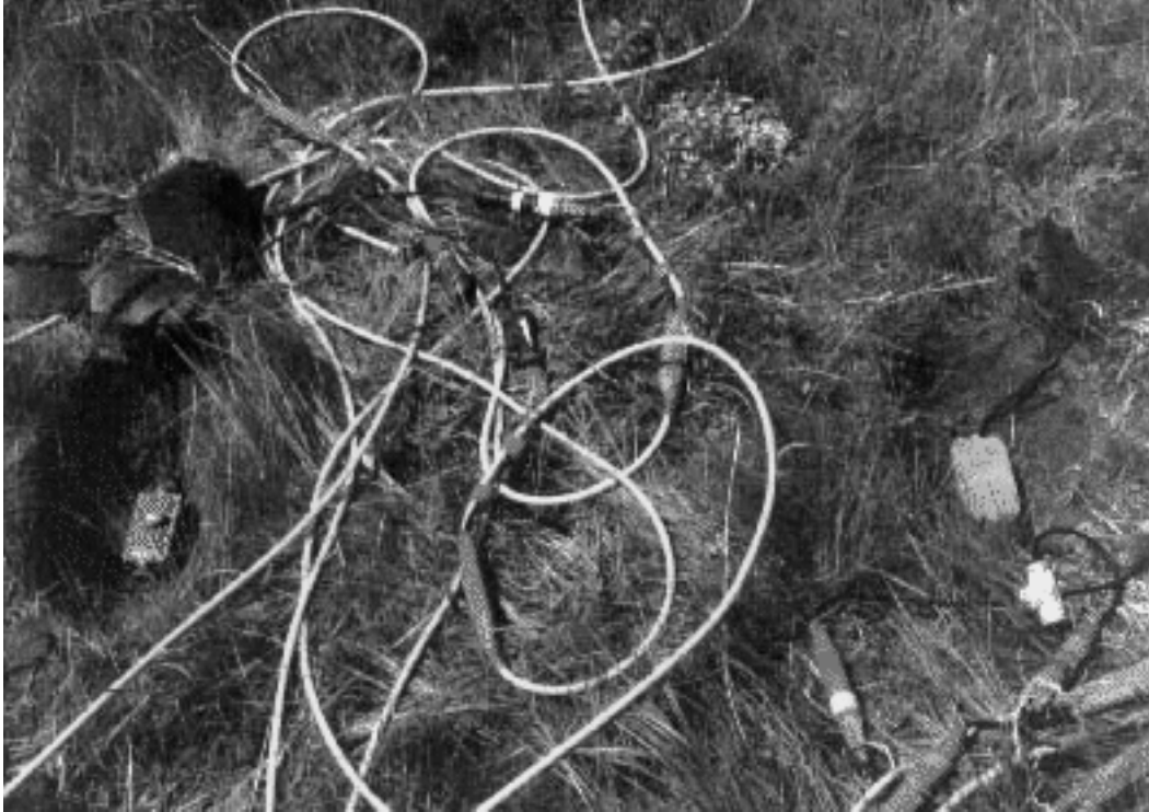
Fig. 6. The LRS-1033 3-Component 10 Hz geophone (on the left) planted in a 30 cm deep hole. The L-28 3-Component 4.5 Hz geophone (on the right) which is also in a 30 cm deep hole. The cable between the phones which at the time of deployment was laid straight, has been rearranged by the cattle who share the pasture with our seismic line.
