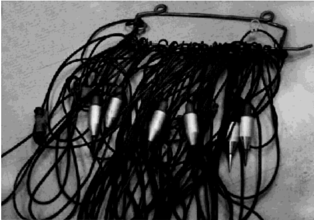
Fig. 5. A string of Oyo Geo-Space Ltd., GS-30CT geophones with marsh cases.
