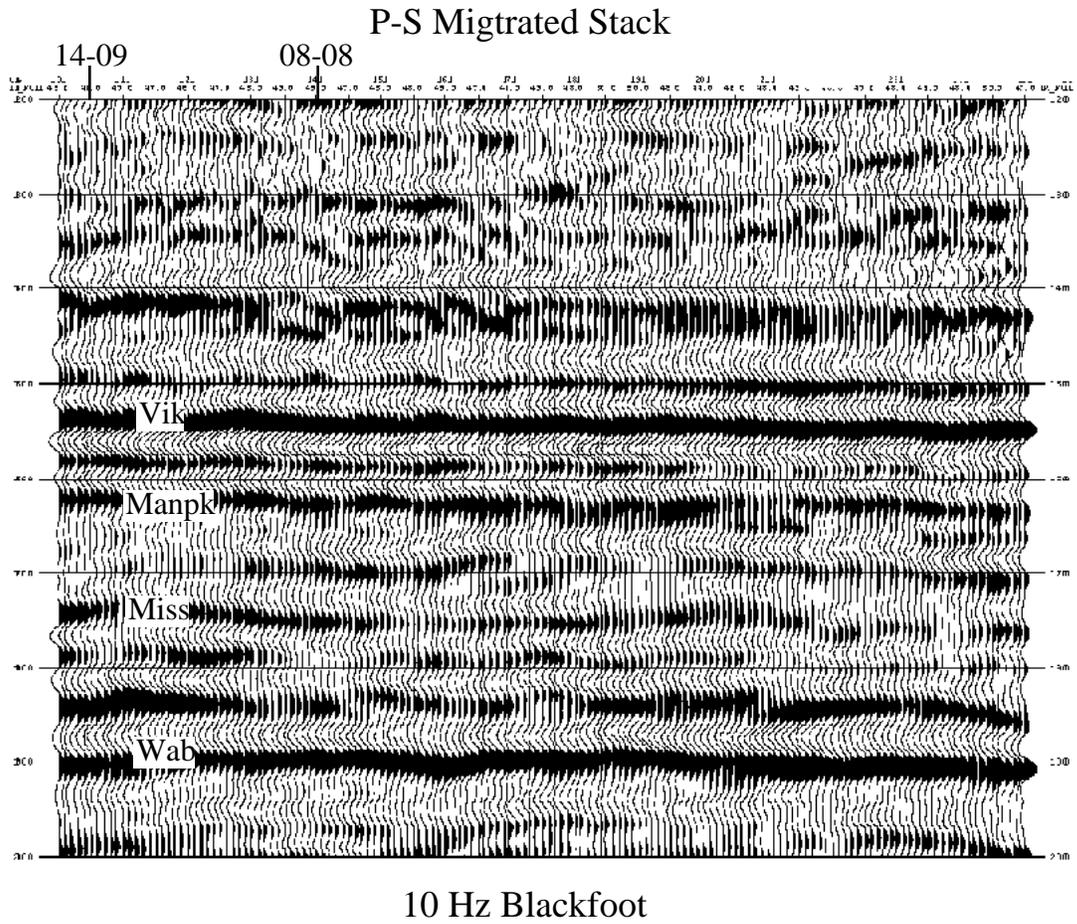
Fig. 4. P-S stack section. FX decon, Migration and signal enhancement all done pre-stack.
