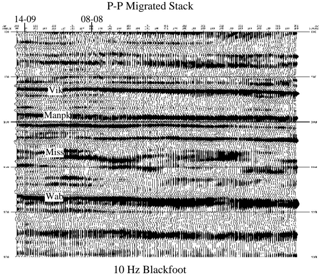
Fig. 1. Vertical component section. This display has been filtered and AGC scaled for viewing only. No AGC scaling was applied prior to inversion. P sonic log locations of wells 14-09 and 08-08 are indicated. The Glauconitic Channel (Miller et al, 1995) can be seen to the right of the 08-08 well, at the Miss level.
