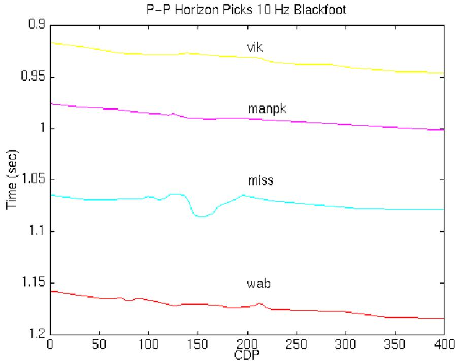
Fig. 5. Horizon picks for P-P data. These, in conjunction with the corresponding P-S horizon picks, were used to correlate P velocity and S-velocity estimate to P-S time for P-S inversion.
