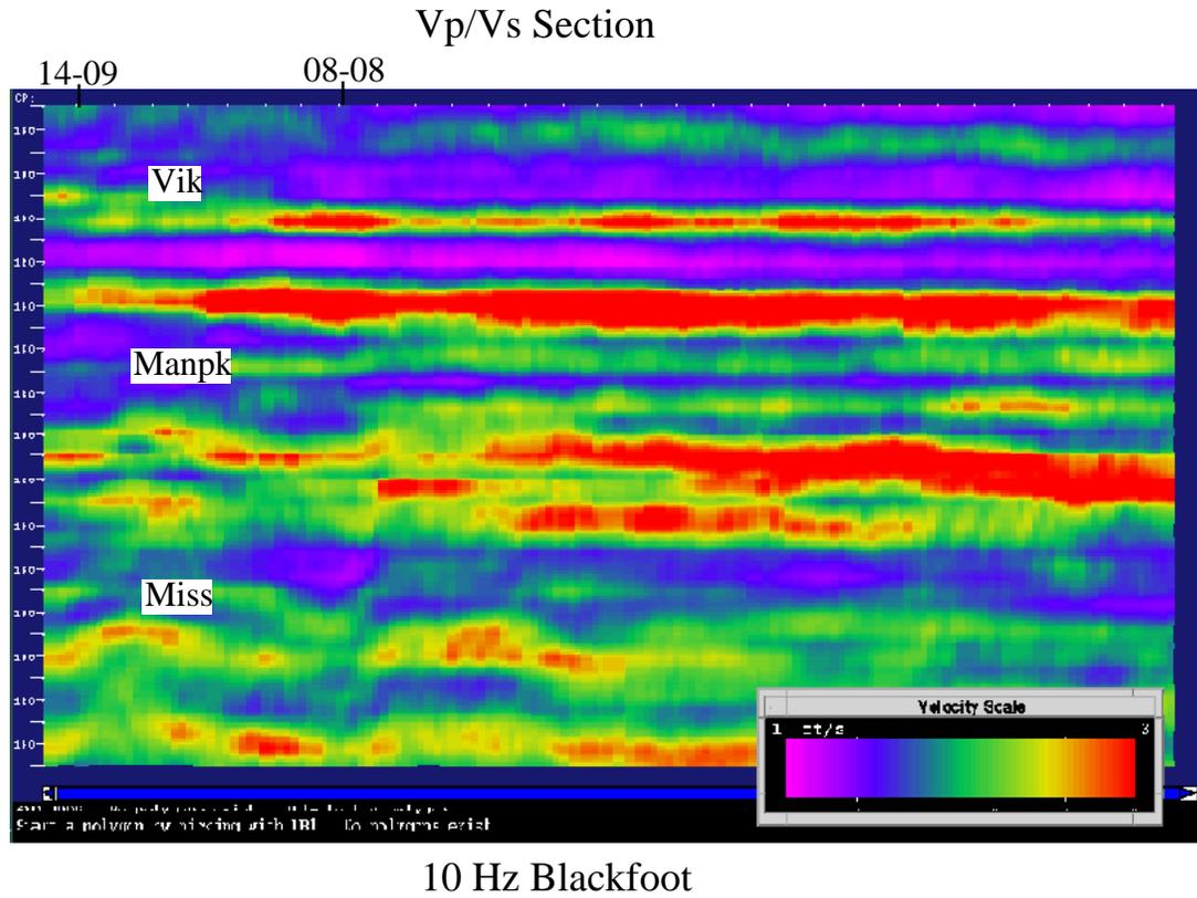
Fig. 9. Close up for Figure 8, with Vp/Vs ranges clipped at 3.0. Vp/Vs decrease visible across the target zone.
