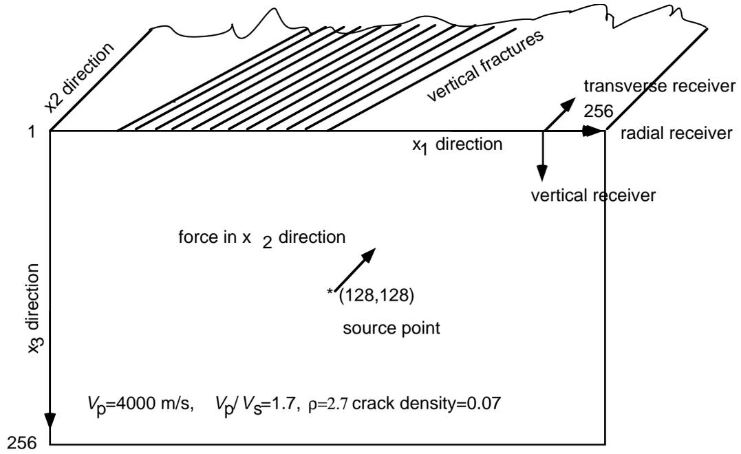
Figure 1. Illustration of model 1.
