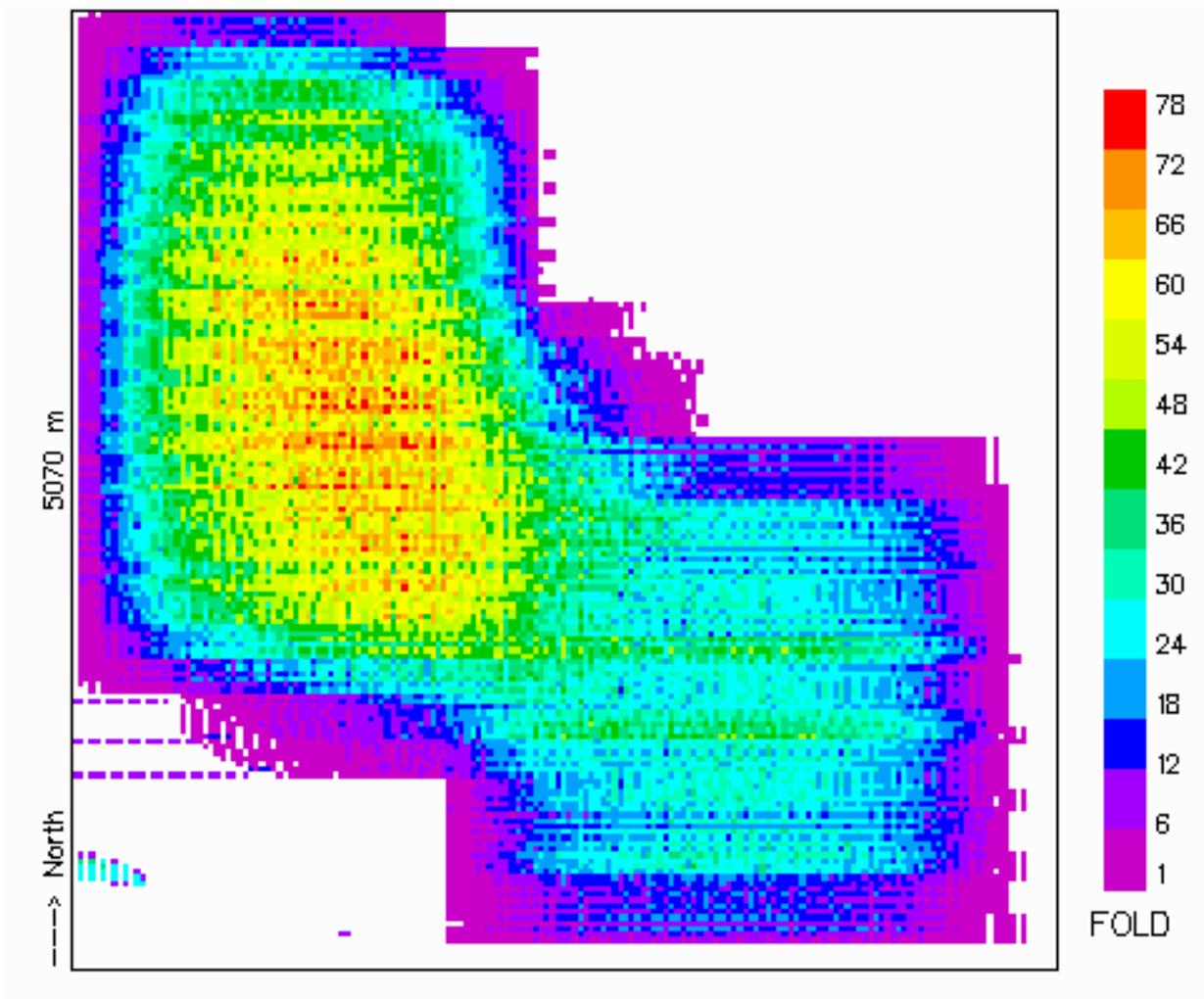
Fig 11. Post-survey depth-variant P-S fold distribution. Bin size 30 m x 30 m. Glauconitic target level.
