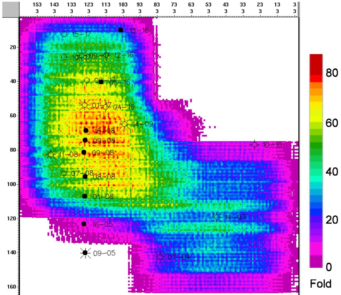
Fig 13. Processed stacking P-S fold distribution at 1500 ms. Bin size 30 m x 30 m. Glauconitic target level.
