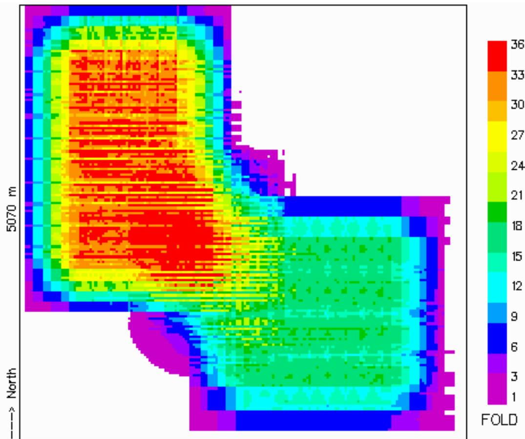
Fig 7. Post-survey P-P fold distribution. Bin size 30 m x 30 m.
