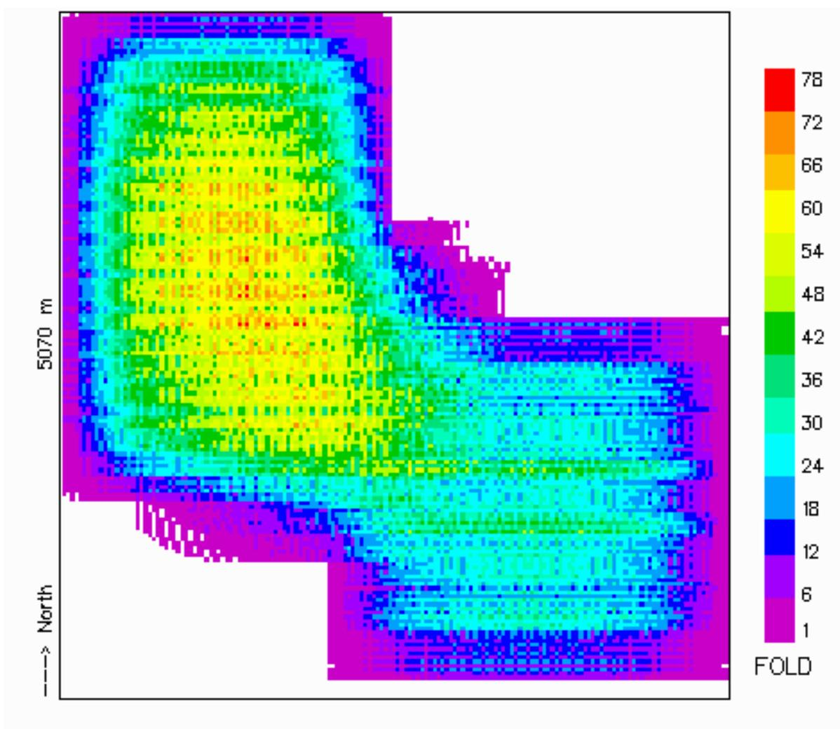
Fig 10. Pre-survey depth-variant P-S fold distribution. Bin size 30 m x 30 m.
