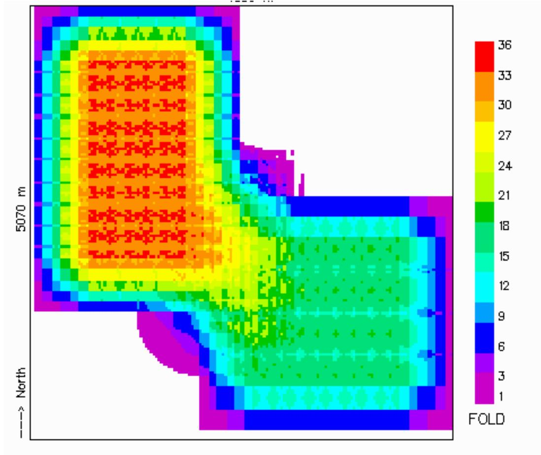
Fig 6. Pre-survey P-P fold distribution. Bin size 30 m x 30 m.
