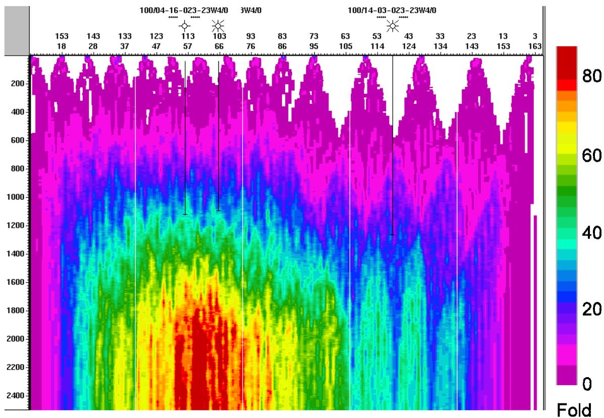
Fig. 16. Processed stacking fold for P-S data from NW-SE diagonal line through survey volume. Trace spacing is 30 m.
