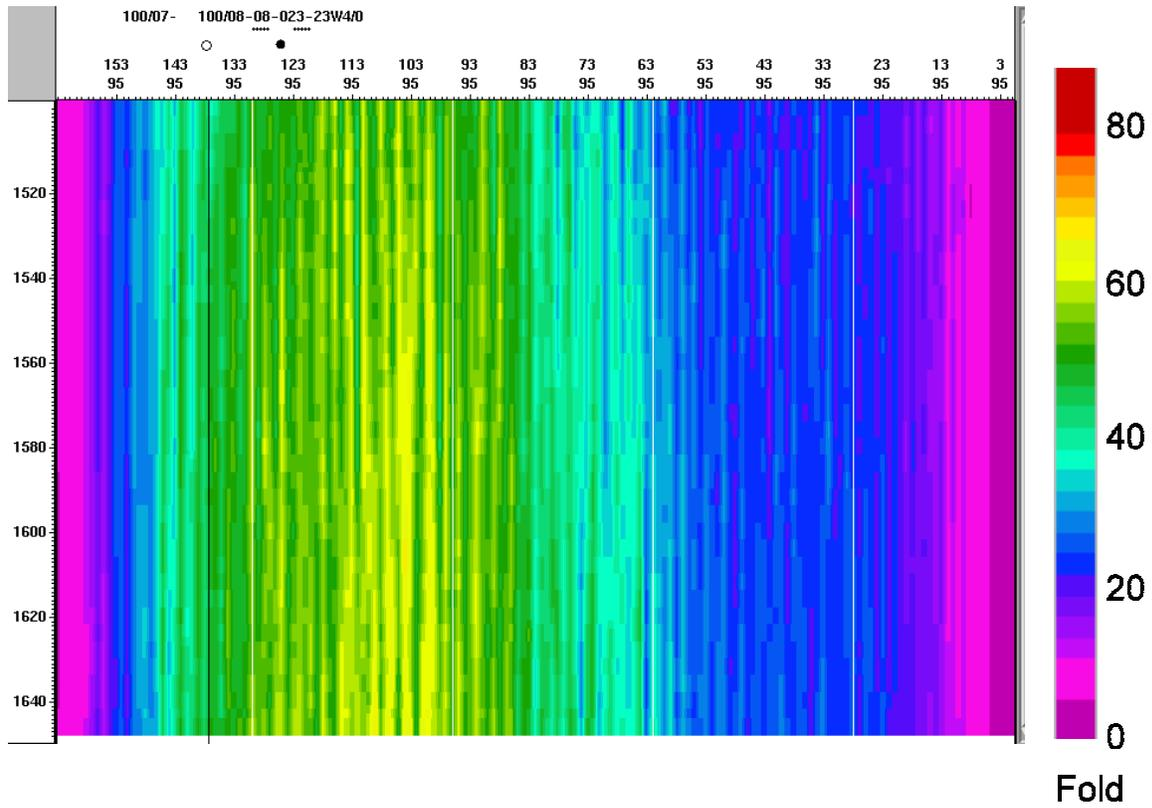
Fig. 19. Detail of processed stacking fold for P-S data from in-line 95 through survey volume at Glauconitic reservoir level. Trace spacing is 30 m.
