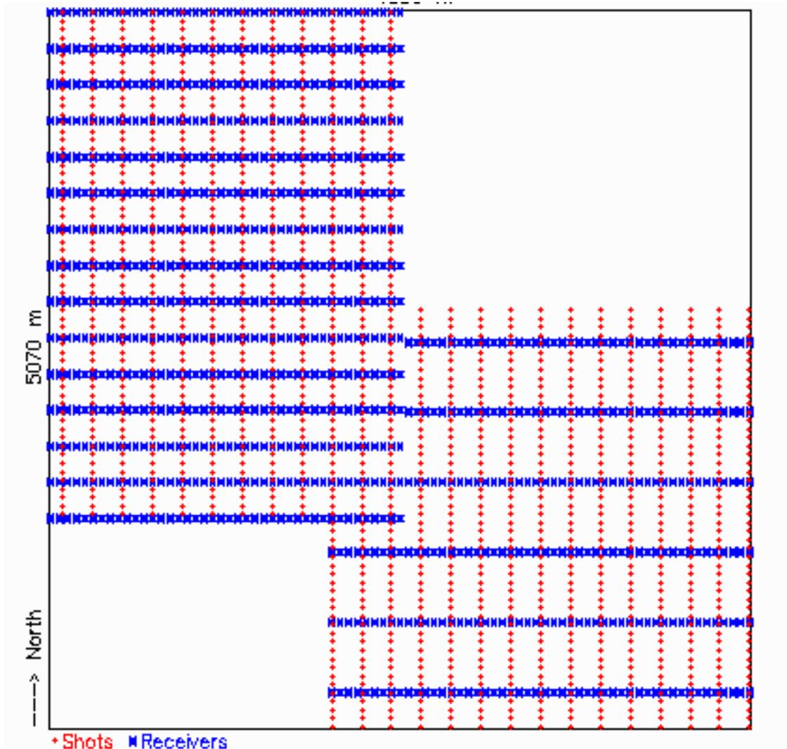
Fig. 2. Pre-survey source and receiver line geometry for Blackfoot 3C-3D program
