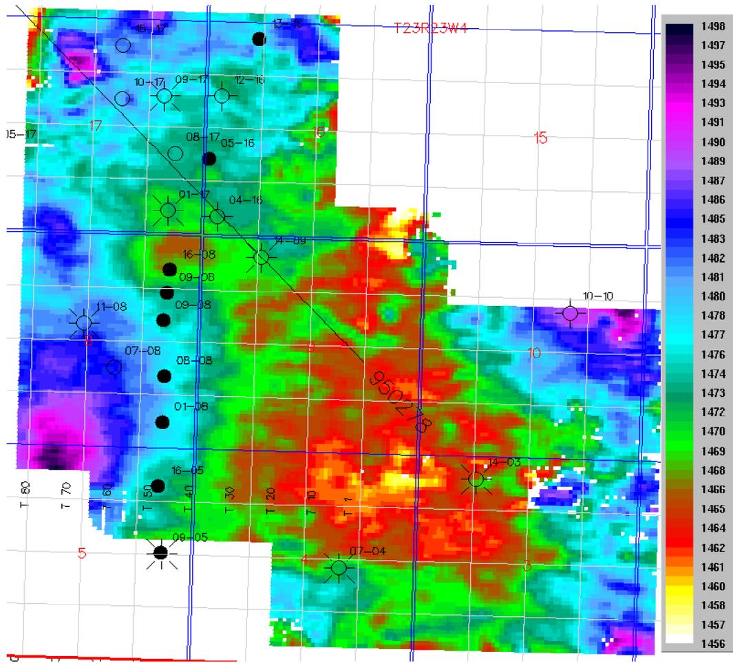
Fig. 10b. P-S time structure, Mannville event, the red/yellow color zones indicate the structural high. Color bar is reflection time (ms).
