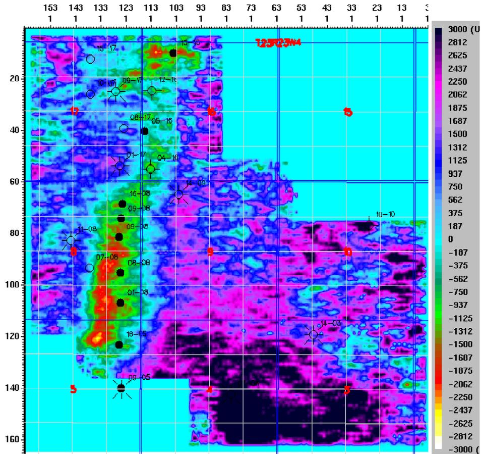
Fig. 13b. *P-S* time slice section at 1590 ms (flattened at Mannville), equivalent to the level of a channel just above the Mississippian surface. The greenish color running north-northeast to south on the left part of the image is evident. Color bar is amplitude.
