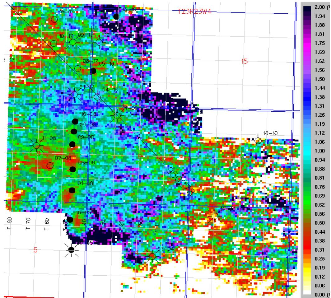
Fig. 19b. Amplitude ratio of  $P$ - $S$  versus  $P$ - $P$  on Lower Mannville event. The bluish purple color indicates the  $P$ - $S$  amplitude is higher than the  $P$ - $P$  amplitude.
