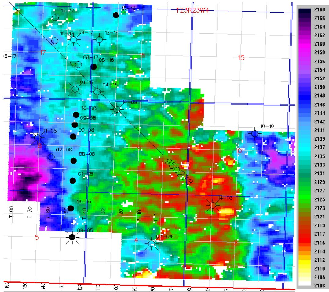
Fig. 5b. P-S time structure map, basal Cambrian time. The red/yellow area shows a horst block in the south-central part of the area. More local variations are visible than shown in figure 5a. Color bar is reflection time (ms).
