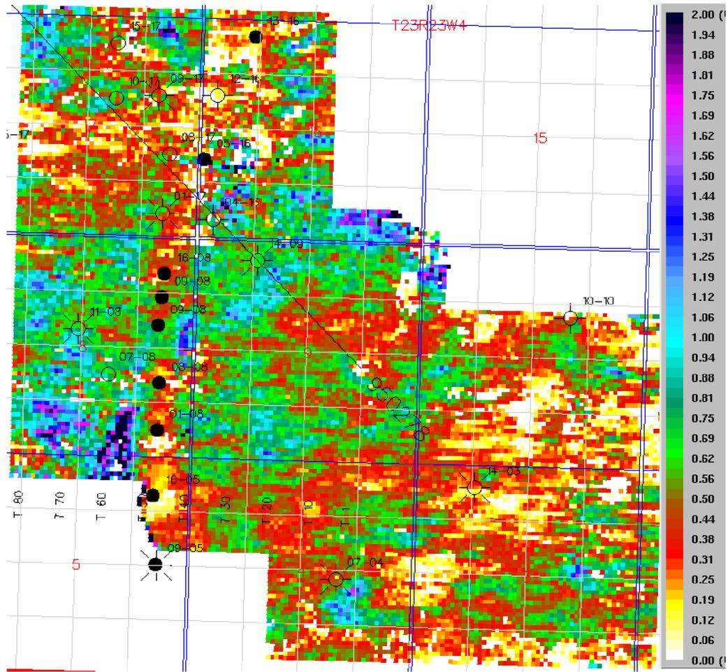
Fig. 19a Amplitude ratio of  $P$ - $S$  versus  $P$ - $P$  on Top Channel event
