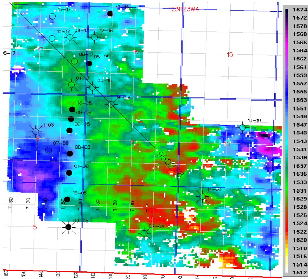
Fig. 9b. P-S time structure, Lower Mannville event. Color bar is reflection time (ms).
