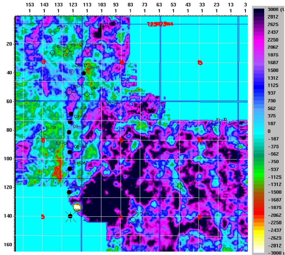
Fig. 13a. *P-P* time slice section at 1080 ms (flattened at Mannville). This time slice cuts the volume at about the level of a possible Detrital channel just above the Mississippian surface.
