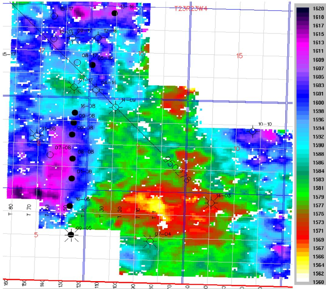
Fig. 7b. P-S time structure, Mississippian event. Note that the structural relief marked in green extends into section 17 through the corner of sections 8, 9, 16 and 17. Color bar is reflection time (ms).
