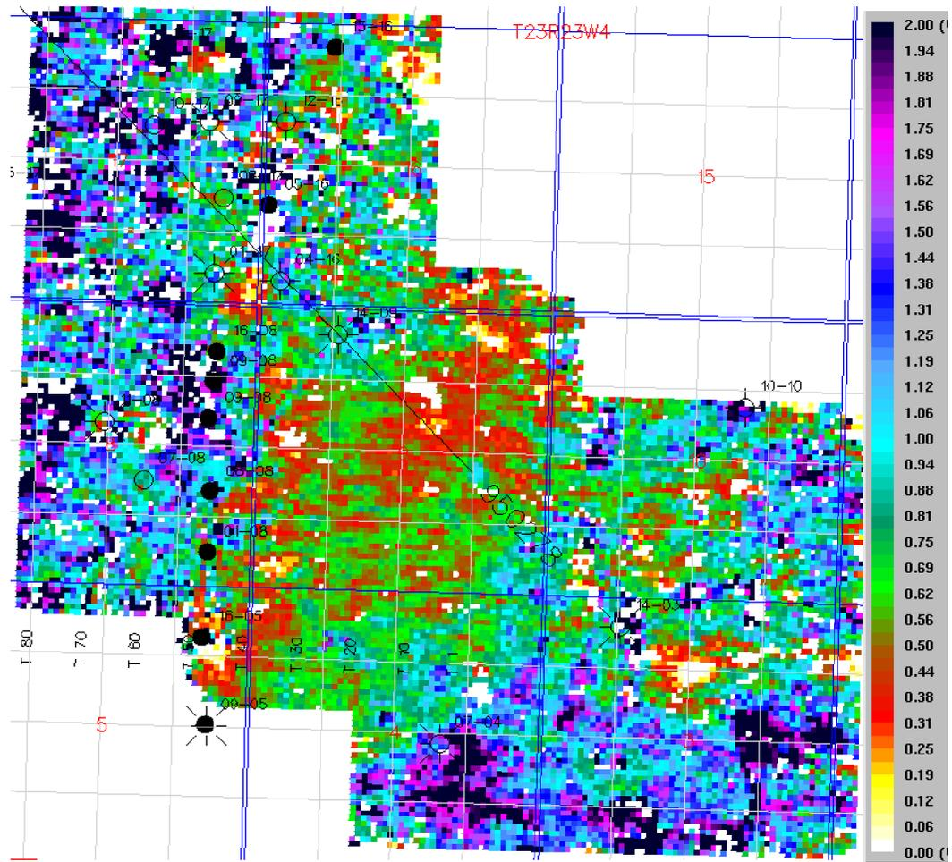
Fig. 19c. Amplitude ratio of  $P$ - $S$  versus  $P$ - $P$  on Mississippian event. Note that in the central part of the survey area,  $P$ - $S$  amplitude is less than  $P$ - $P$  amplitude. The edge coincides with the well controls, is it where the lithology changes from sand to shale?
