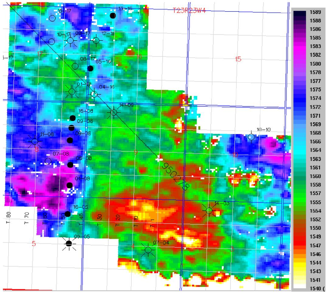
Fig. 8b. *P-S* time structure, top channel level. The greenish color (high relief) surrounded by the purple color (low in relief) in section 17 formed an updip seals for reservoirs in the south. Color bar is reflection time (ms).
