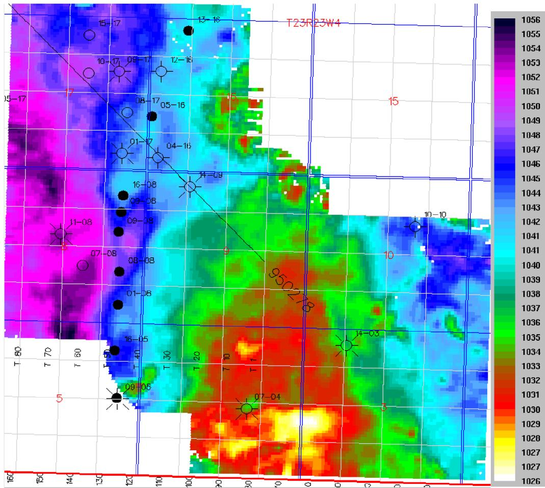
Fig. 9a. *P-P* time structure, Lower Mannville event, the red/yellow color zones indicate the structural high. Color bar is reflection time (ms).
