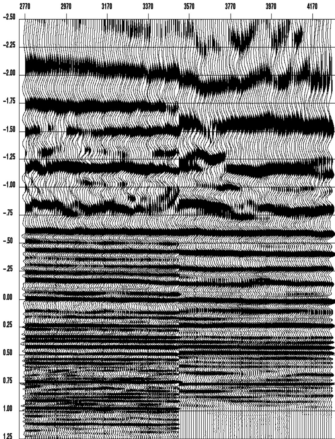
Fig. 4. Events are matched reasonably well in the log-domain after P-P DMO stack (the first half of record) are shifted by 0.4 downwards.
