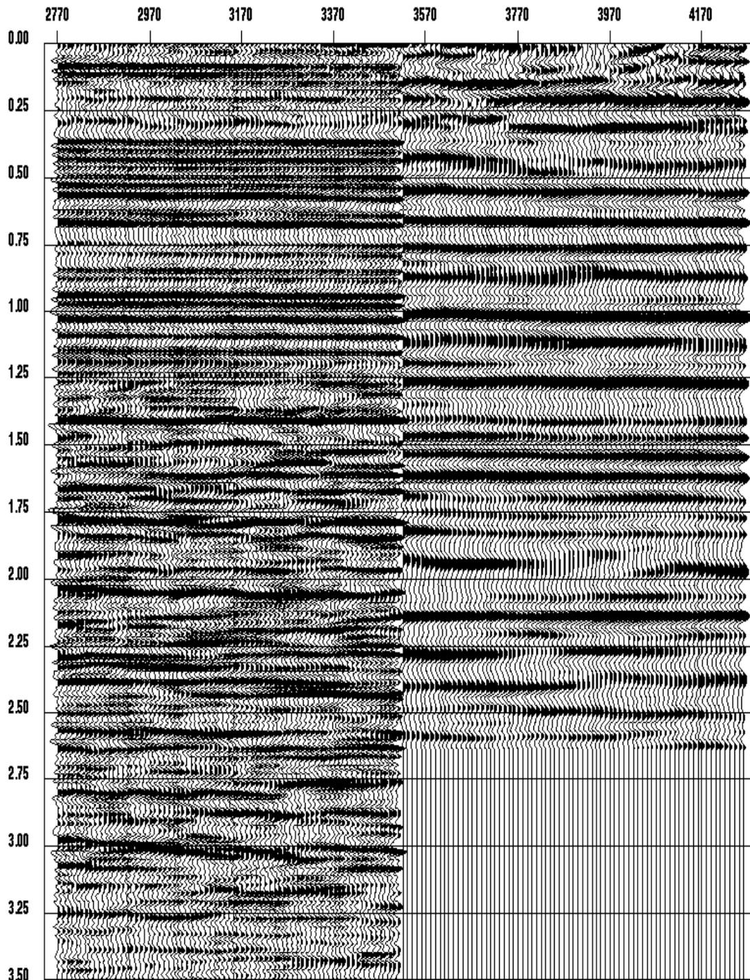
Fig. 2. Input to the log-method. The first half of record is P-P DMO stack shifted by 0.479 seconds upwards, and the second half is P-S DMO stack shifted by 0.864 seconds upwards, so that the event on both stacks are line-up at zero second.
