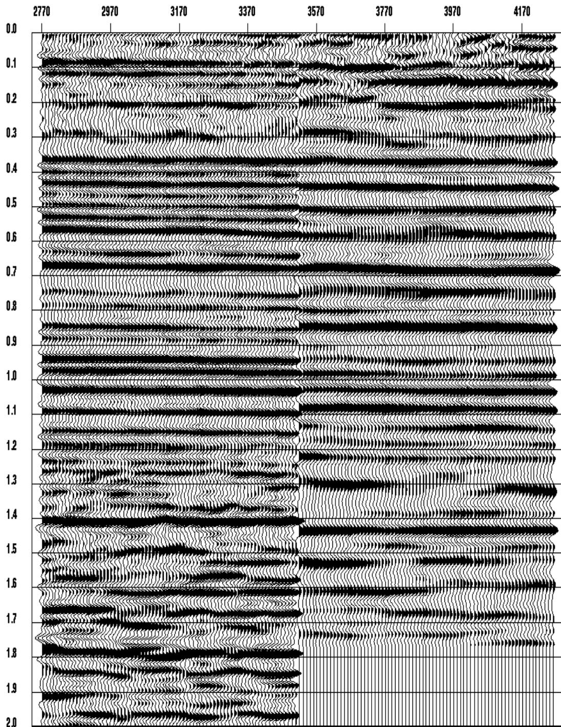
Fig. 5. P-P and P-S match in P-P time. The P-S data on the right has been squeezed with  $\gamma_{ps} = 1.98$  to match P-P data on the left.
