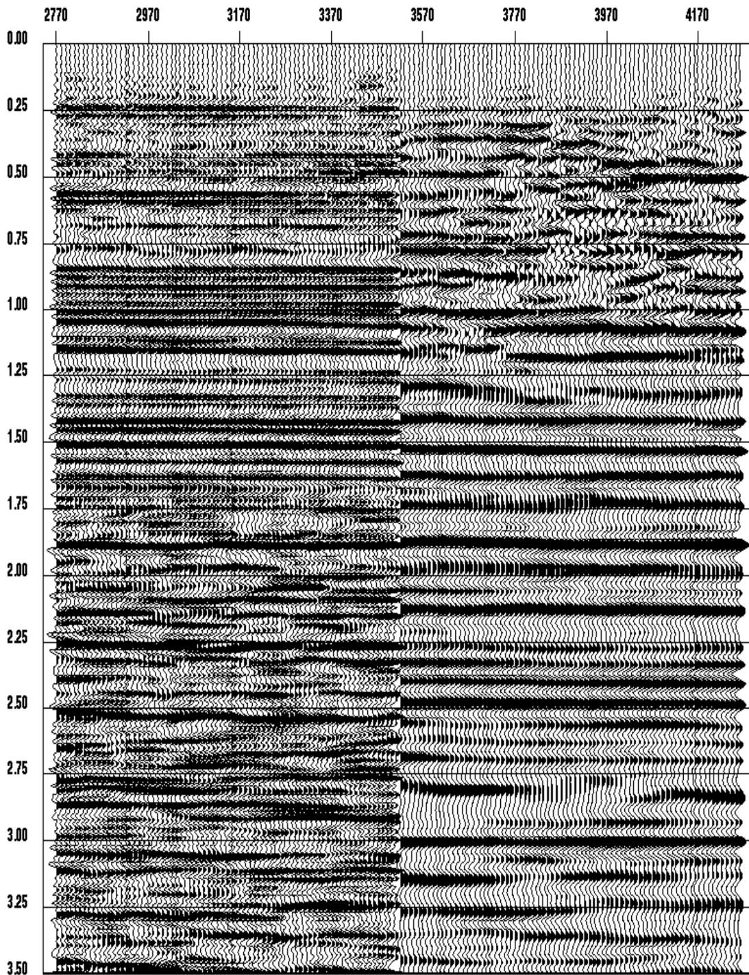
Fig. 1. P-P DMO and P-S DMO Stacks. The first half of record is P-P DMO stack from stations 2770 to 3510, the second half of record is P-S DMO stack from stations 3520 to 4260.
