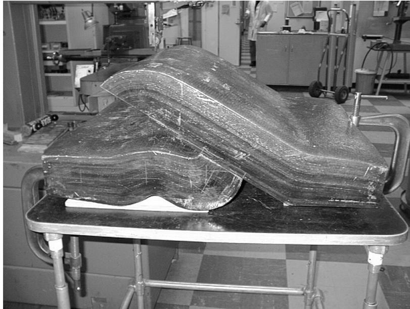
Fig 2. Photograph of the anisotropic thrust model.
