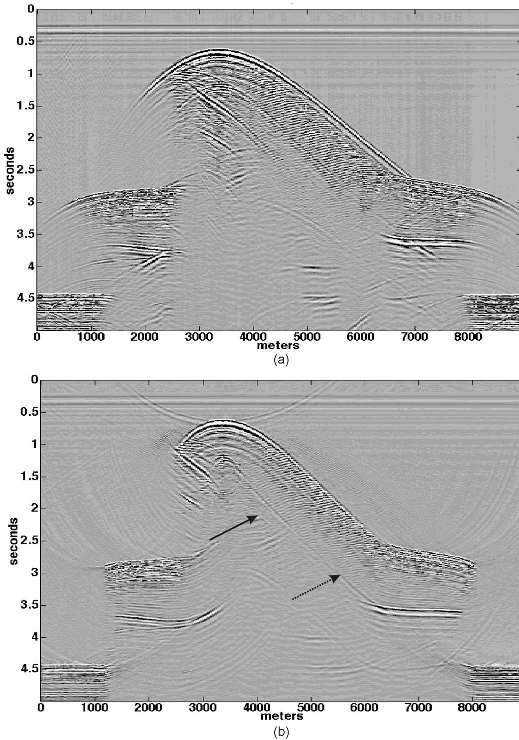
Fig. 6. Raw (a) and migrated (b) data from the survey across the anisotropic thrust model with target rod C (identified by solid arrow). The migration was performed using a constant velocity of 1480 m/s (water velocity). Location of rod C is shown in Figure 1. Dashed arrow is fault plane reflection
