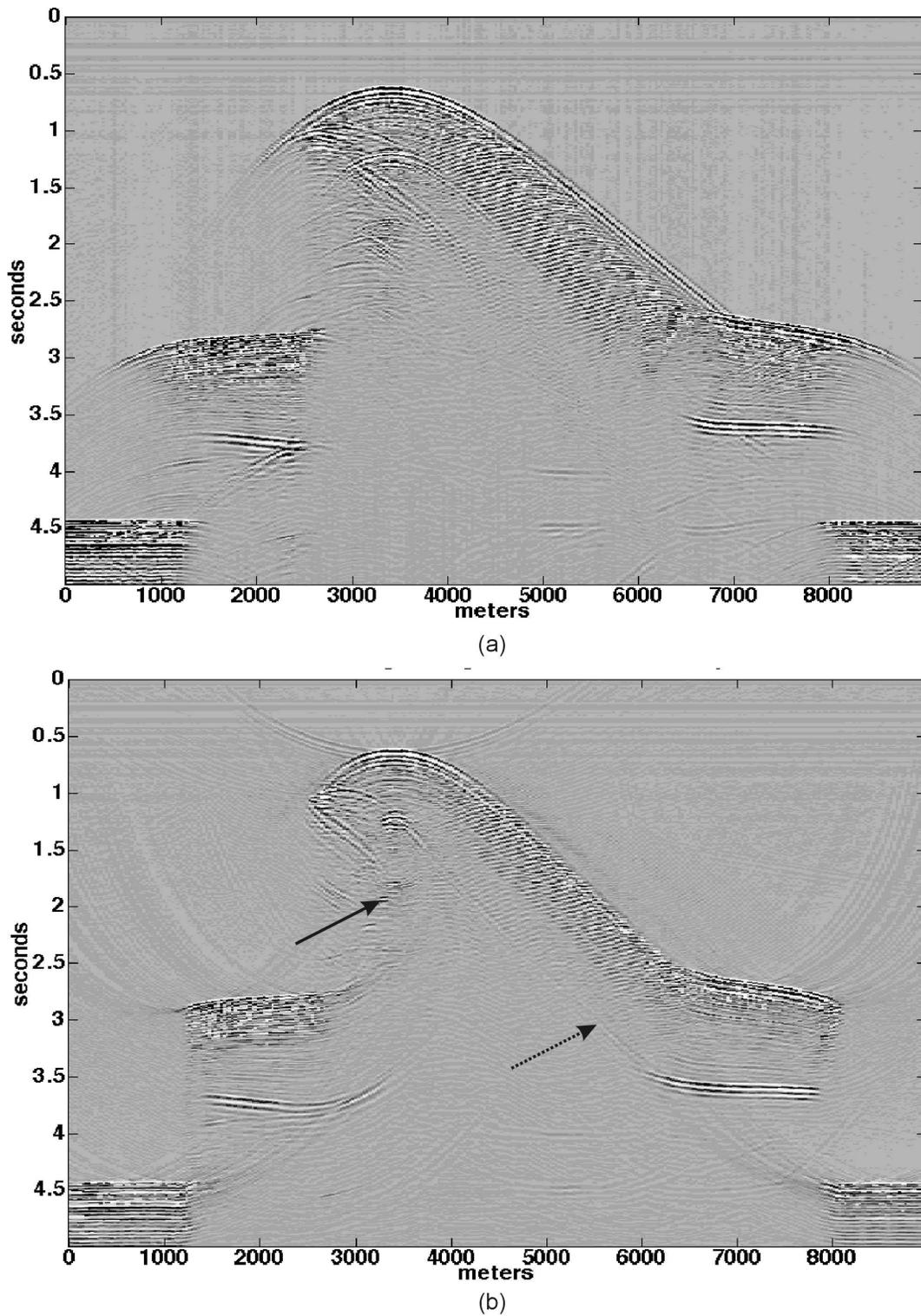
Fig. 4. Raw (a) and migrated (b) data from the survey across the anisotropic thrust model with target rod A (identified by solid arrow). The migration was performed using a constant velocity of 1480 m/s (water velocity). Location of rod A is shown in Figure 1. Dashed arrow is fault plane reflection.
