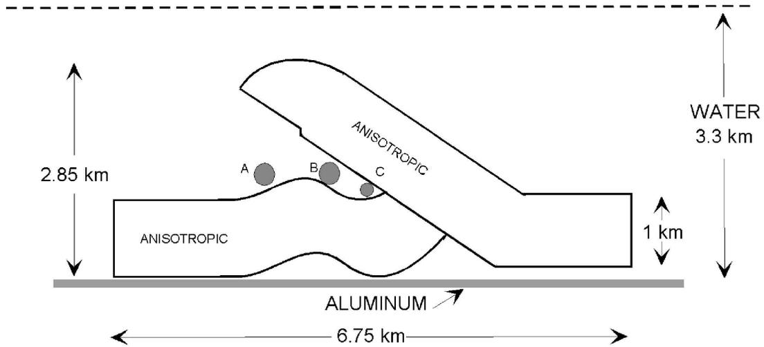
Fig. 1. Schematic cross-section of the anisotropic thrust model. Target rods marked A, B, C were placed in the model for three different surveys.
