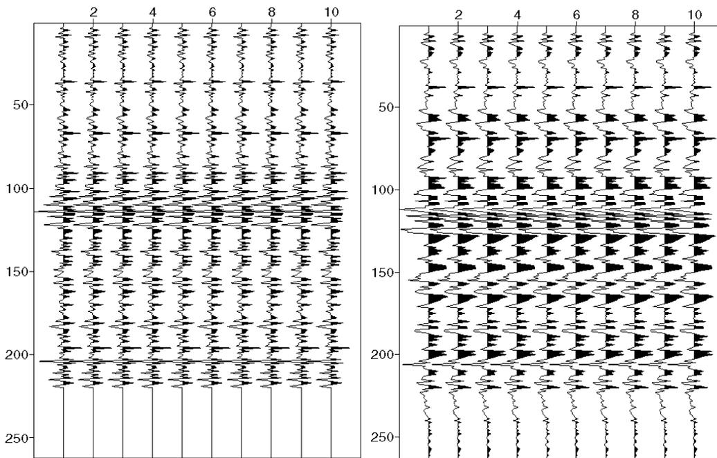
Fig. 17: The actual well-log derived reflectivity series (left) and the Wiener-Levinson reflectivity series estimate (right).
