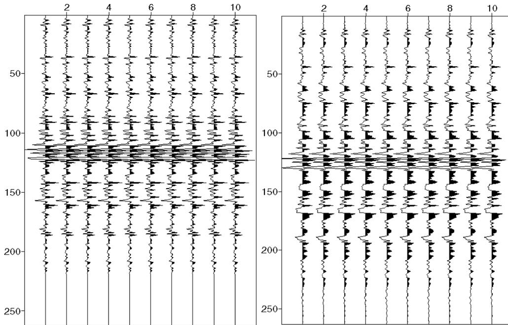
Fig. 9: The actual well-log derived reflectivity series (left) and the Hilbert transform reflectivity series estimate (right).
