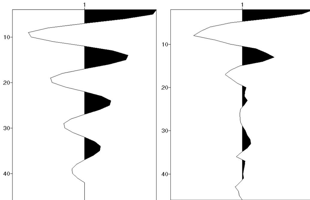
Fig. 13: The model wavelet (left) and a Wiener-Levinson wavelet estimate (right).
