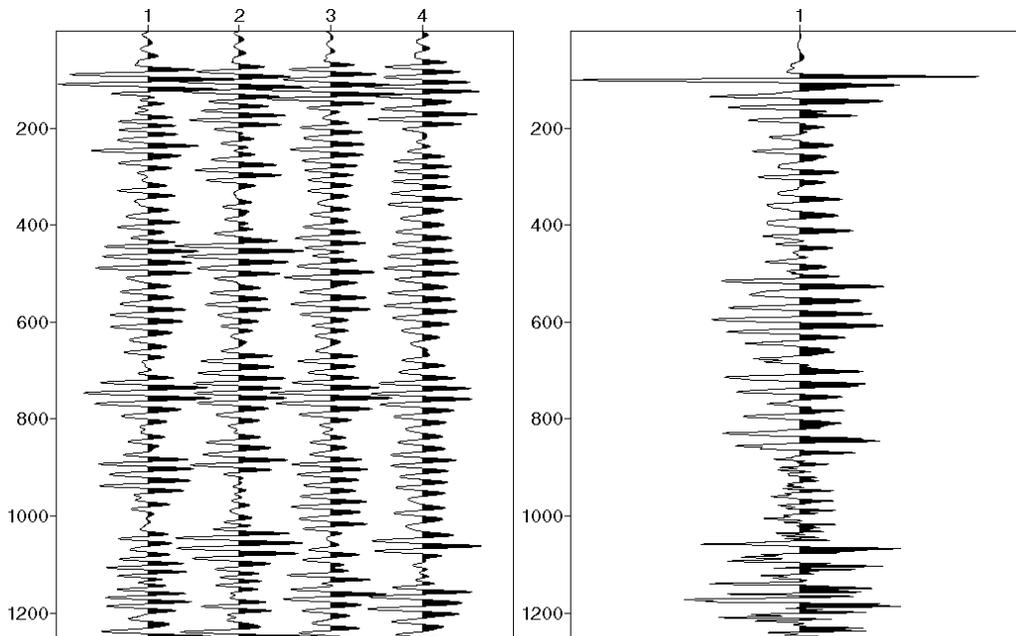
Fig. 34: Near offset surface data and the in-situ measured wavelet (downgoing VSP).
