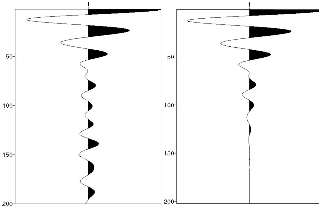
Fig. 38: Near offset trace autocorrelation (left) and Klauder wavelet autocorrelation (right).
