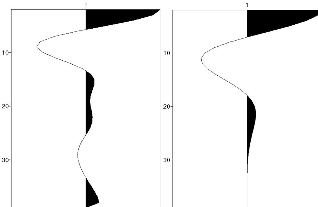
Fig. 21: The trace autocorrelation (left) and the Ricker wavelet autocorrelation (right).
