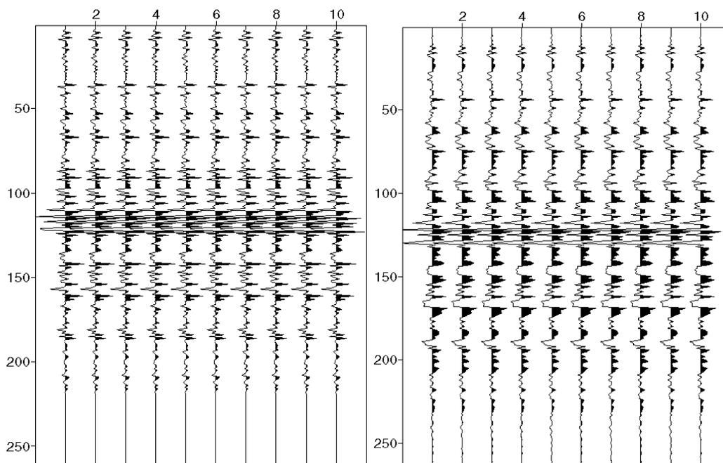
Fig. 8: The actual well-log derived reflectivity series (left) and the Wiener-Levinson reflectivity series estimate (right).
