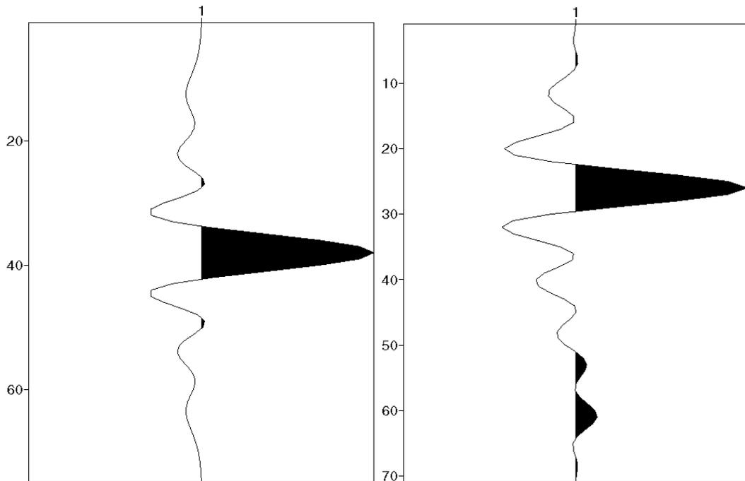
Fig. 23: Ricker wavelet deconvolution (left) and Klauer wavelet deconvolution (right).
