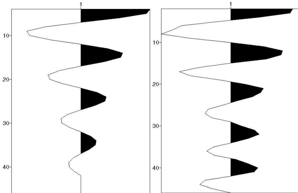
Fig. 5: The model wavelet (left) and a Hilbert transform wavelet estimate (right).
