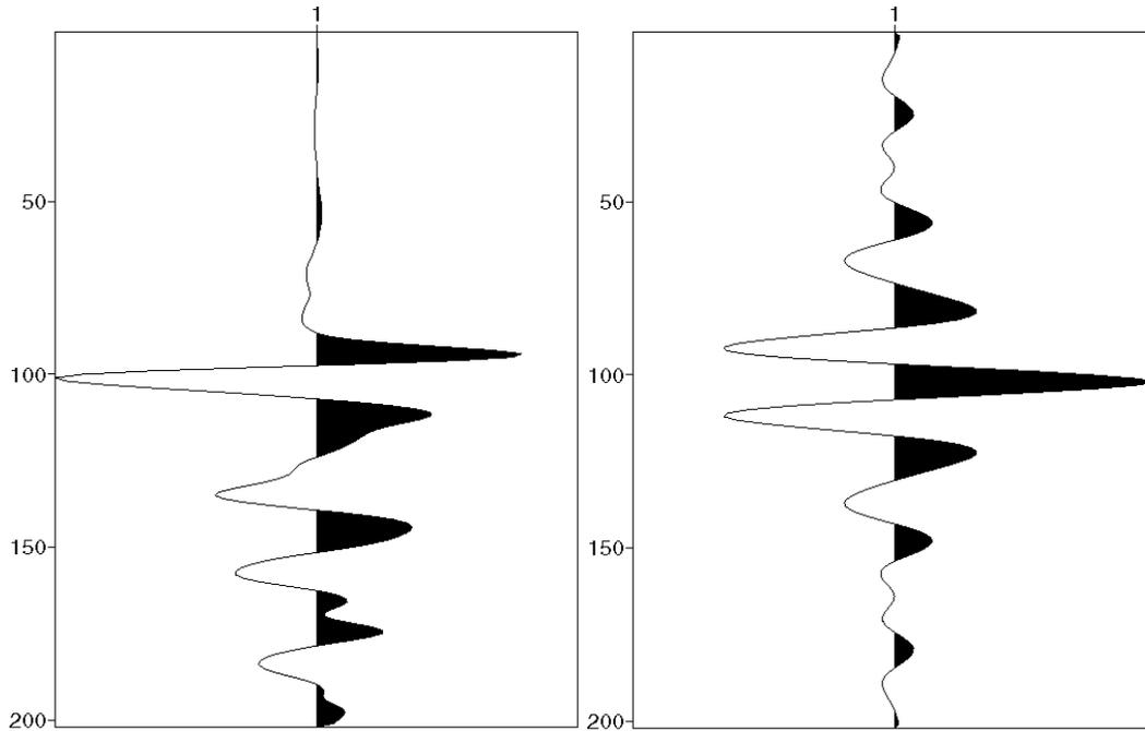
Fig. 36: Truncated measured wavelet (left) and a Klauder zero-phase wavelet (right).
