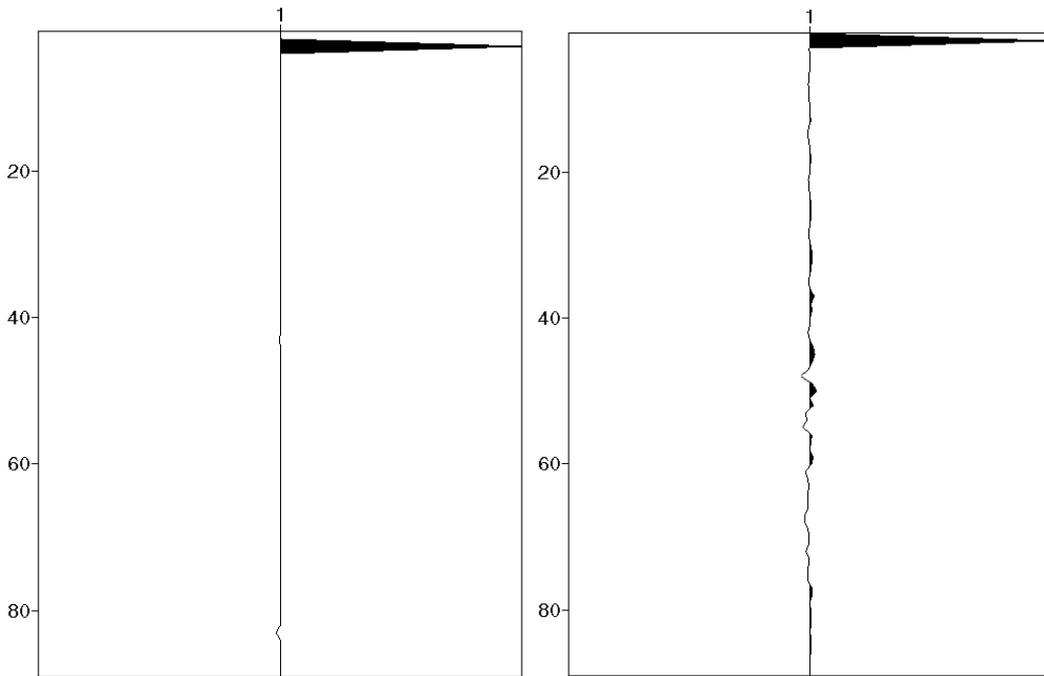
Fig. 15: Model wavelet deconvolution (left) and Wiener wavelet deconvolution (right).
