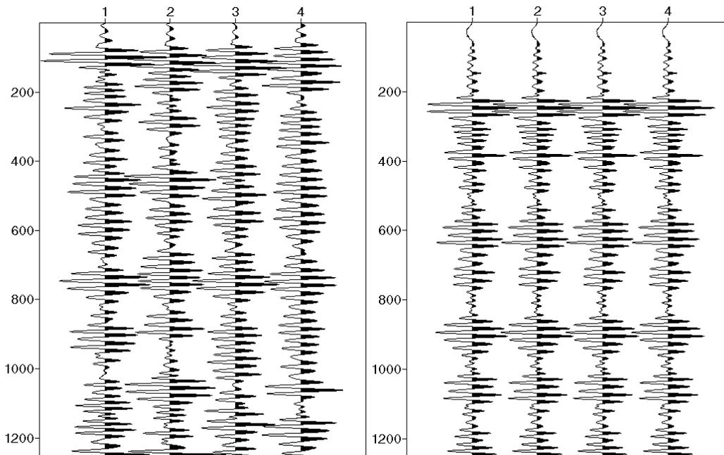
Fig. 42: Near offset traces (left) and their convolution with a truncated filter (right).
