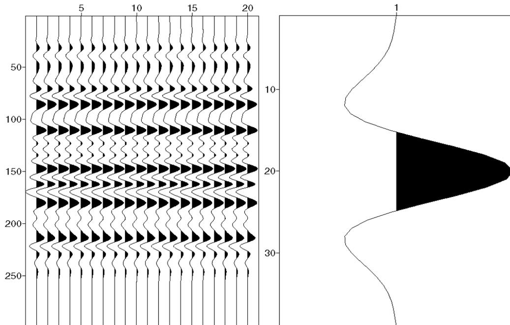
Fig. 27: A zero-phase synthetic trace, with primaries and multiples, and the Ricker wavelet used to create it.
