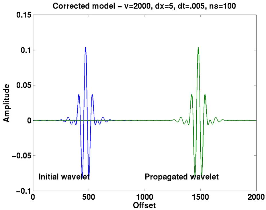
Figure 9: Corrected unstable model, propagated 100 steps. The correction factor (.25, .5, .25) was convolved at each step with the result of the spatial operation.
