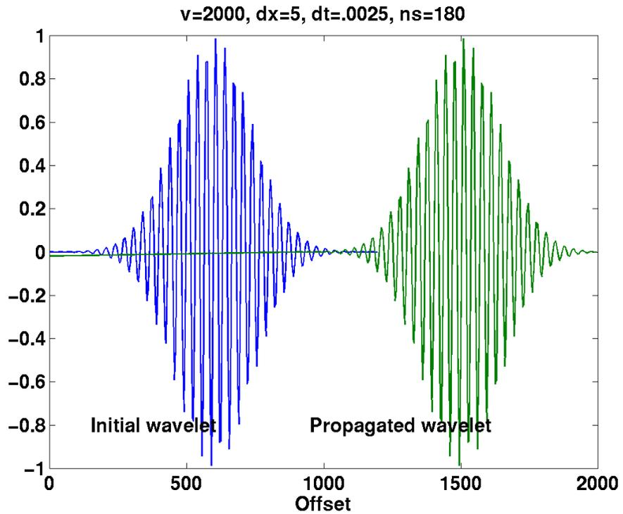
Figure 2. The single frequency wavelet propagated with no dispersion. ( $\Delta t = \Delta x/v$ )
