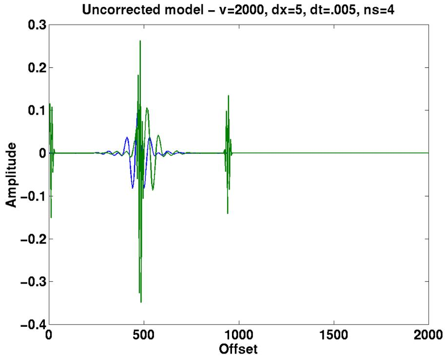
Figure 8: Uncorrected unstable model, propagated only four steps. The signature of unstable parameters appears as high frequencies at three places.
