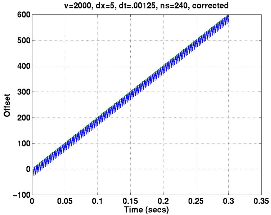
Figure 5: Offset of the propagated wavelet with the correction applied. The straight line on the plot is the real velocity.
