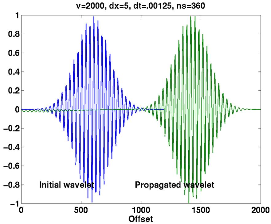
Figure 3: The single frequency wavelet propagated through the same conditions as Figure 2 except with twice as many time steps of half the size. Note lower distance covered.
