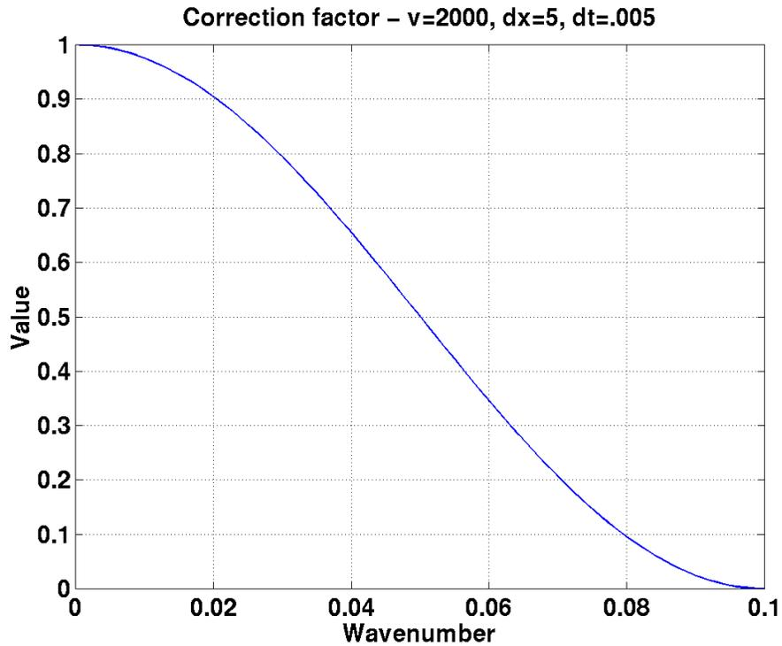
Figure 6: Correction factor in wave number space for an unstable model (with the time sample rate twice as large as it should be).
