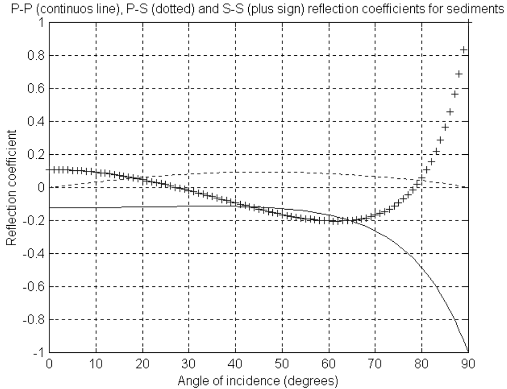
Figure 4 – Mode conversion (reflection) at top of turbidite reservoir for incident down going P- and S-wave. P-P (continuous line), P-S (dotted) and S-S (plus sign) modes. Observe that, below 70^\circ , modes have (relatively) close reflection coefficient values.
