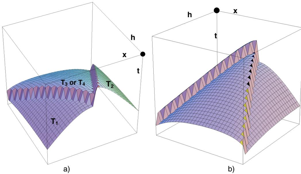
Figure 5. Front a) and rear b) perspective views of the prestack surface where a scatterpoint lies below a step change in surface elevation.
