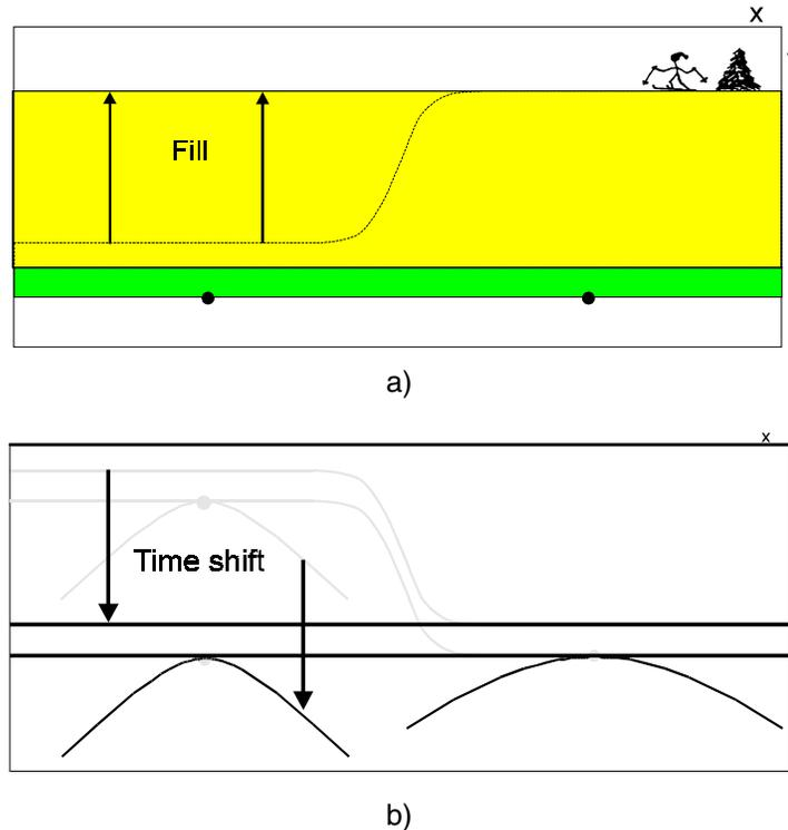
Figure 2. The maximum elevation datum showing: (a) the filled valley; and (b) the time section.
