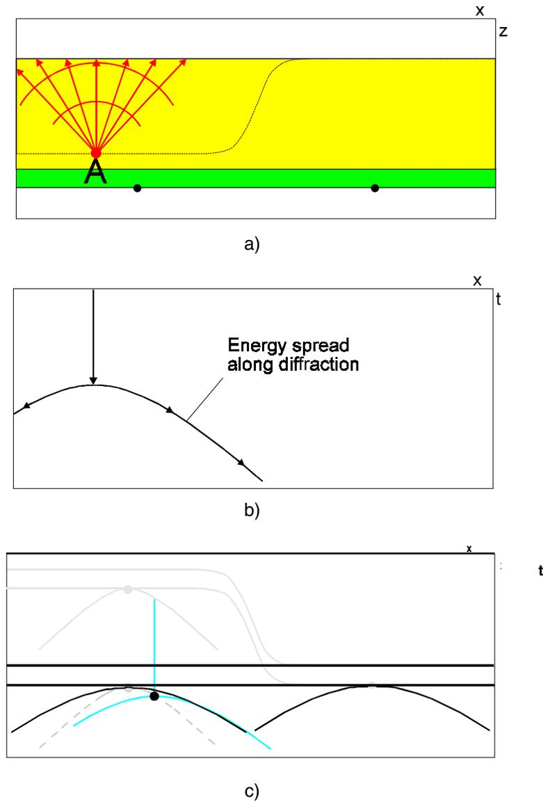
Figure 3. Wave equation datum modelling with: (a) the geological structure; (b) the shape of the dispersion diffraction; and (c) the time response at the new datum.
