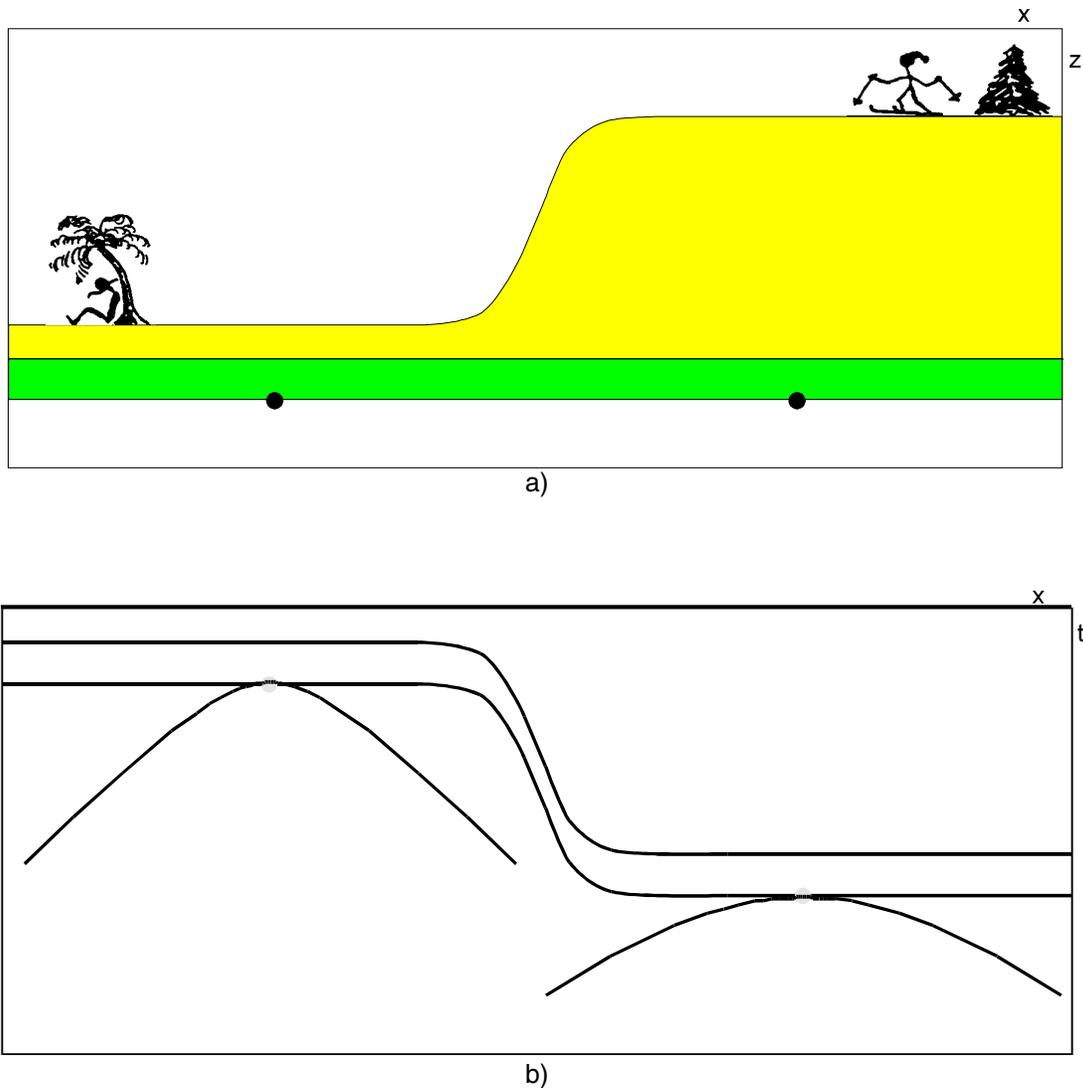
Figure 1. A geological structure (a) with a large elevation change; and (b) the resulting zero-offset time section. Time migration of this section will create large errors in the flat reflections.
