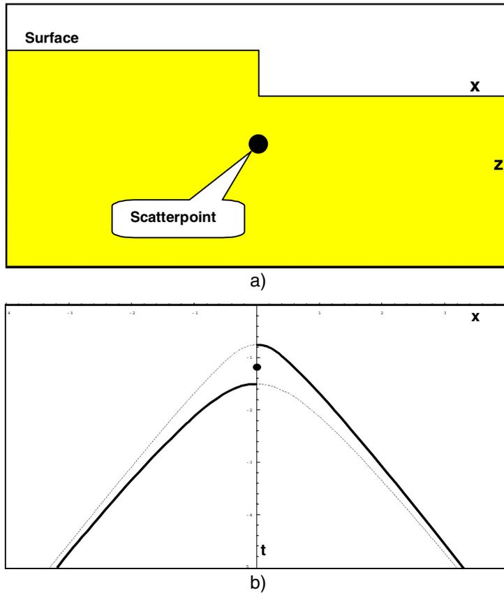
Figure 4. Scatterpoint below a step change in elevation with: a) showing the geological cross-section and; b) the resulting zero-offset time section.
