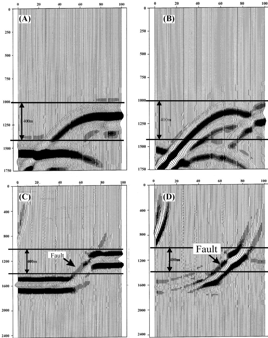
**Figure 4.** Differencing results of unmigrated and migrated data of the simple fault model: (A) unmigrated result, (B) differencing result of unmigrated section, (C) migrated result, and (D) differencing result of migrated section.
