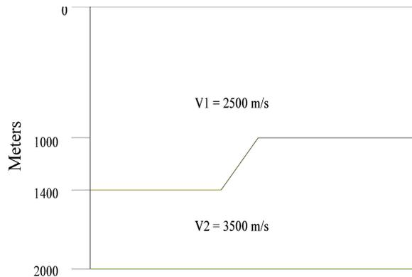
Figure 3. Simple fault model.
