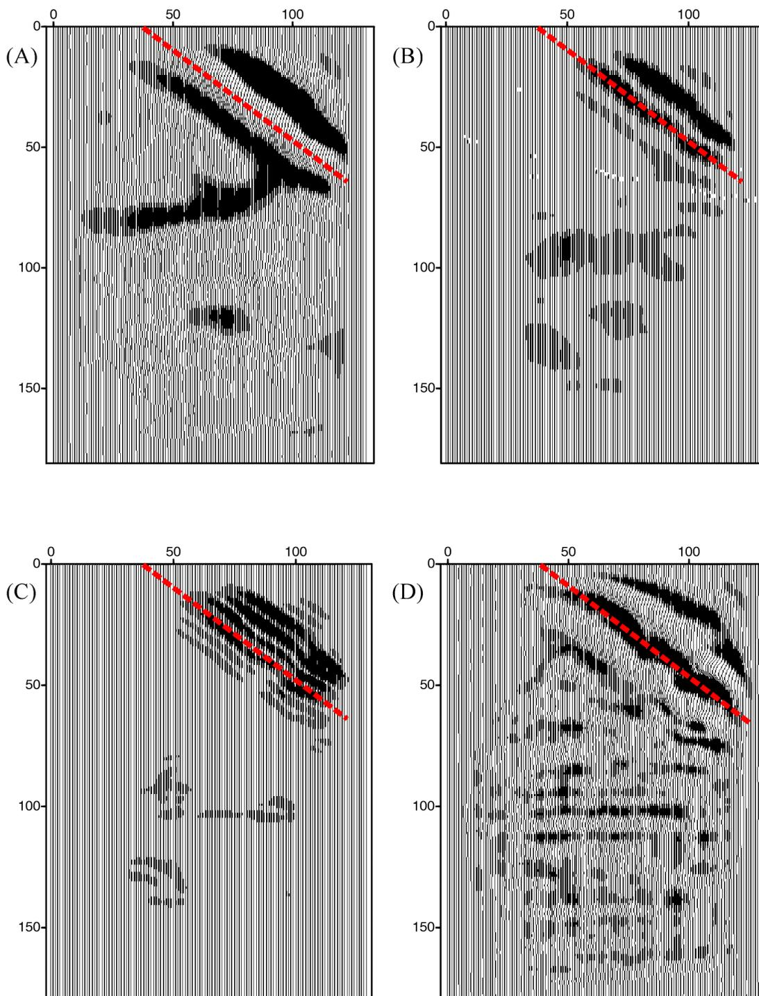
**Figure 6.** Comparison between coherence (B), differencing (C), and second derivative (D) result using input model (A) at depth slice 215 .
