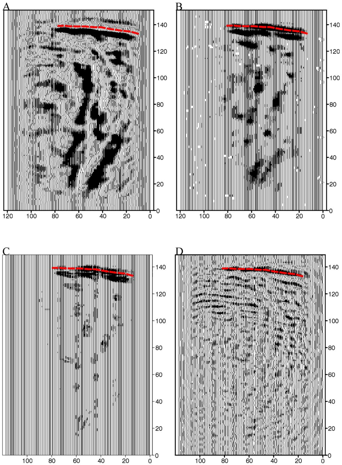
**Figure 7.** Comparison of result for depth slice 275. (A) input data, (B) coherency result, (C) differencing, and (D) second derivative result.
