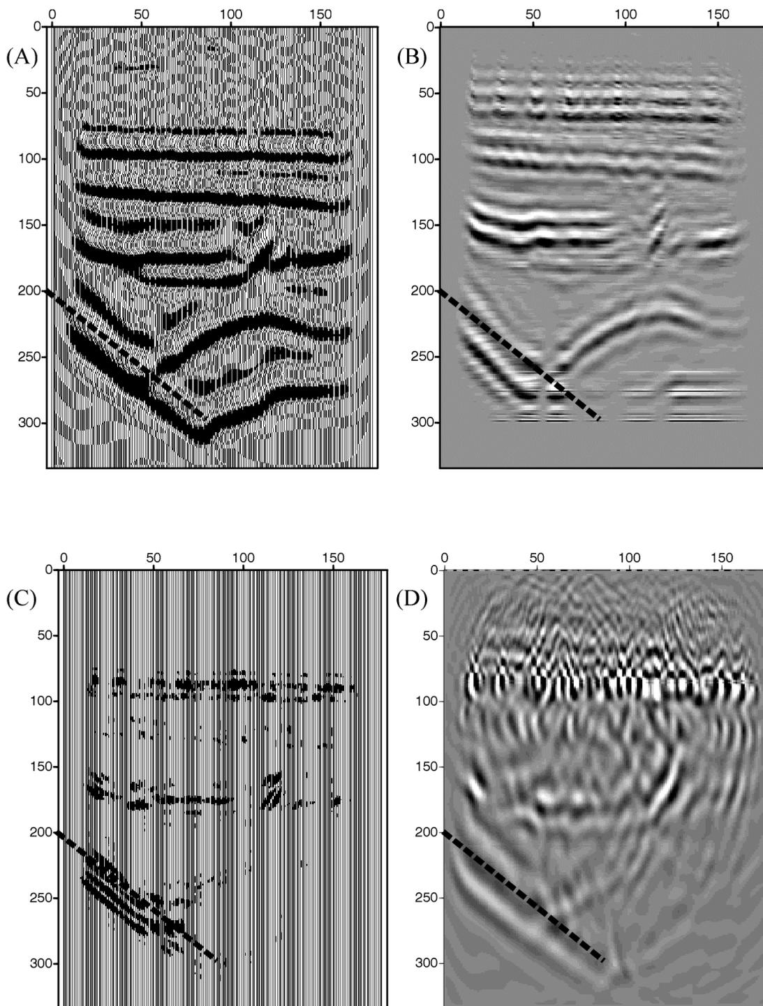
**Figure 8.** Comparison of results for in-line 60. (A) Input data, (B) coherency result, (C) differencing result, and (D) second derivative result.
