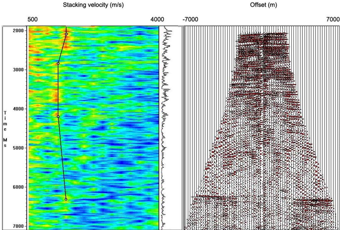
FIG. 8. Velocity analysis for the horizontal channel 4 at station 309. Note the event at just over 6 s that that builds with offset and may correspond to the event at 4 s in Figure 7.
