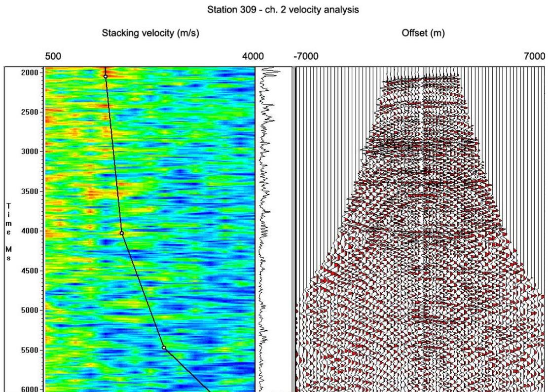
FIG. 7. Velocity analysis for the vertical channel (no. 2) at station 309. We note that the reflector at 4.0 s has a stacking velocity of about 1950 m/s.
