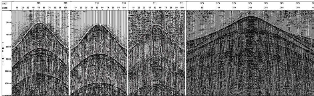
FIG 4. Common receiver gathers of the vertical component (V1), at locations 3090, 3110, 3100 and 3250.
