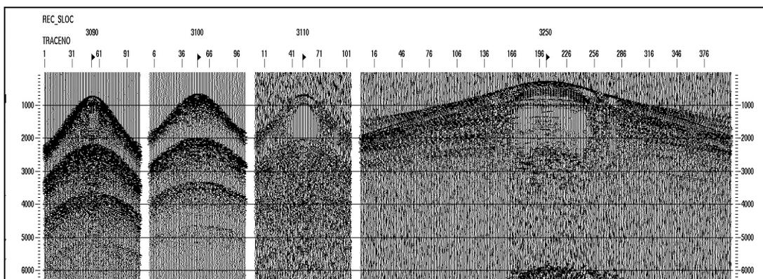
FIG. 3. Common receiver gathers for the hydrophone (pressure sensor), at locations 3090, 3110, 3100 and 3250.
