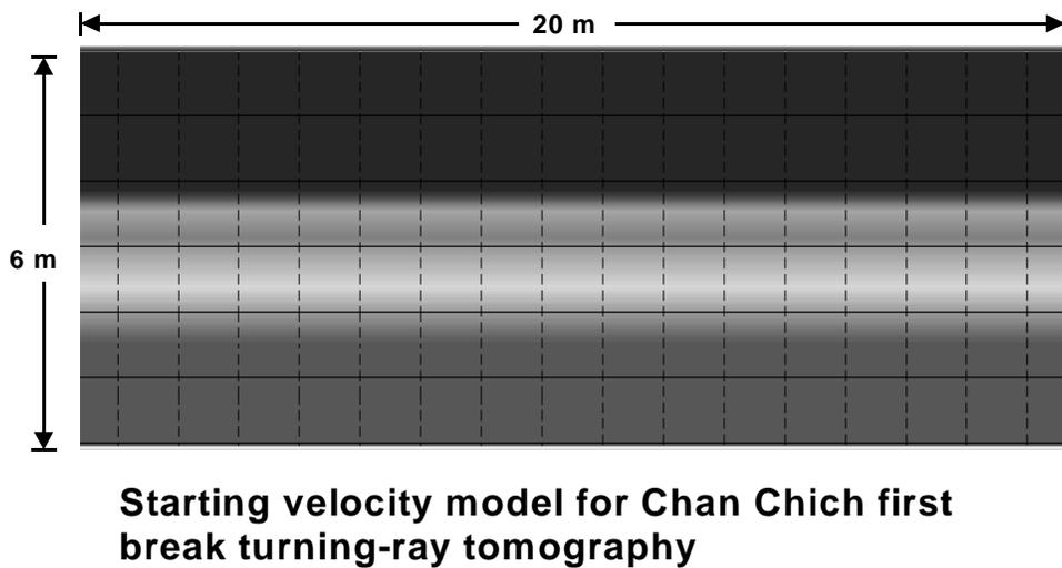
FIG. 7 Starting velocity model for Chan Chich first break turning-ray tomographic imaging. Velocities range from 500 m/s at the surface to 1200 m/s at 6 m depth, with a large gradient just above 3 m.
