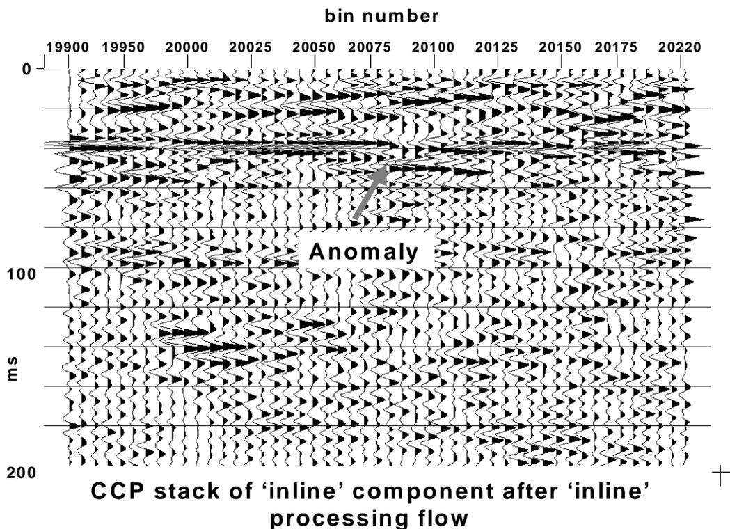
FIG. 1. Image obtained from 2000 inline horizontal component using processing tailored for 'inline' component.
