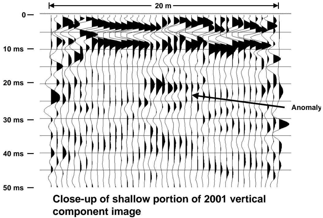
FIG. 6. Close-up image of 2001 vertical component data, showing anomaly.
