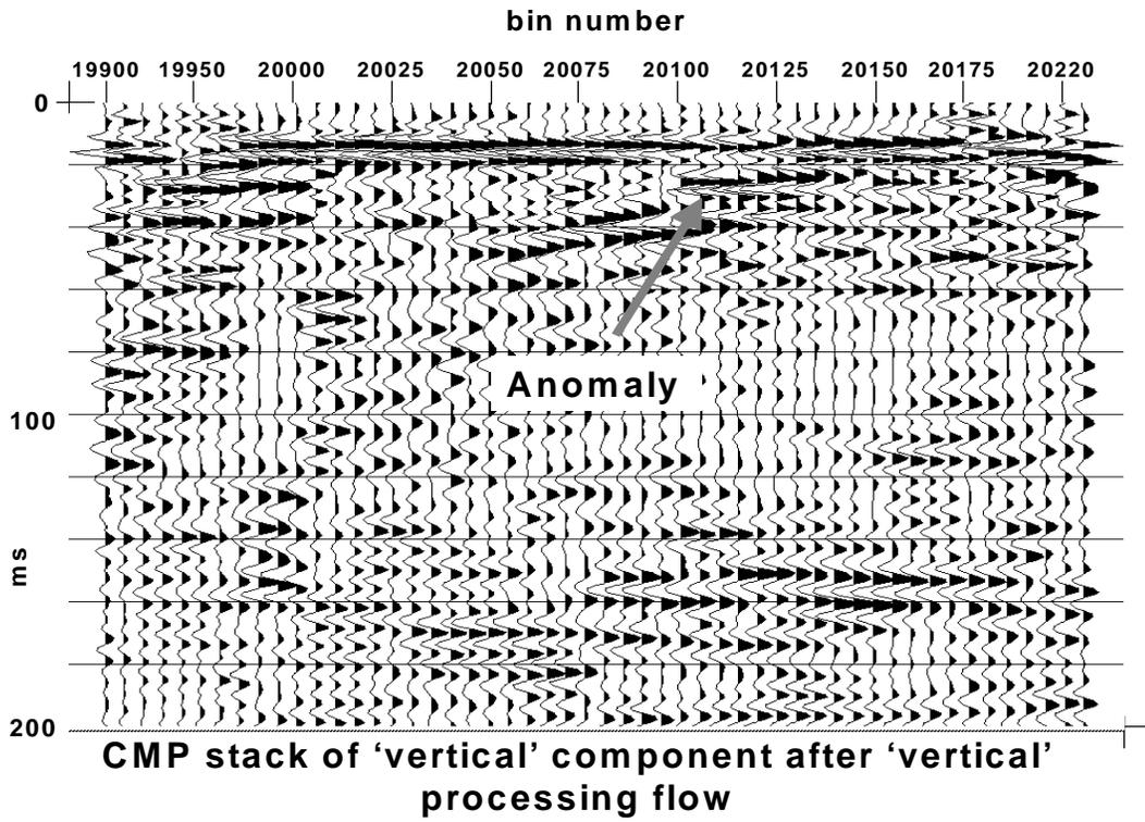
FIG. 2. Image obtained from 2000 vertical component using processing tailored for 'vertical' component.
