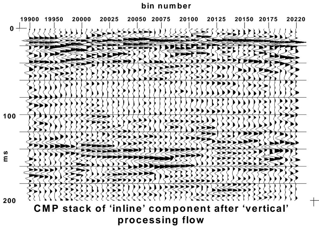
FIG. 4. Image of 2000 inline horizontal component after processing tailored for 'vertical' component.
