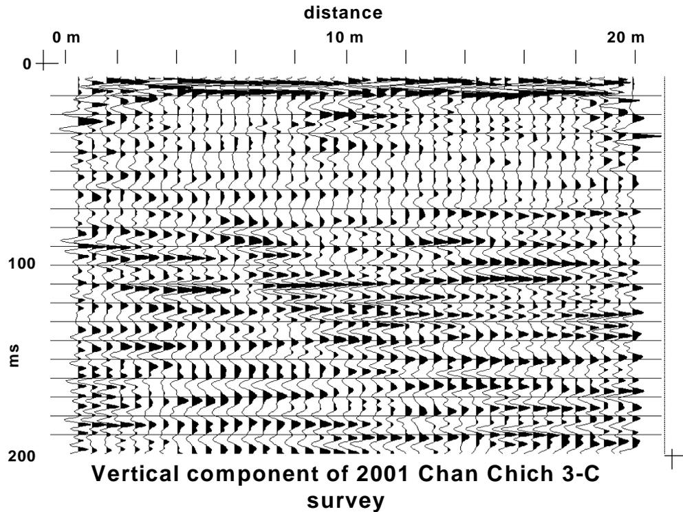
FIG. 5. Image of 2001 vertical component showing a clear anomaly near the centre.
