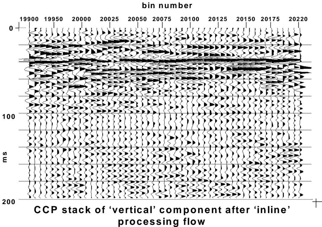
FIG. 3. Image of 2000 vertical component after processing tailored for 'inline' component.
