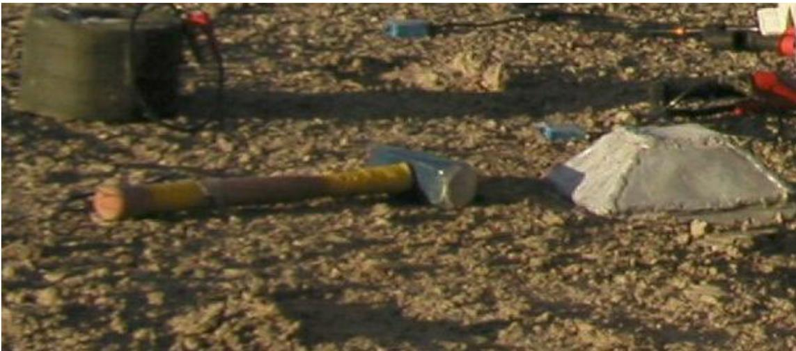
FIG. 6. Flat top pyramid for generating both P-wave and S-wave beside a three pound sledge hammer.
