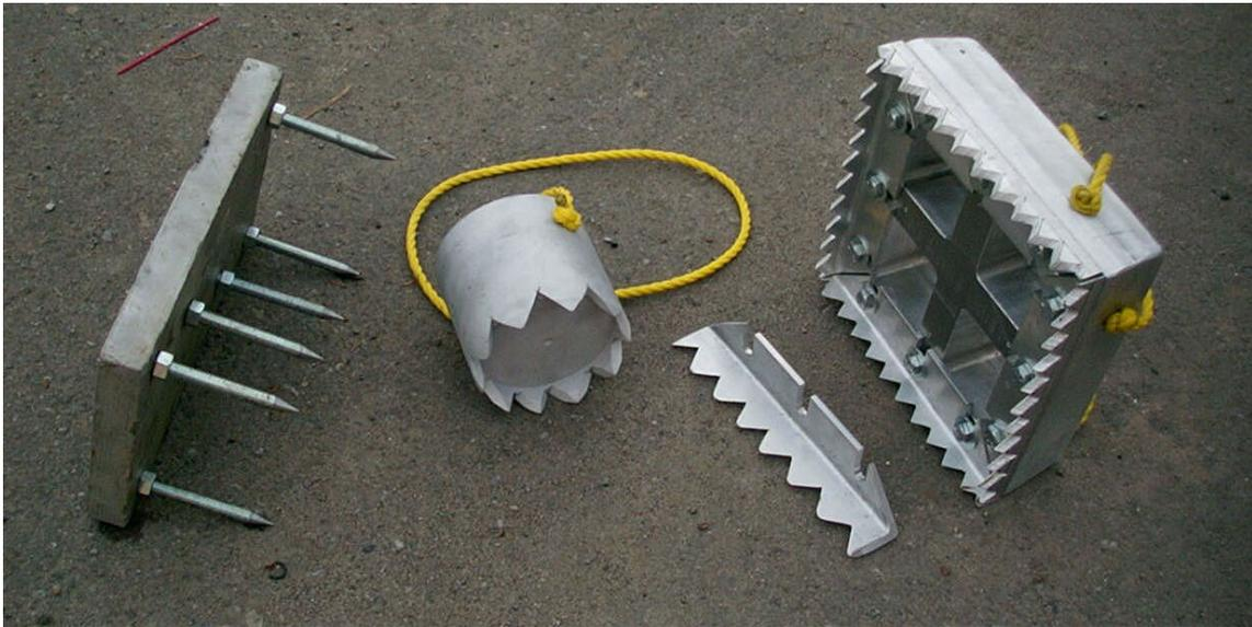
FIG. 5. Hammer seismic plates and blocks. On the left is a flat plate with geophone-like spikes and to its right is a cylinder. Both of these are vertical point sources. On the far right is the tapered block which can generate both P-wave and S-wave energy.
