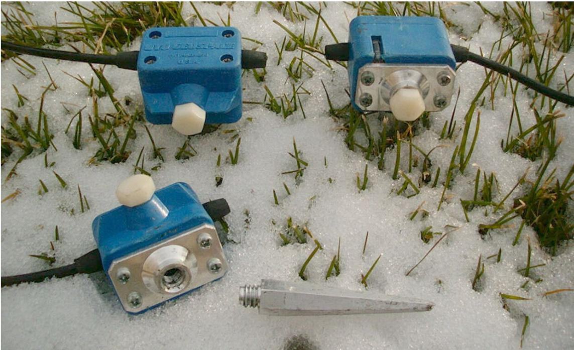
FIG. 1 Single-channel omni-directional geophones. The top left geophone is in the vertical position and the top right geophone is in the horizontal position. Note the levelling bubble on the left side of the top of the case. In the foreground is the CREWES designed adapter plate and hex-sided geophone spike. The white plastic bolts on the geophones are to keep the unused threads clean of mud or snow.
