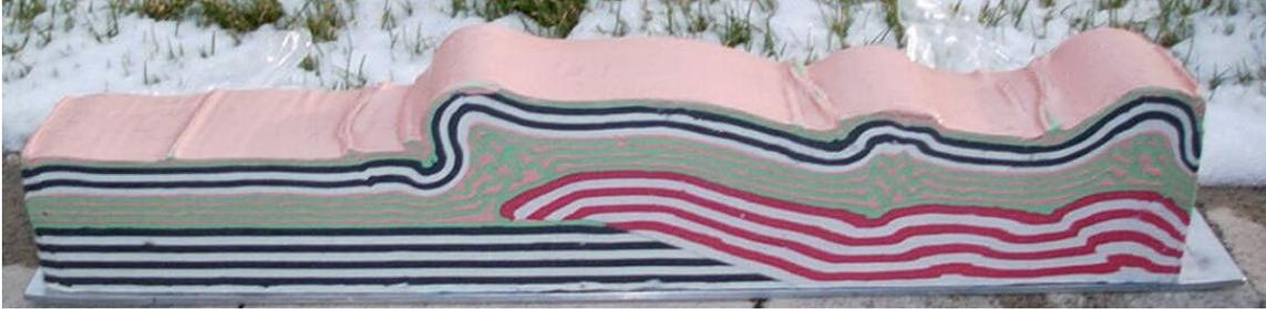
FIG. 7. A very complex fold-thrust model from the C-CORE Laboratory, Memorial University, in Saint John's, Newfoundland. The model, which is 650mm long x 100mm wide and 120mm high at the highest point, is made from silicone putty and plastercine.
