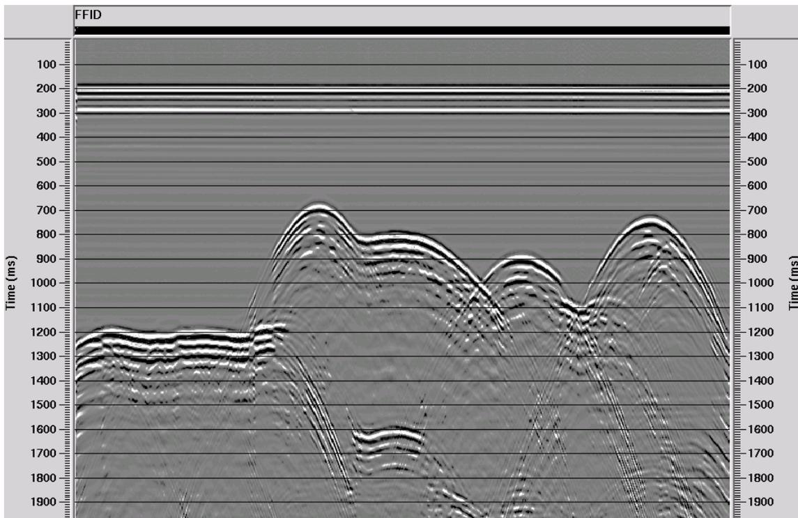
FIG. 8. Fixed offset physical modelling acoustic data from the fold-thrust model in Figure 7. Source/receiver offset 15mm, shot interval 1mm, 720 traces with 1000ms AGC.
