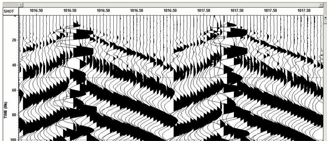
FIG.4. Two consecutive raw shot gathers using transverse oriented, horizontal geophones, with impact towards the east. Recording parameters: .5ms sample rate with traces at every 2 metres.
