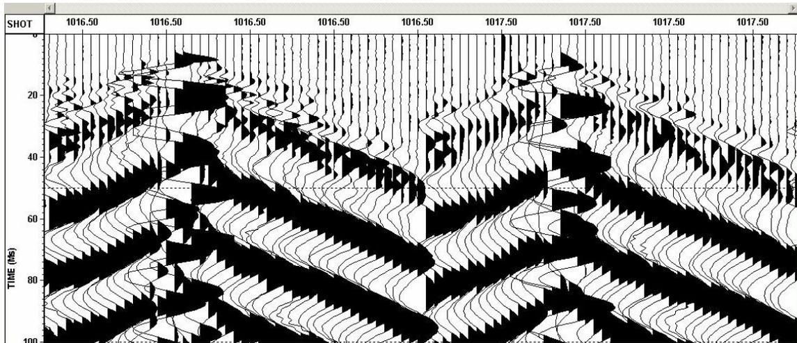
FIG.3. Two consecutive raw shot gathers using transverse oriented, horizontal geophones, with impact towards the west. The recording parameters: .5ms sample rate with traces every 2 metres.
