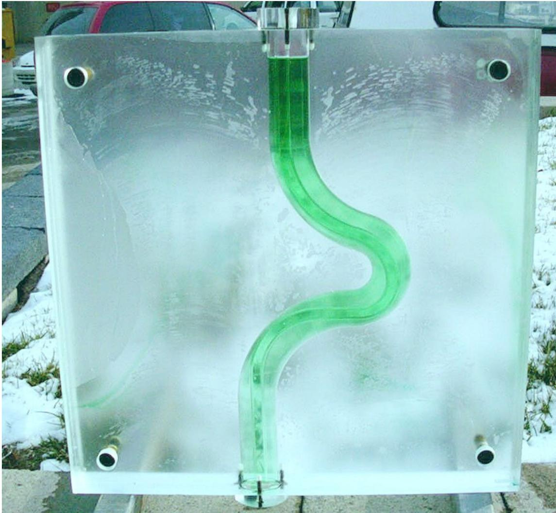
FIG.9. The reusable river channel model. Made of cast acrylic the dimensions are 600mm x 600mm x 100mm thick. The width of the channel is 45mm.
