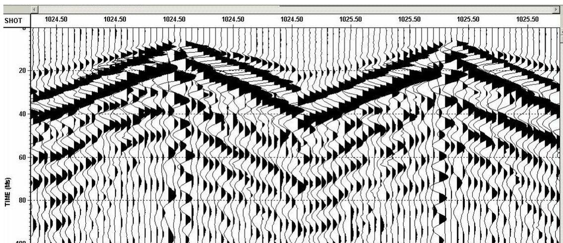
FIG.2. Two consecutive raw shot gathers using vertical oriented geophones and a vertical impact with a hammer. The recording parameters are: .05ms sample rate with traces every 2 metres, with a 200ms AGC.
