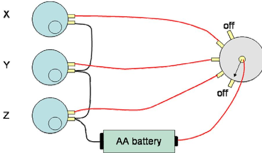
FIG. 12. Three motors are operated in sequence by connecting them to a battery via a rotating selector switch.
