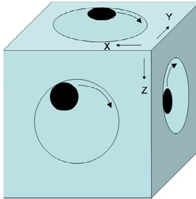
FIG. 3. A three-component vibrating cube incorporates three eccentric-mass vibrators arranged orthogonally. Each vibrator generates motion in two axes.
