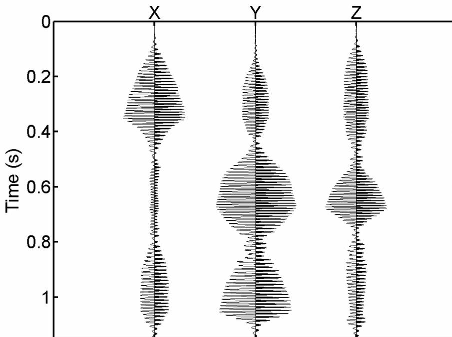
FIG. 13. Output of the prototype 3-C microvibrator recorded by a 3-C geophone. The motors were activated in sequence ( $Y=0$ ,  $X=0$ ,  $Z=0$ ) for a brief period of time.
