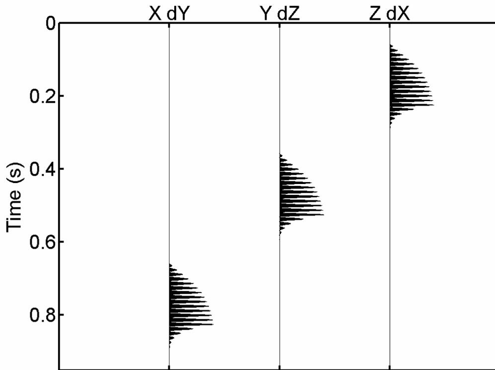
FIG. 6. The synthetic data traces from Figure 4 are processed to detect polarity reversals. Here, trace excursions are exclusively positive because there are no trace polarity reversals.
