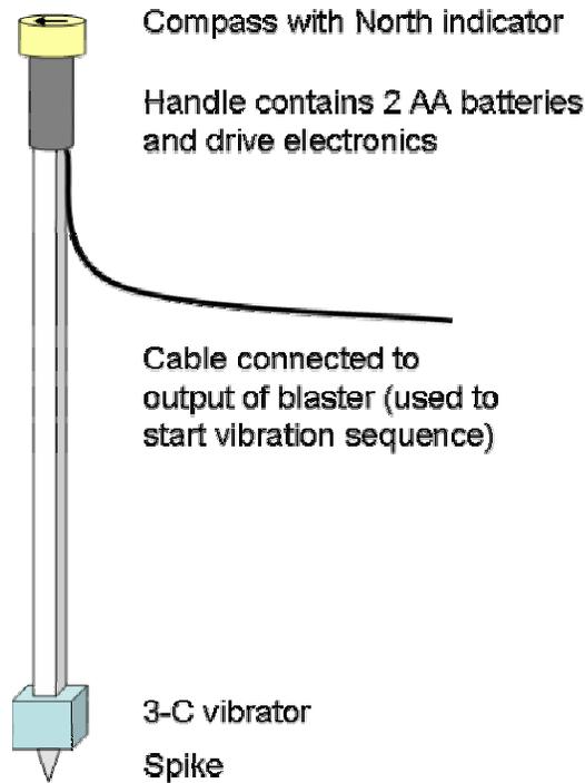
FIG. 5. A staff-mounted 3-C microvibrator shakes the ground beside a geophone. Batteries and electronics in the handle energize each disc vibrator in sequence. A spike on the bottom of the staff improves the coupling of vibratory energy to the ground.
