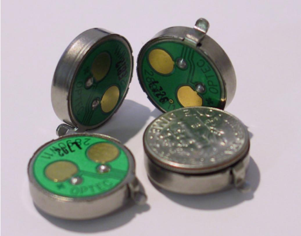
FIG. 1. Small vibrating motors (a dime is shown for scale) produce a two-component sinusoidal vibratory source. These motors are typically used in vibrating mobile telephones and pagers.
