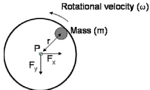
FIG. 2. An eccentric mass rotates about a point P at a distance  $r$  generating sinusoidally-varying forces  $F_x$  and  $F_y$ .
