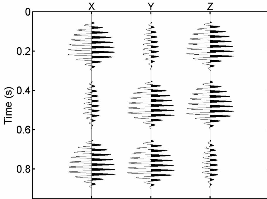
FIG. 9. Crosstalk is added to the ideal (synthetic) data generated by a 3-C microvibrator.
