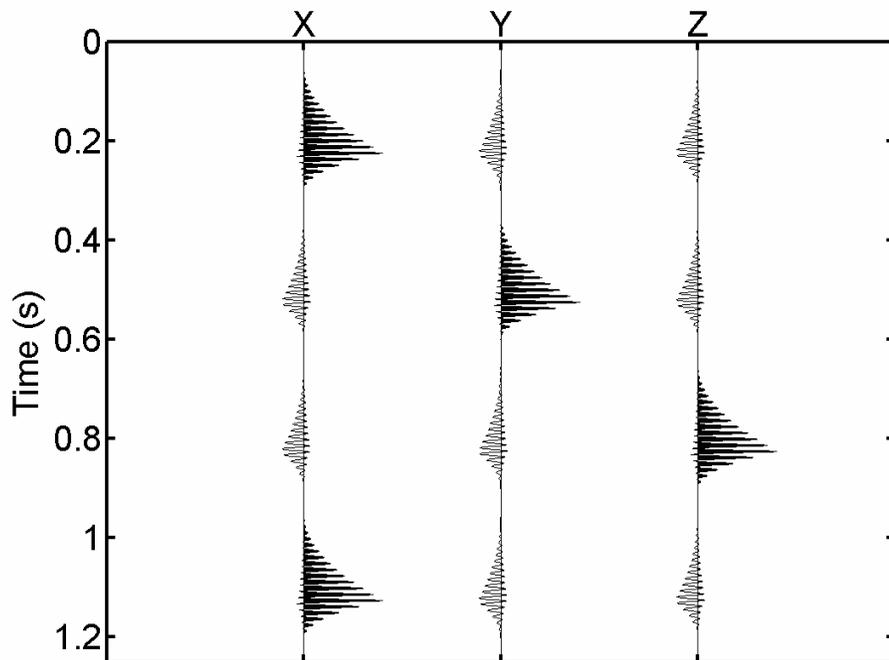
FIG. 10. Processed output of the synthetic data with 25% crosstalk shows how the crosstalk is largely rejected by the procedure.
