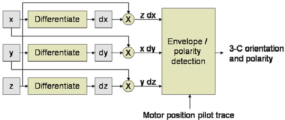
FIG. 8. Block diagram of processing flow to determine 3-C orientation and polarity.
