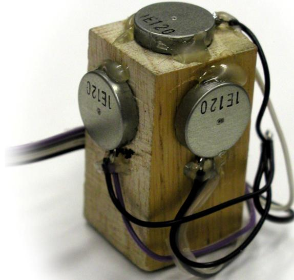
FIG. 11. Prototype 3-C microvibrator.
