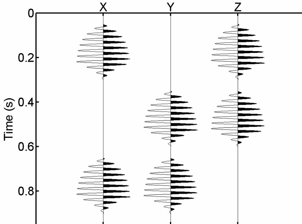
FIG. 4. Theoretical response to the switching on and off of three vibrating disc motors in sequence is shown. Here the motor on the  $Y=0$  plane is activated first, the  $X=0$  plane second, and the  $Z=0$  plane motor third. The amplitude envelope mimics the envelope observed on some test motors. In this example, the motors spin at 40 Hz (2400 RPM).
