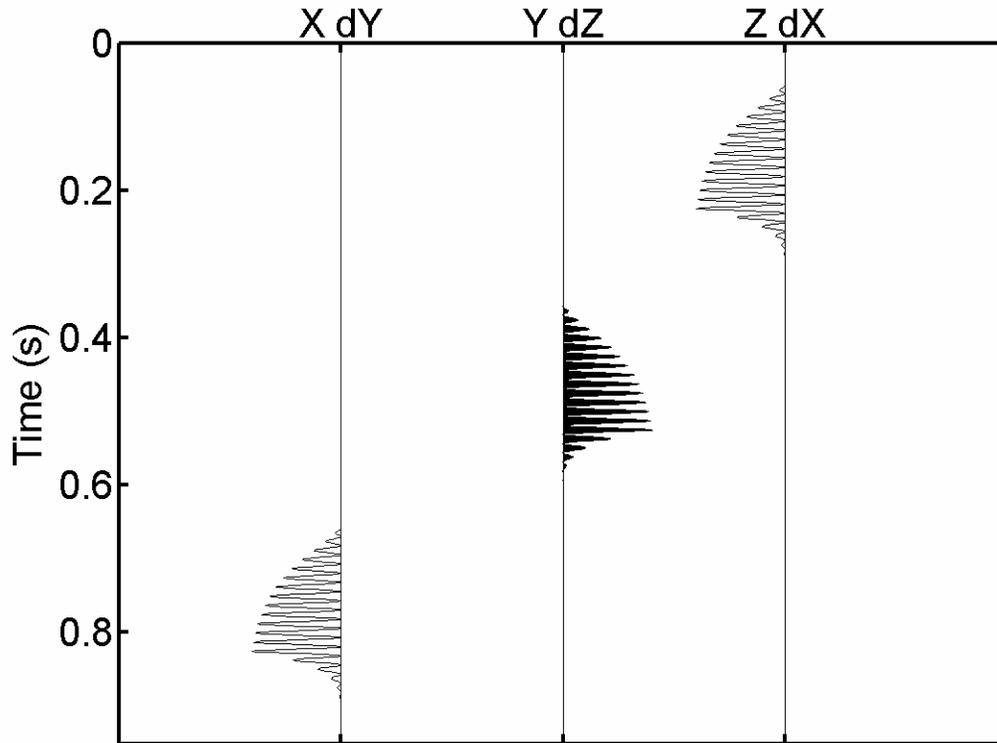
FIG. 7. If the X trace has its polarity reversed, the resultant traces are directed negative whenever the polarity-reversed trace is involved in the calculation.
