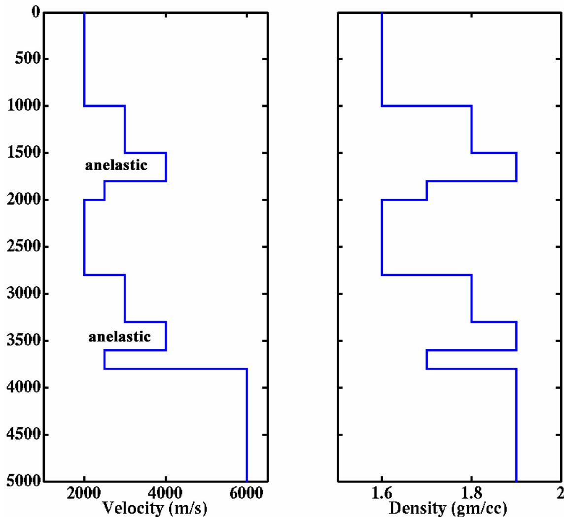
FIG. 2. Velocity and density versus depth profiles for the model considered in this report. The velocities are *reference* velocities supposedly measured at some reference frequency. In actuality they reflect the velocities that would be measured if the media were elastic. The two anelastic layers are indicated on the velocity depth plot.
