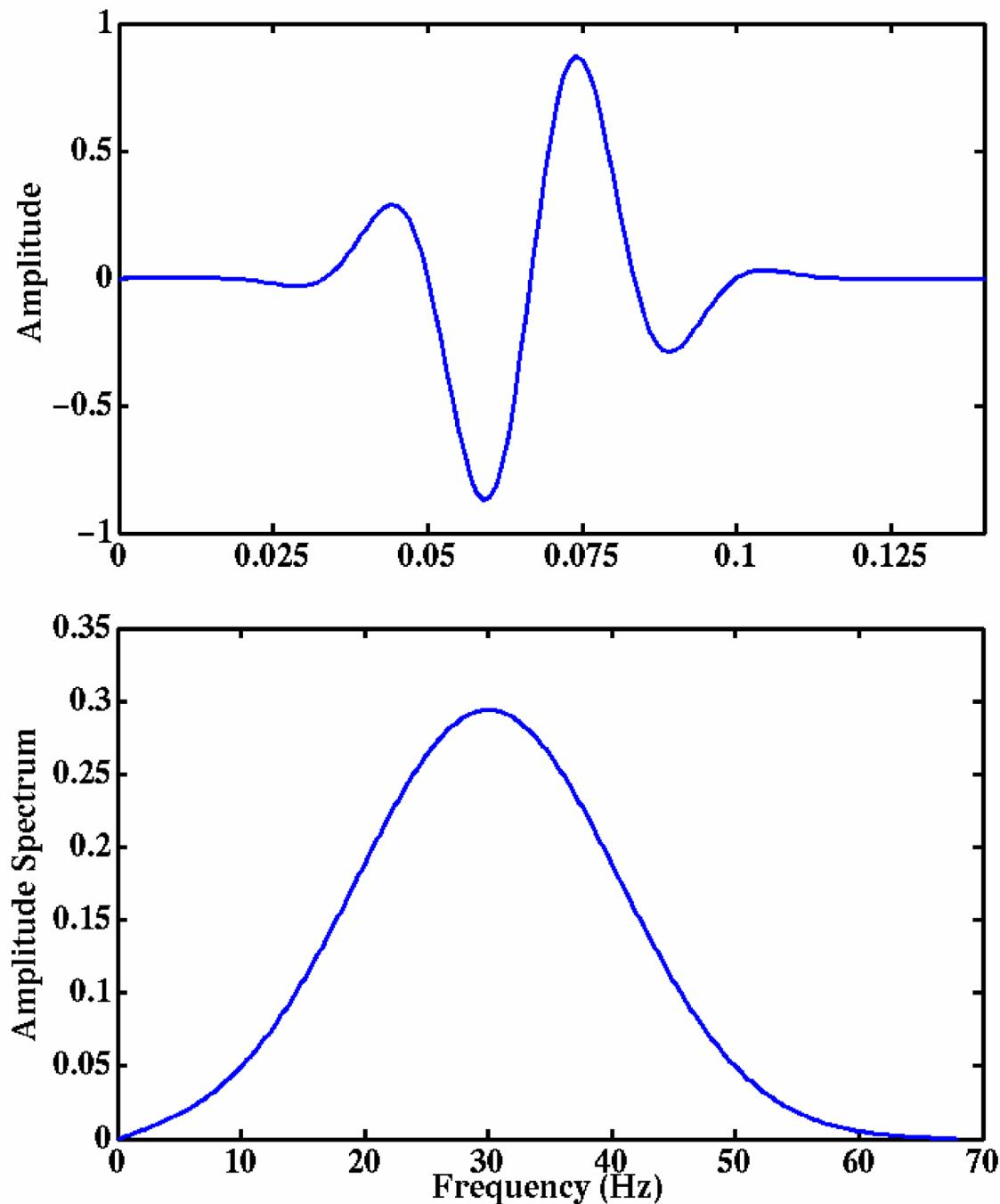
FIG. 1 The time and frequency dependence of the Gabor wavelet with a predominant frequency of 30 Hz and a damping factor of 4.
