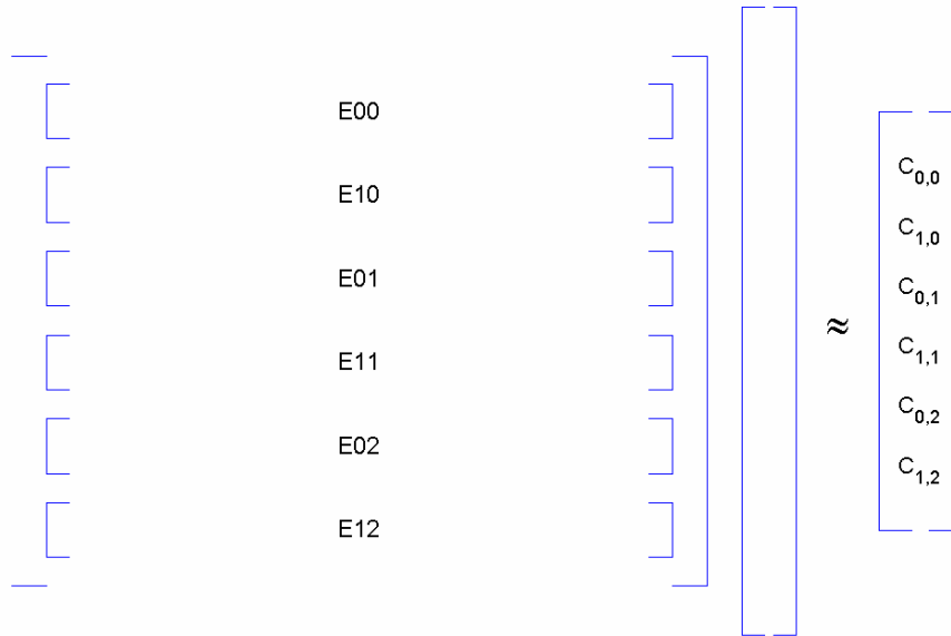
FIG. 7: The equation from Figure 6 has the elementary matrices sorted into separate rows, and output amplitudes reformed into one column. It is in the form MU \approx D , analogous to Figure 3.
