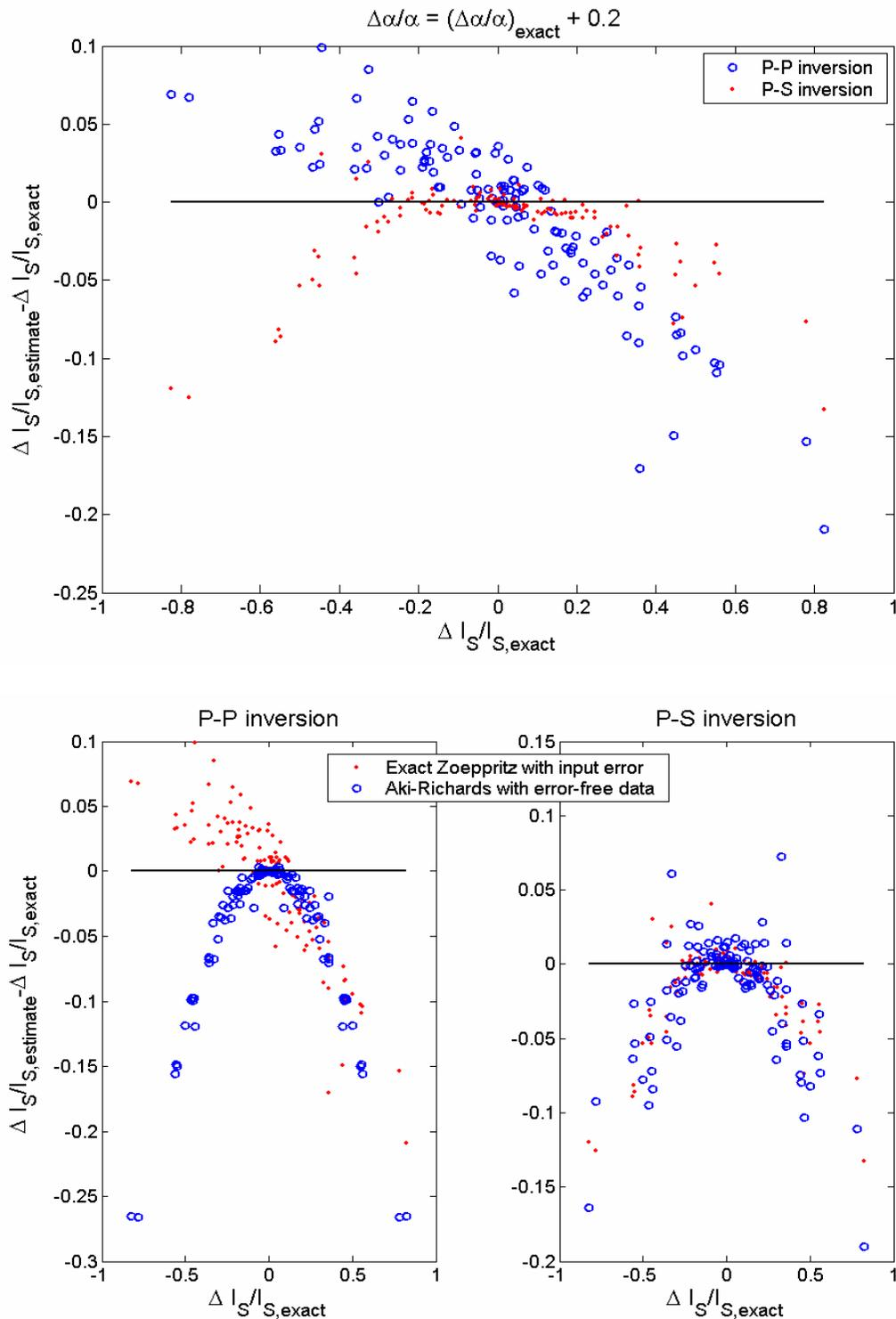
FIG. 3. The upper graph compares P-P and P-S inversions when the background value of  $\Delta\alpha/\alpha$  is overestimated by 0.2. The P-P inversion results vary linearly with  $\Delta|S'/S$ , but with significant scatter. The P-S inversion results vary quadratically overall, but with a similar magnitude. The lower plots compare this same data to the corresponding Aki-Richards inversions of error-free data.
