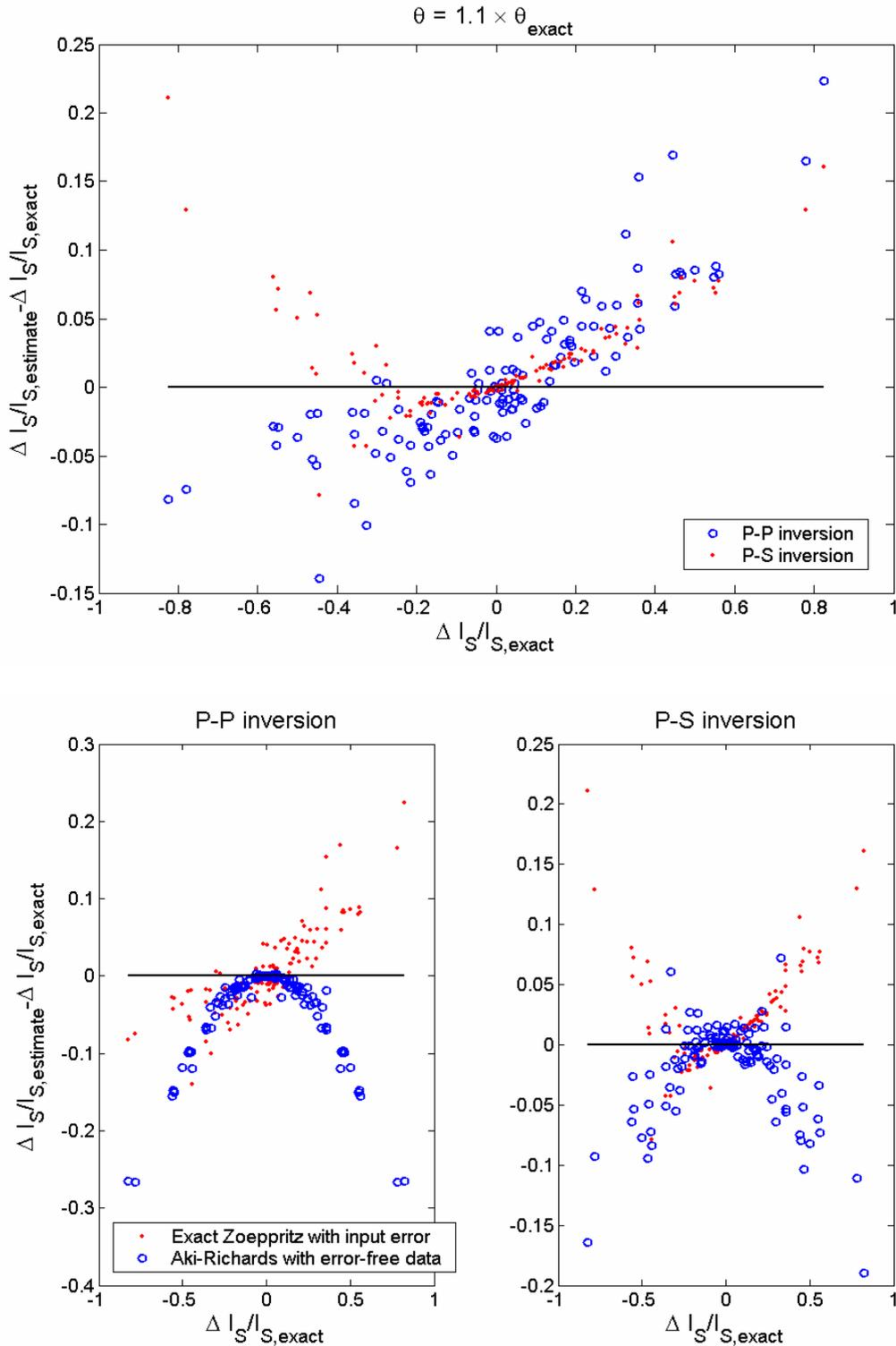
FIG. 7. The upper graph compares P-P and P-S inversions when the angles of incidence are linearly scaled up by 10%. The resulting contrast errors are correlated with  $\Delta I_S/I_S$  but possess significant scatter. The lower plots compare this same data to the corresponding Aki-Richards inversions of error-free data.
