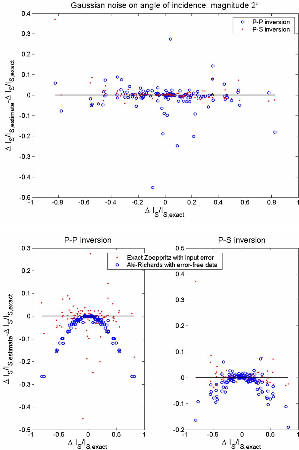
FIG. 6. The upper graph compares P-P and P-S inversions when Gaussian noise is added to the angle of incidence with an order of magnitude of 2°. The P-S errors are generally smaller for  $\Delta l_S/l_S < 0.4$ , but both methods are similar above that. The lower plots compare this same data to the corresponding Aki-Richards inversions of error-free data.
