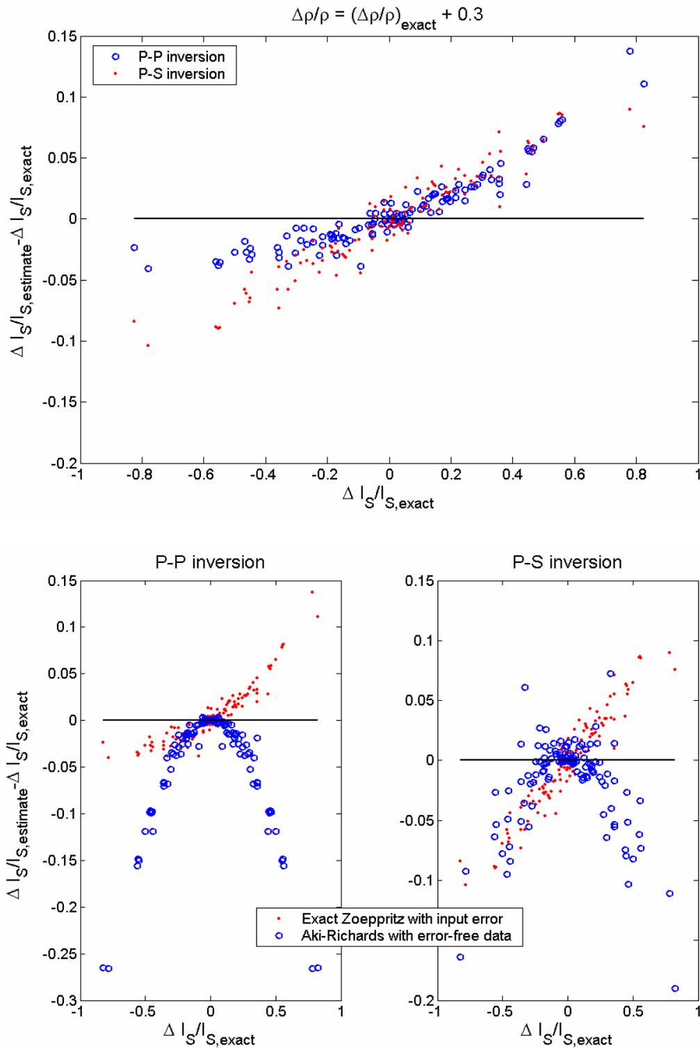
FIG. 5. The upper graph compares P-P and P-S inversions when the background value of  $\Delta\rho/\rho$  is overestimated by 0.3. In this case both methods yield very similar errors, linearly correlated with  $\Delta l_S/l_S$ . The lower plots compare this same data to the corresponding Aki-Richards inversions of error-free data.
