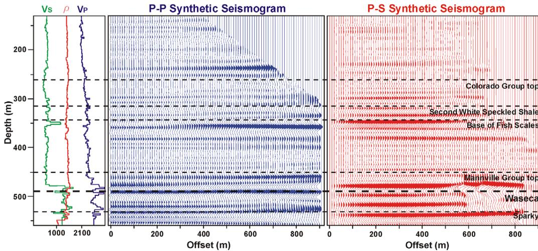
FIG. 4. Well 1A15-6 P-P and P-S synthetic seismograms used in calculating the RMS amplitude values over a range of offsets.
