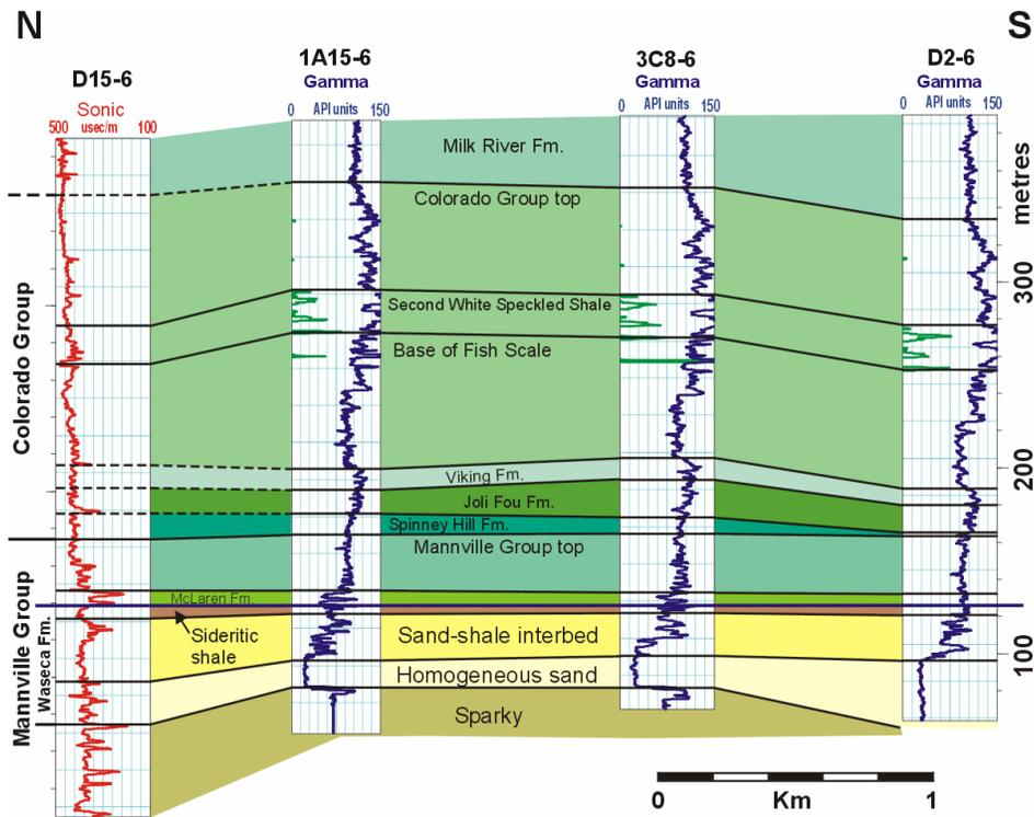
FIG. 2. Well-log cross-section illustrating the Lower Cretaceous stratigraphy (flattened at the top of the Waseca Fm). There is a channel sequence previously interpreted within the Waseca Fm (Van Hulst, 1984) and refined by the authors.
