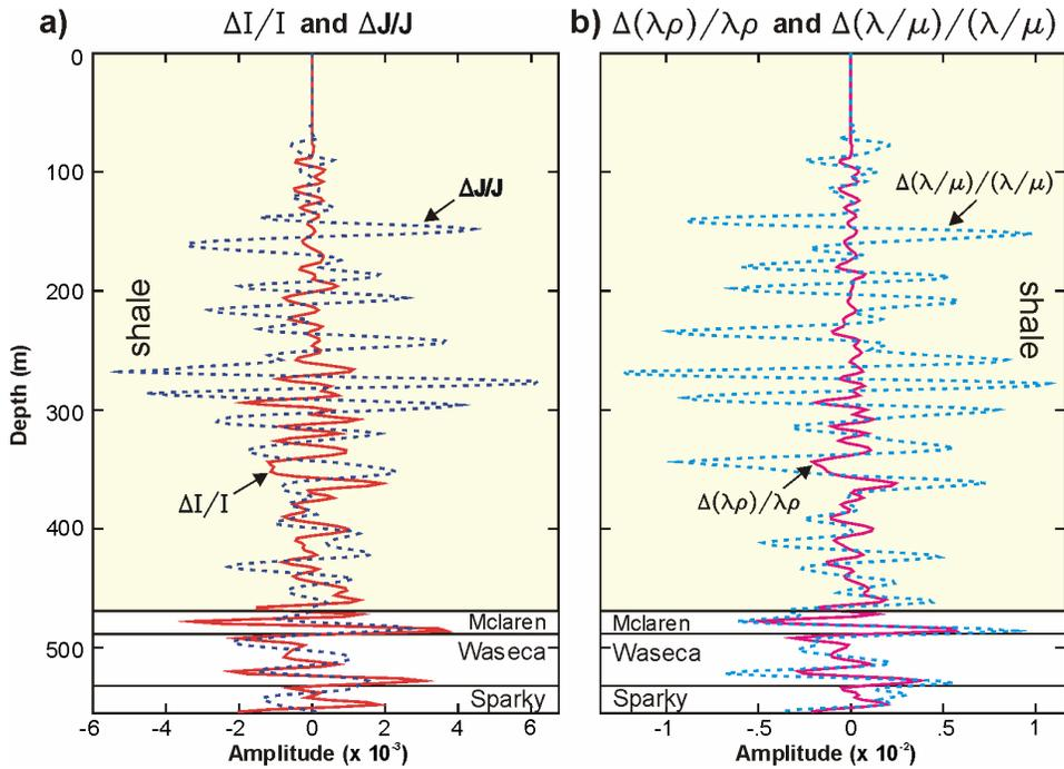
FIG. 9. Average amplitude values of a)  $\Delta I/I$  and  $\Delta J/J$  and b)  $\Delta(\lambda\rho)/\lambda\rho$  and  $\Delta(\lambda/\mu)/(\lambda/\mu)$  from traces around well 1A15-6.
