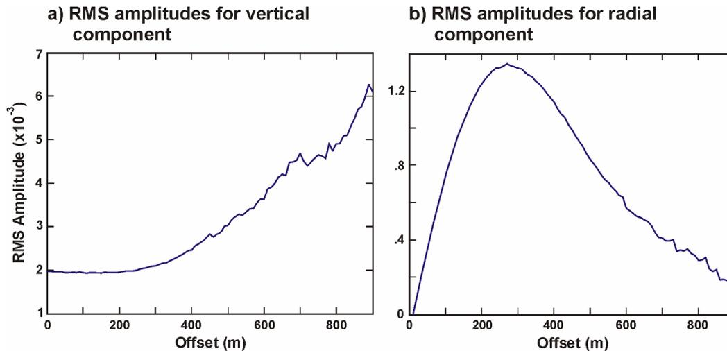
FIG. 5. RMS amplitudes versus offsets for (a) vertical and (b) radial components.
