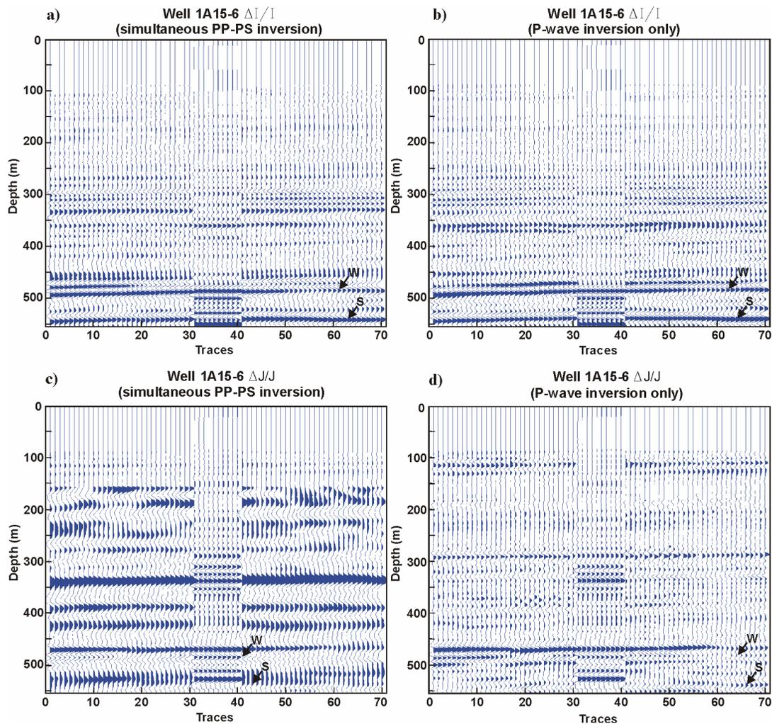
FIG. 7. Comparison of  $\Delta I/I$  and  $\Delta J/J$  from A15-6 well-log computation with  $\Delta I/I$  and  $\Delta J/J$  from a) and c), the simultaneous inversion, and b) and d), P-P standalone inversion. W-Waseca top; S-Sparky top.
