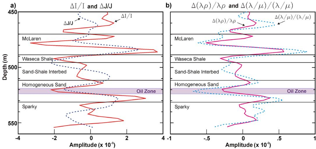
FIG. 10. Expanded attribute curves of  $\Delta I/I$ ,  $\Delta J/J$ ,  $\Delta(\lambda\rho)/\lambda\rho$ , and  $\Delta(\lambda/\mu)/(\lambda/\mu)$  around well 1A15-6.
