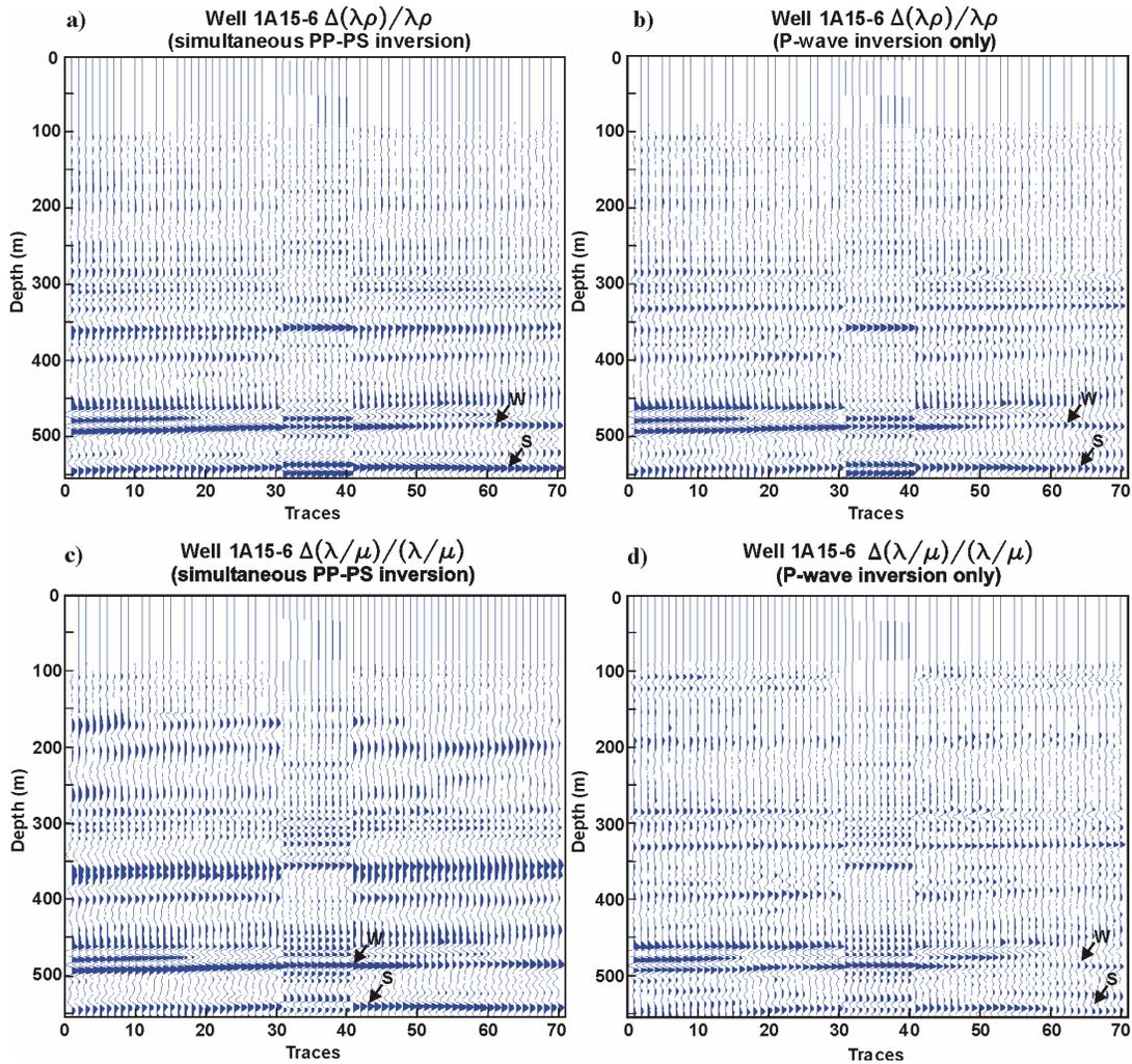
FIG. 8. Comparison of  $\Delta(\lambda\rho)/\lambda\rho$  and  $\Delta(\lambda/\mu)/(\lambda/\mu)$  from A15-6 well-log computation with  $\Delta(\lambda\rho)/\lambda\rho$  and  $\Delta(\lambda/\mu)/(\lambda/\mu)$  from a) and c), the simultaneous inversion, and b) and d), P-P standalone inversion. W-Waseca top; S-Sparky top.
