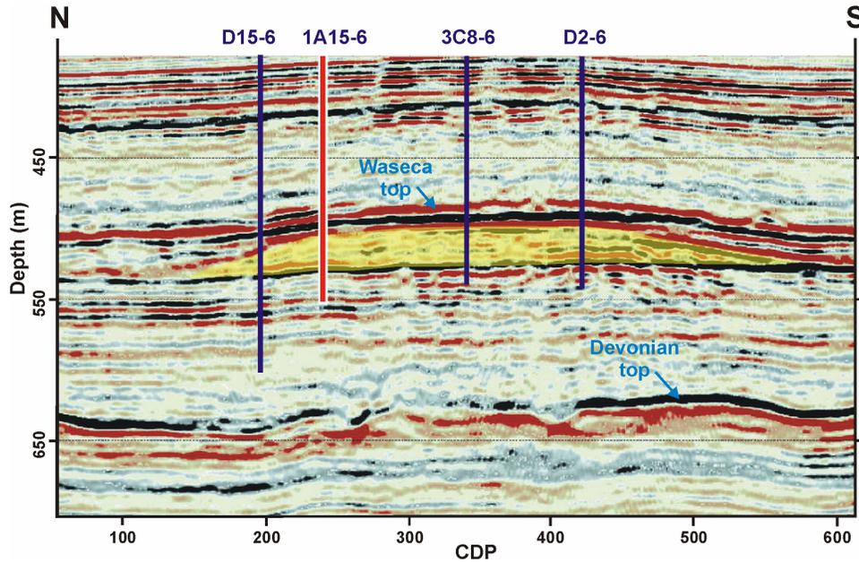
FIG. 6. The Waseca Fm reservoir (in yellow) and wells, including the dipole well 1A15-6 used in this paper.
