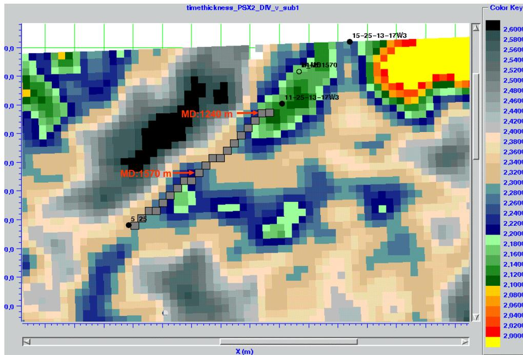
FIG. 9. Zoomed  $V_p/V_s$  map with the projection of the horizontal well (grey squares). The top red arrow indicates the starting point of the horizontal borehole.
