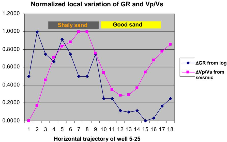
FIG. 10. Plot showing the normalized variation of MWD GR and seismic  $V_p/V_s$  along the trajectory of the horizontal section of well 5-25.
