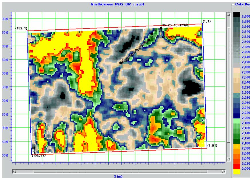
FIG. 8.  $V_p/V_s$  map between the IHACM and the RushLake horizon. The yellow and green colours are interpreted as sands while black and grey are interpreted as shale or shaly sands.
