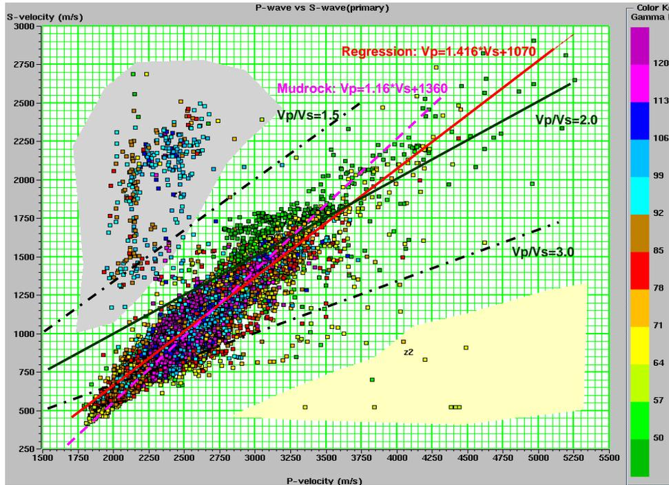
FIG. 1. Crossplot of measured  $V_p$  and  $V_s$  logs from 4 regional wells.
