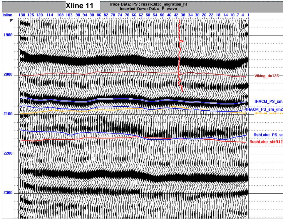
FIG. 6. Horizon pickings on the PS seismic section. Blue lines are picked PS horizons while red lines are same PP horizons shown in PS time, using the constant  $V_p/V_s=2.35$ .
