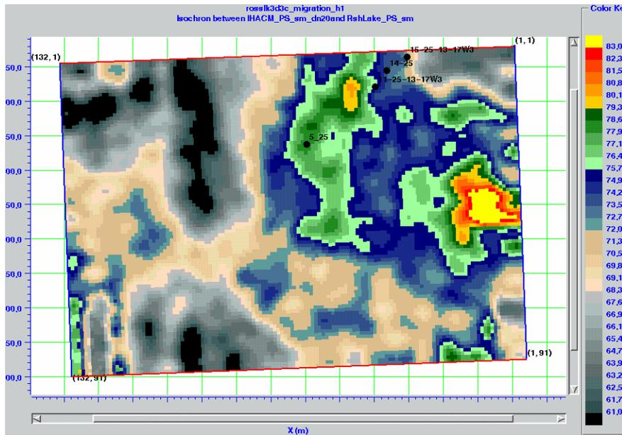
FIG. 7. PS time-thickness map for the IHACM and the RushLake horizon.
