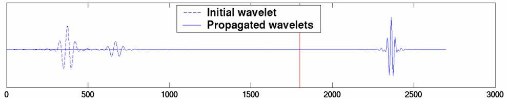
FIG. 3. Propagation with the right side of the model corrected at each step with a 5 point spatial operator.
