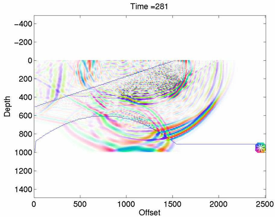
FIG. 8. Corrected model. The corrections may be seen to have concentrated the energy, although some events still show dispersion.
