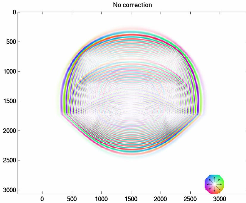
FIG. 5. Uncorrected two dimensional model. The source is centered at the (x,z) coordinates (1500,1500), just above the velocity contrast.
