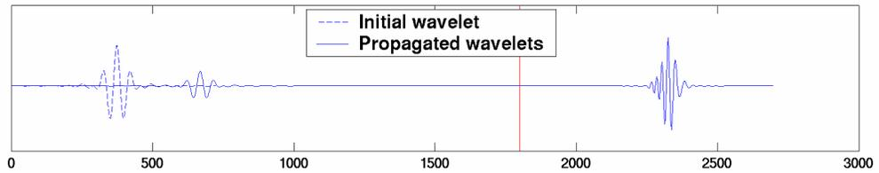
FIG. 2. Uncorrected wavelet propagation. Right side of model has half the velocity of the left side.
