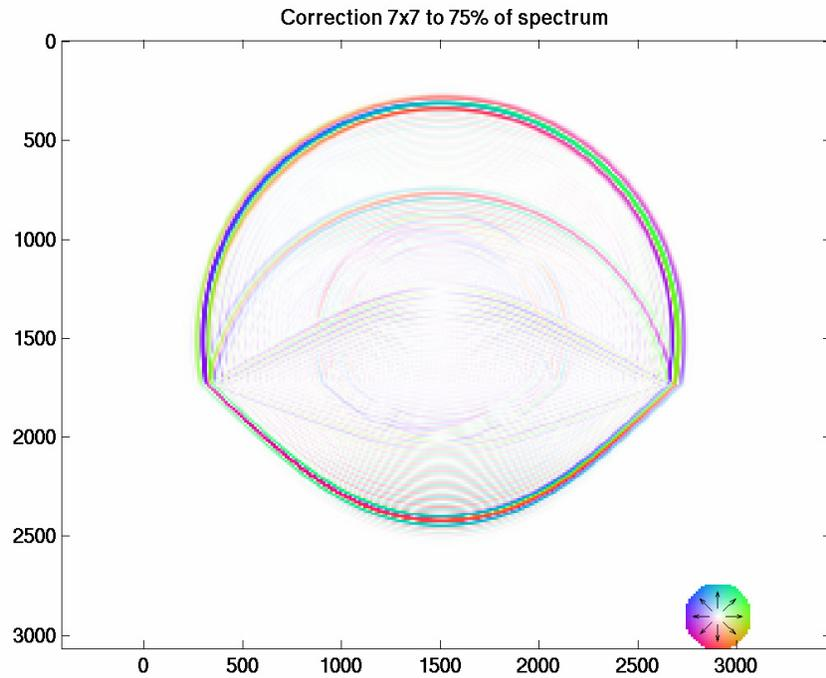
FIG. 6. Corrected model. Reflected P and S, and transmitted P and faint transmitted S waves can be seen.
