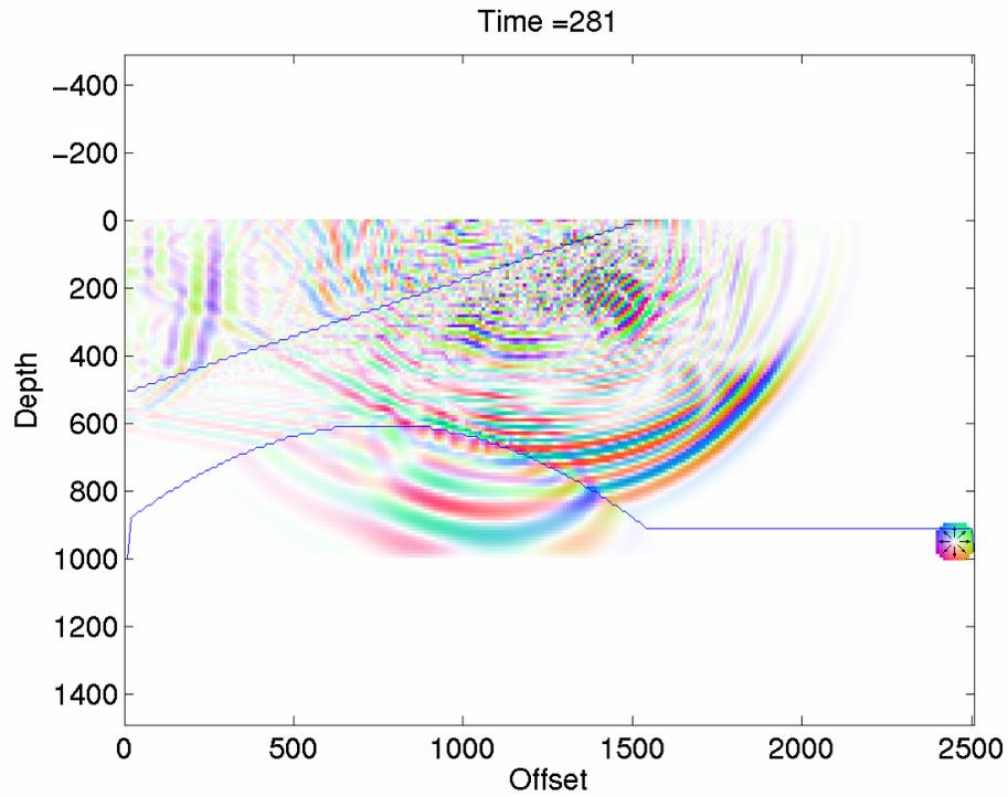
FIG. 7. Uncorrected high velocity wedge model. The source is in the centre of the model, just above the wedge boundary and below the surface.
