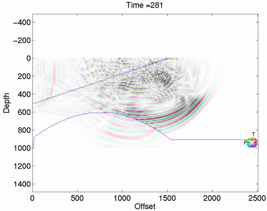
FIG. 9. Uncorrected model in the interpreted P/T (pressure/torque) format. There is obvious dispersion of both P and S waves.
