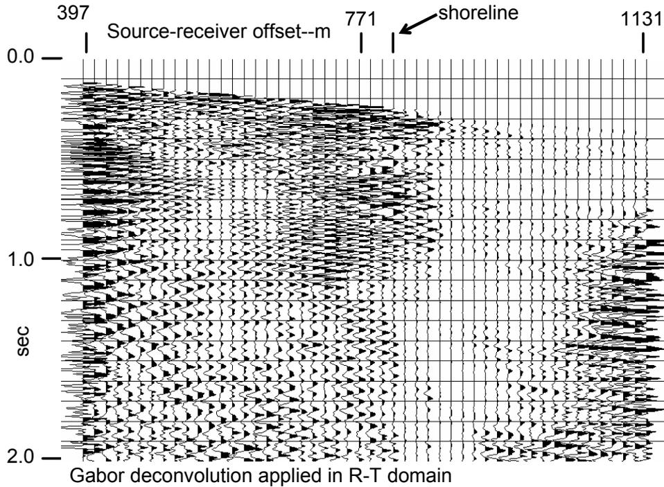
FIG. 14. Instead of spectral clipping, Gabor deconvolution has been applied in the R-T domain to attempt to reduce monochromatic spectral spikes by whitening. This result is not as good as that shown in Figure 13.
