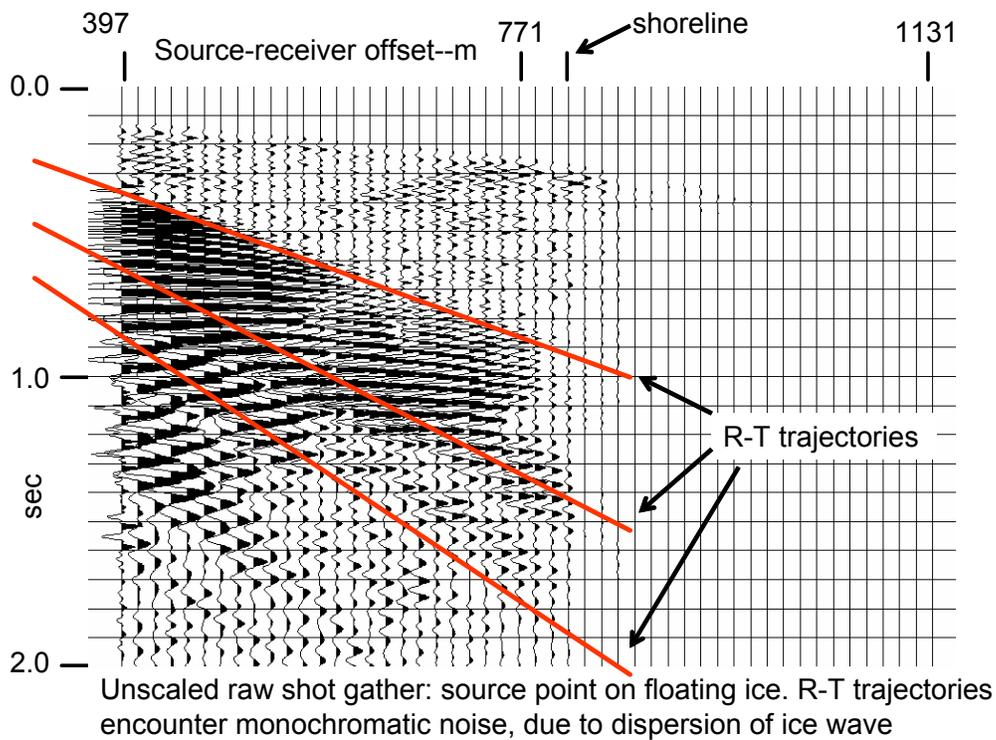
FIG. 4. Illustration showing why the radial trace (R-T) domain is an attractive one in which to attack the ice flexural wave. R-T trajectories sample the noise along paths of constant frequency, due to dispersion.
