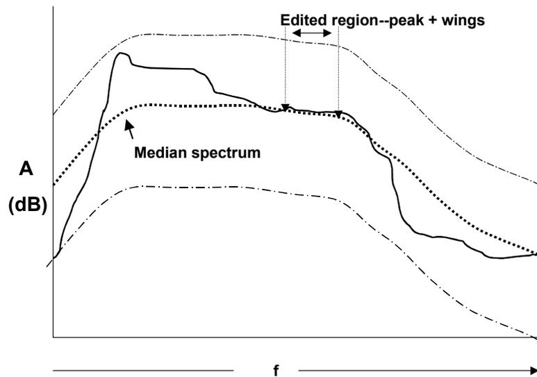
FIG. 9. The result of applying spectral clipping...the raw amplitudes are untouched, except for those frequencies which fell outside the thresholds. Phase is completely unaltered.
