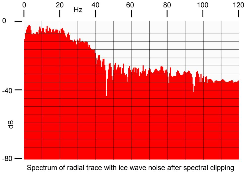
FIG. 11. Spectral clipping applied to the spectrum of Figure 6. There are now no spikes, but local spectral detail remains.
