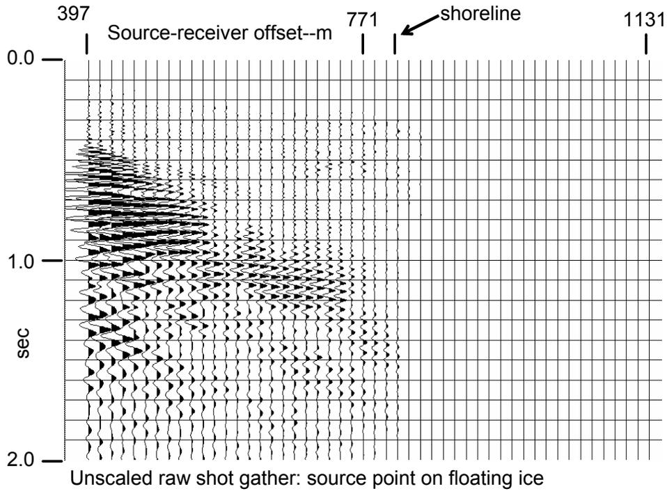
FIG. 1. Typical ice flexural noise generated by a surface source positioned on floating ice. The strength of the noise is evident, since no legitimate reflection energy can be seen on this unscaled shot gather.
