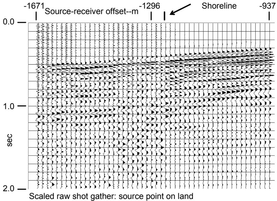
FIG. 3. Shot gather for shot positioned off the shoreward end of the receiver line. Legitimate seismic events can be seen on all stations, including those on the floating ice.
