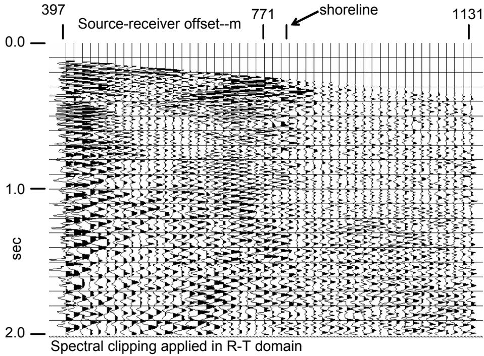
FIG. 13 Shot gather after spectral clipping in the R-T domain. The ice wave, though still present, is greatly diminished compared to Figure 4.
