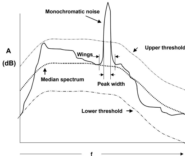
FIG. 8. Schematic illustrating the principle behind the “spectral clipping” algorithm. First, a running median of the amplitude spectrum is computed. Next, “threshold” curves are placed parallel (in dB space) above and below the median. Then, any frequencies for which the raw input amplitudes fall above or below the threshold curves are flagged, as are a few adjacent “wing” values. Finally, amplitudes for the flagged frequencies are set to their corresponding median values.
