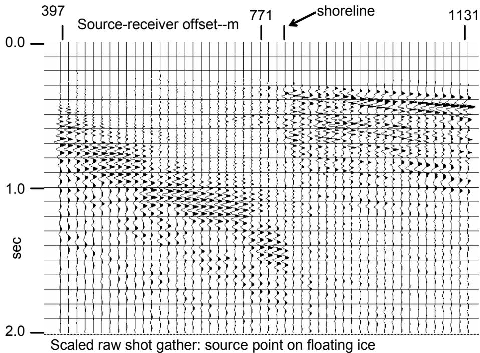
FIG. 2. Shot gather of Figure 1 after normalizing the traces. Legitimate seismic events can now be seen on those stations positioned on solid land. Stations positioned on floating ice are still dominated by the flexural noise.
