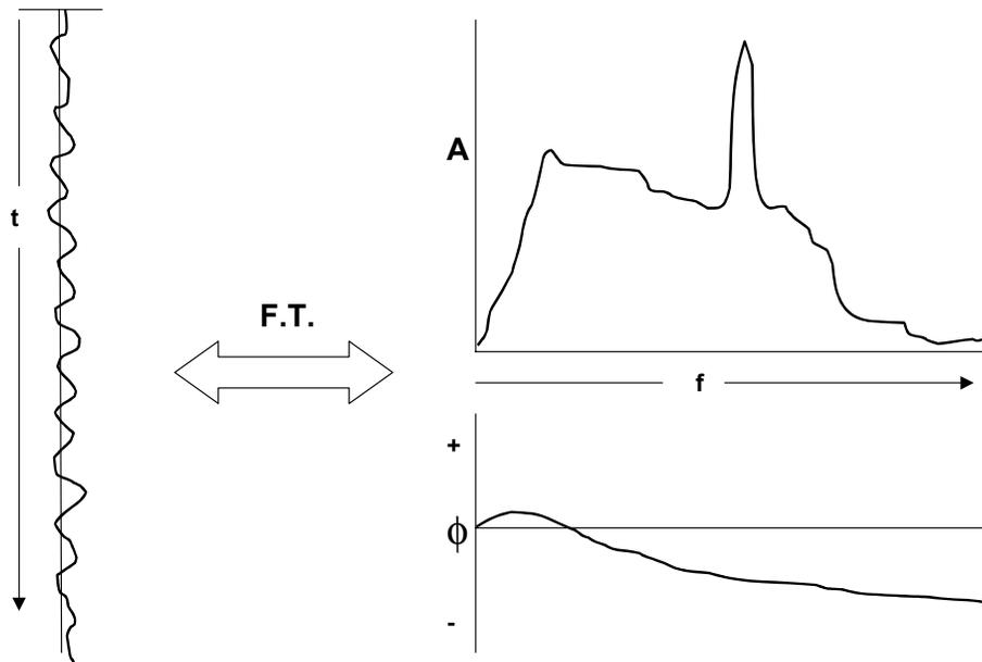
FIG. 7. Schematic showing the relation between a seismic trace contaminated with a strong monochromatic noise (left) and its amplitude and phase via the Fourier Transform.
