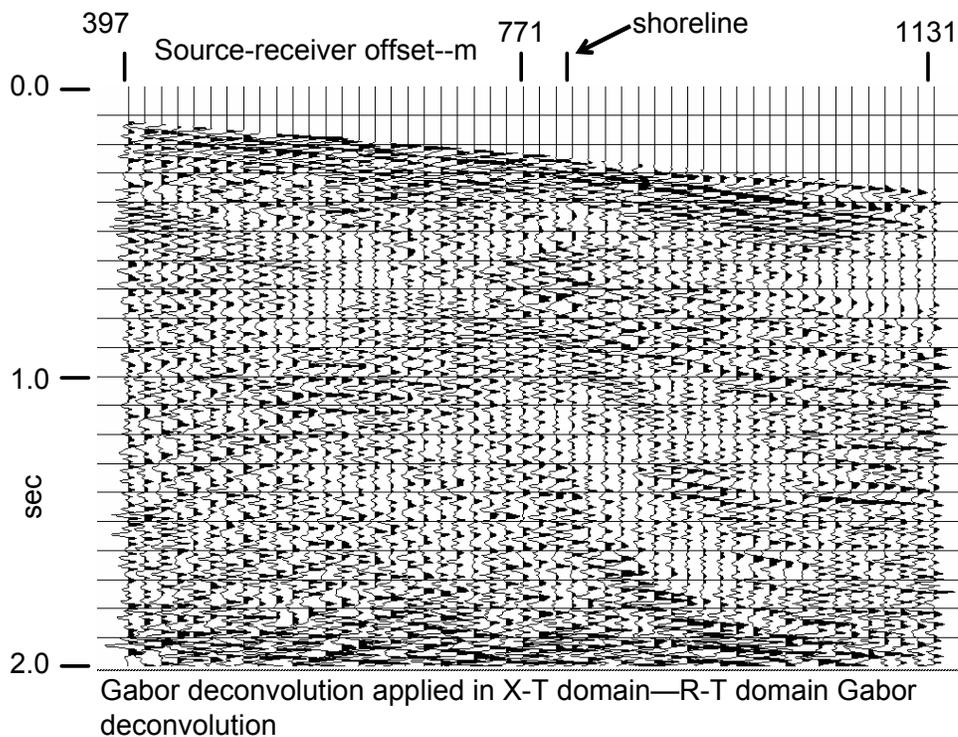
FIG. 16. Gabor deconvolution has been applied in both the R-T and X-T domains. This is the best result yet.
