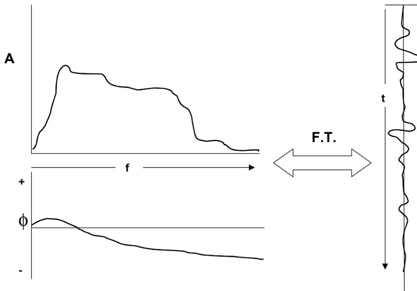
FIG. 10. After spectral clipping, amplitude and phase spectra are transformed back to a seismic trace, now with no monochromatic noise contamination.
