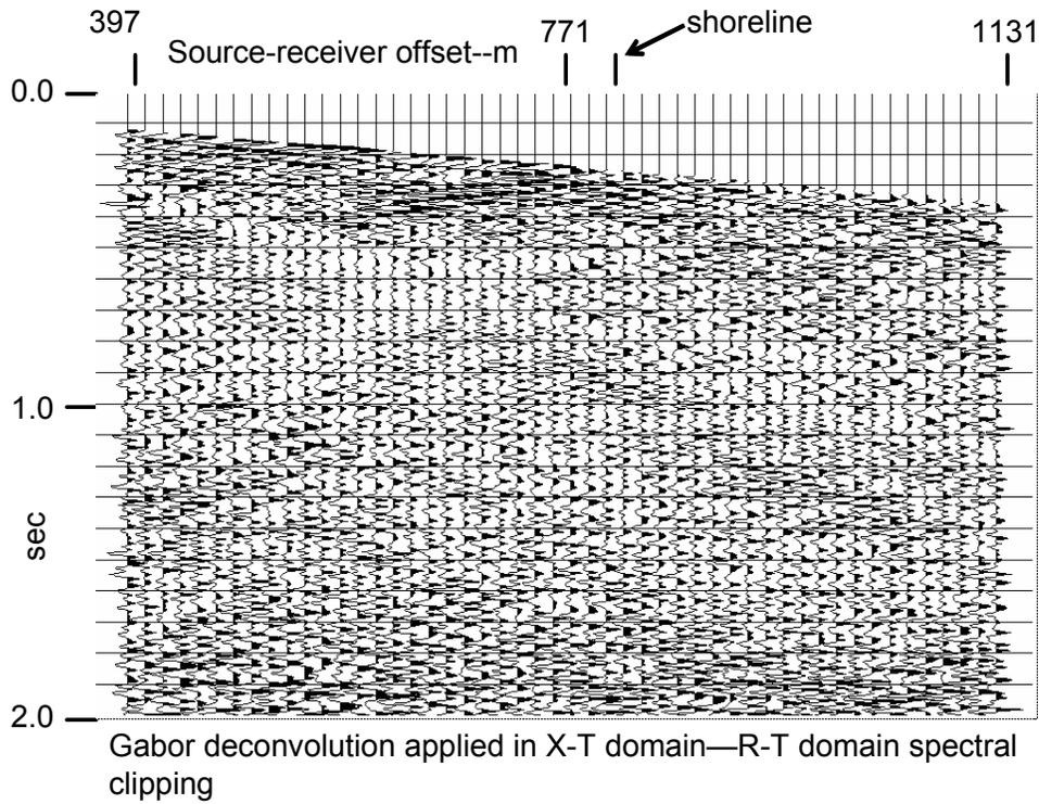
FIG. 17. Gabor deconvolution applied in X-T domain after spectral clipping in the R-T domain. This is the best result obtained yet, particularly for reflections deeper than 1.0 sec.
