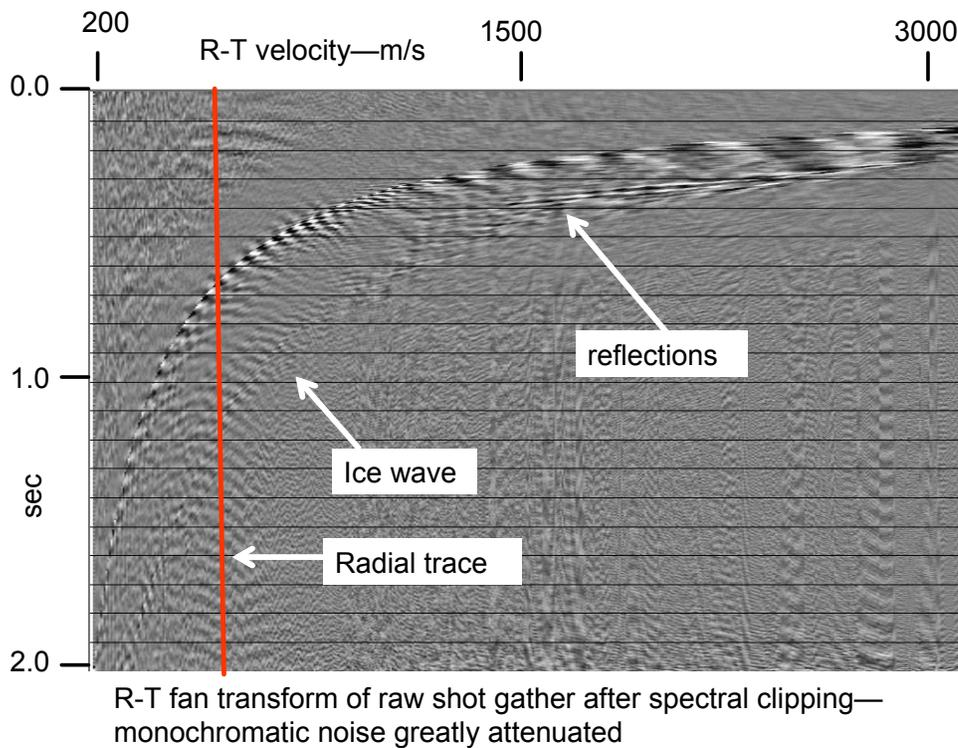
FIG. 12. R-T transform of shot gather after application of spectral clipping to the radial traces. The portion of the transform dominated by reflections is now much stronger than that dominated by the ice wave.
