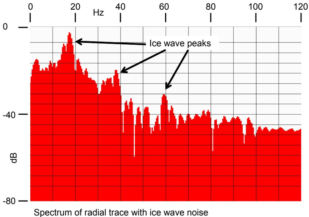
FIG. 6. The power spectrum of a radial trace at the position shown in Figure 5. Note the prominent spectral spikes just below 20, 40, and 60 Hz, all manifestations of the ice flexural wave.
