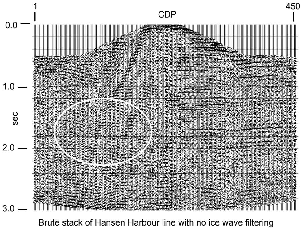
FIG. 18. Hansen Harbour stack—no ice wave filtering applied to shot gathers. Ice flexural noise dominates much of the left half of the section.
