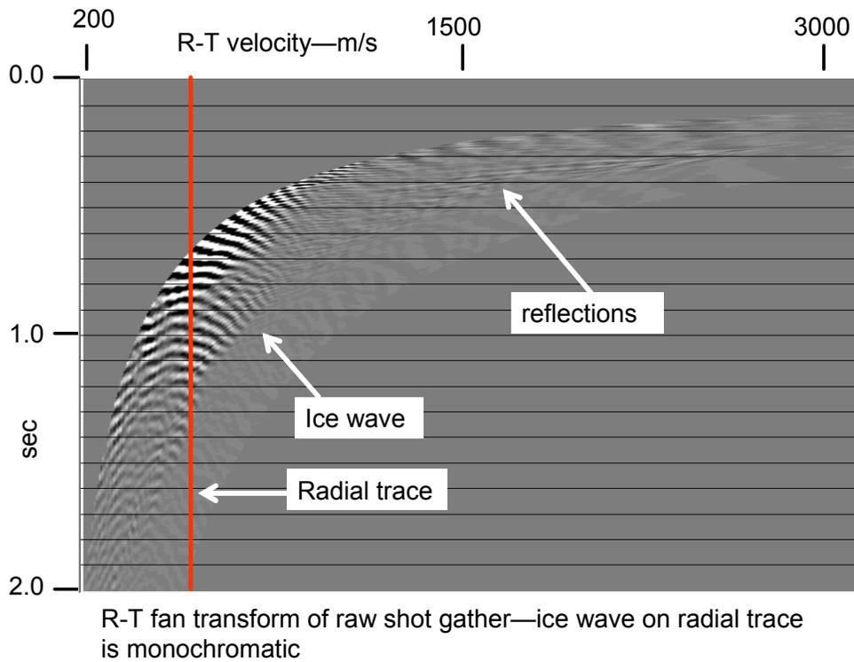
FIG. 5. Shot gather in the R-T domain. The ice wave noise is the strongest energy in the gather. Note the constant frequency of the noise along the radial trace axis (red).
