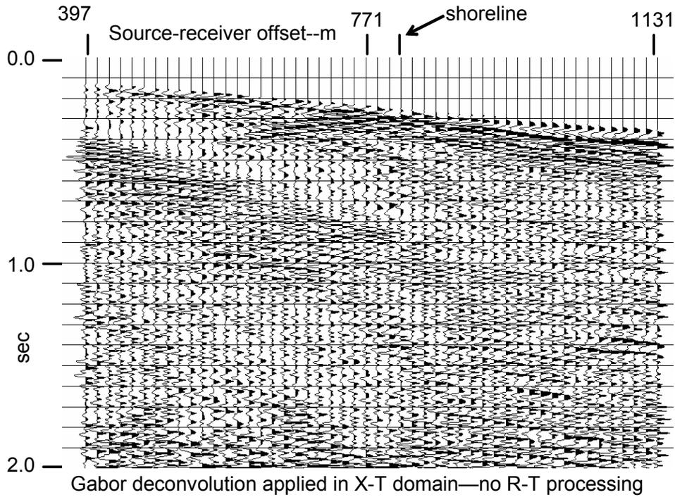
FIG. 15. Gabor deconvolution has been applied in the X-T domain to attempt to remove the ice wave noise by whitening. While an improvement over Figure 14, the imprint of the noise is still prominent.
