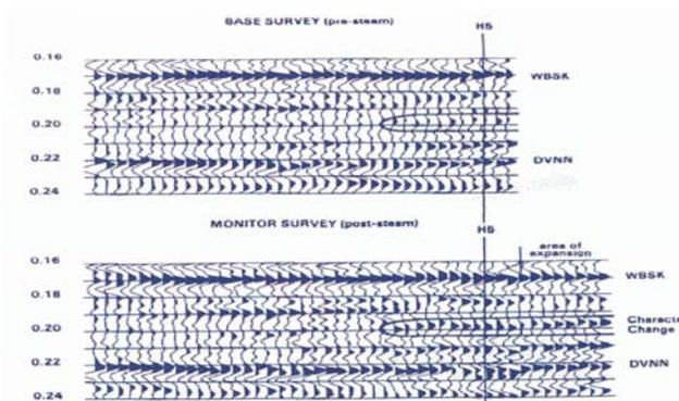
FIG. 14. Seismic amplitude change associated with pre- and post-steam surveys (from Matthews, 1992).
