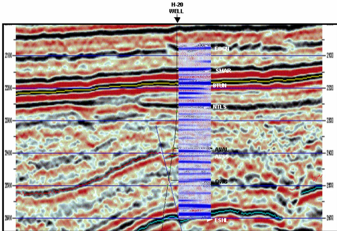
FIG. 15. Result from matching the PP synthetic (Ricker 45Hz) and streamer seismic section, showing well H-20 (modified after Emery, 2001).
