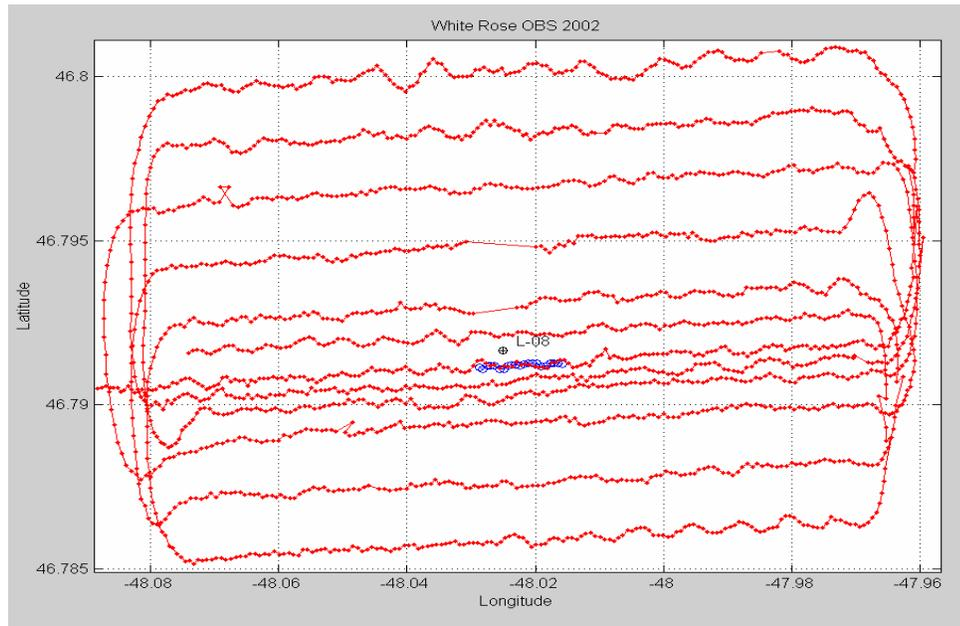
FIG. 12: Location of source lines (red) and approximate position of 21 OBS receivers (blue). (Hall and Stewart, 2002)
