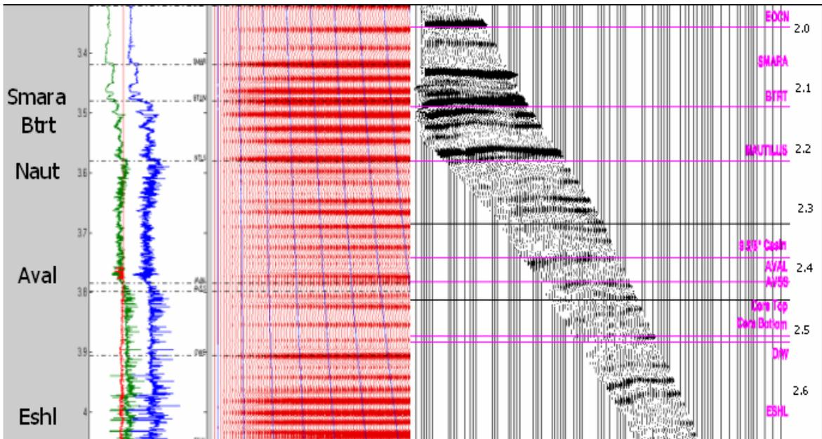
FIG. 14. Result from matching the PS synthetic (Ricker 45Hz) and the H-20 Offset VSP section.
