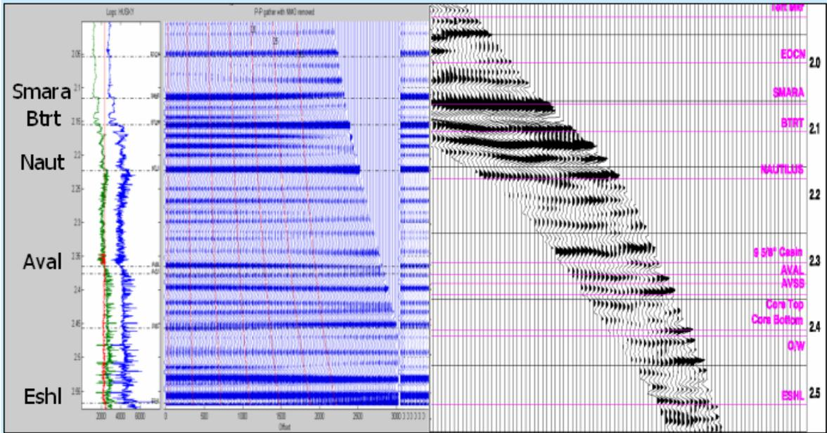
FIG. 13. Result from matching the PP synthetic (Ricker 45Hz) and the H-20 offset VSP section.
