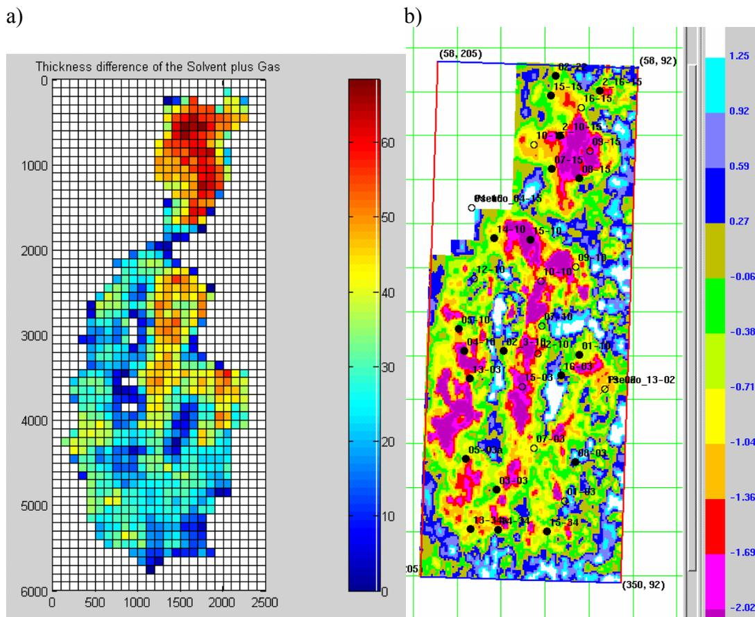
FIG. 5. a) Difference of gas and solvent thickness between 1987 and 2002 (metres). Data from the reservoir simulation. b) Time-delay map for comparison (milliseconds)
