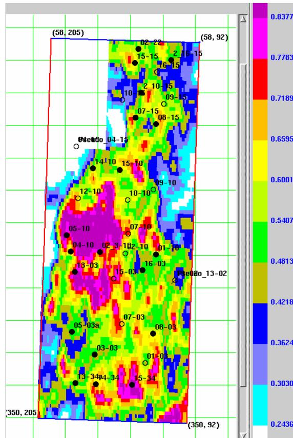
FIG. 2. Difference of Normalized RMS averaged amplitude between 1987 and the 2002 with a window centered at 20 ms on the Keg River horizon. (fractional units)
