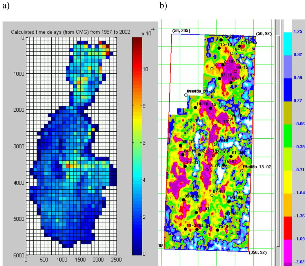
FIG. 4. a) Gassmann calculated time-delay map (seconds) based on saturation and porosity results from the reservoir simulation. These results are calculated using the Gassmann equation and the Batzle and Wang (1992) derived fluid properties. b) Time-delay map for comparison (milliseconds).
