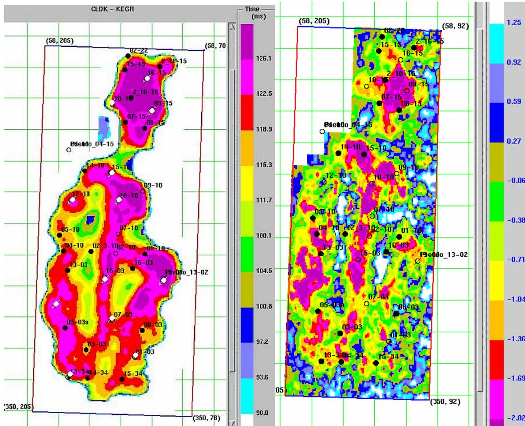
FIG. 3. a) Isochron map of the Keg River horizon to the Cold Lake horizon. The map represents the thickness of the reservoir. b) Time-delay map (milliseconds).
