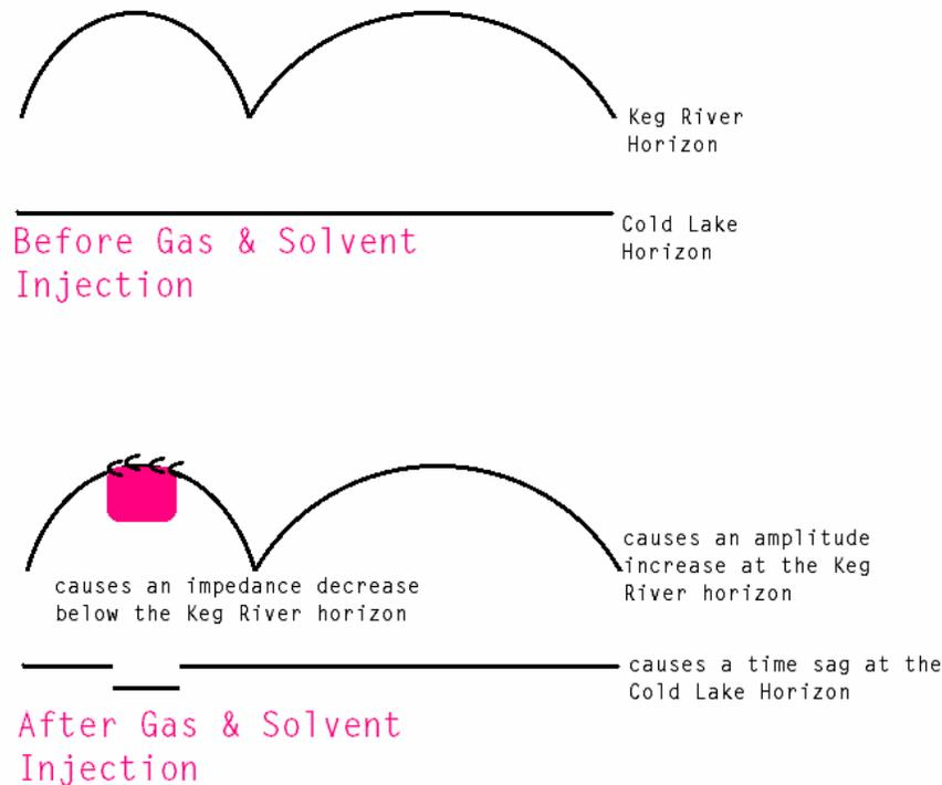
FIG. 1. Schematic diagram of seismic results expected after the injection of gas and solvent.
