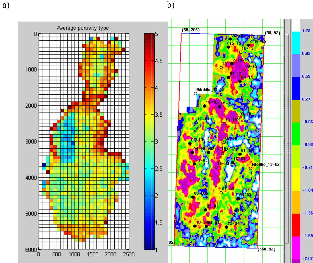
FIG. 6. a) Porosity type map: average of all the layers. Data taken from the reservoir simulation. b) Time-delay map for comparison (milliseconds)
