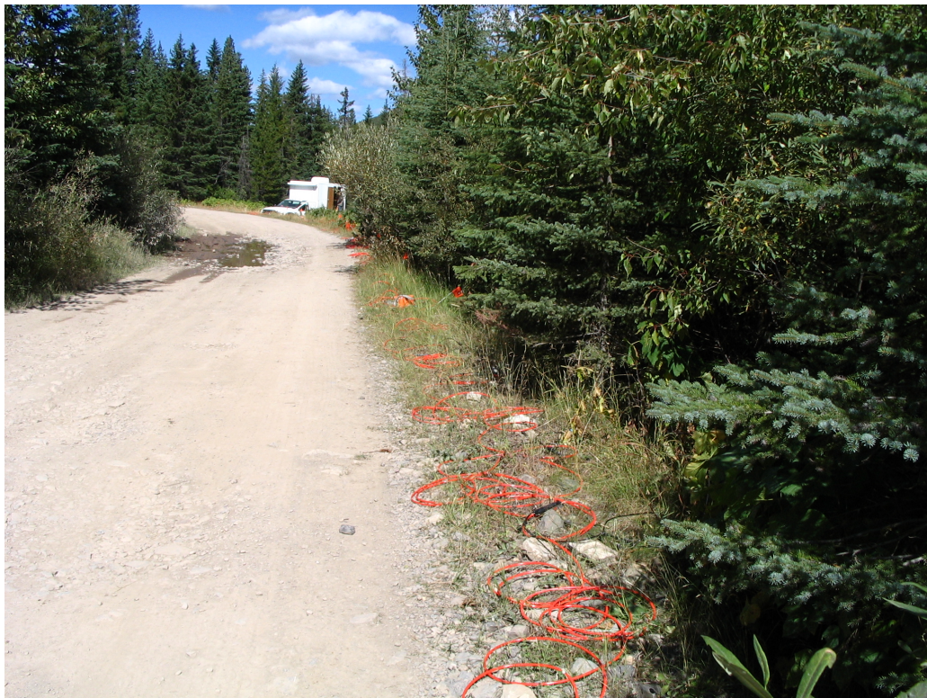
FIG.6. Aries spread at the 2005 Geophysics Field School.
