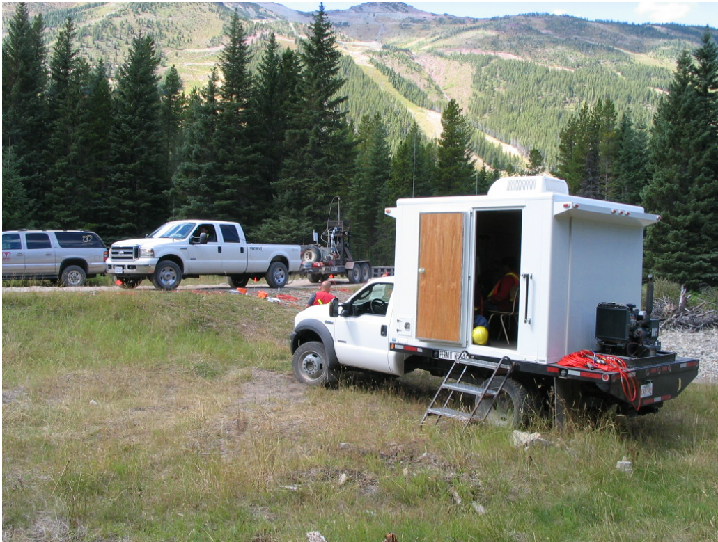
FIG. 5. The recording truck with the Aries system installed. One of the other support trucks is towing the EWG 5 source in the background.
