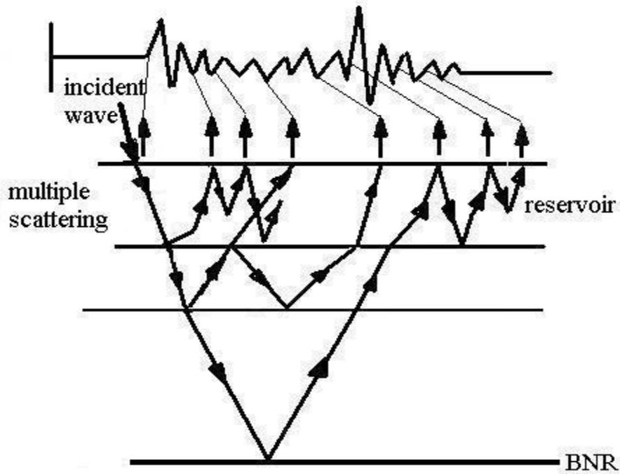
FIG. 14. Multiple scattering from the reservoir and the base near the reservoir.
