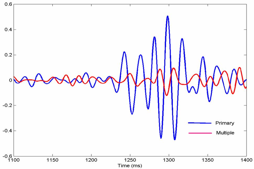
FIG. 8. There is a large difference between the primary (blue) and multiple (red) synthetic seismograms.
