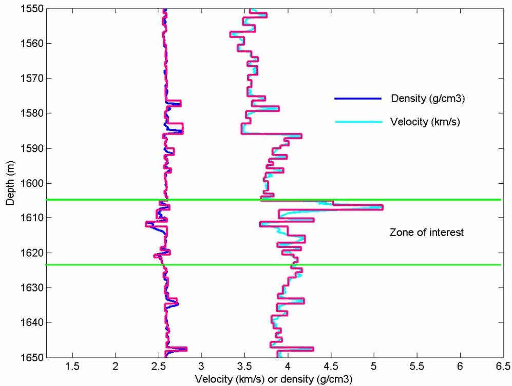
FIG. 6. Blocked density and sonic logs in the reservoir section.
