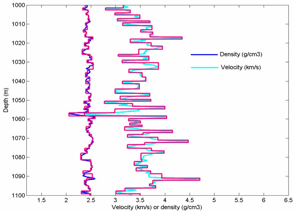
FIG. 5. Blocked density and sonic logs in the overburden section.
