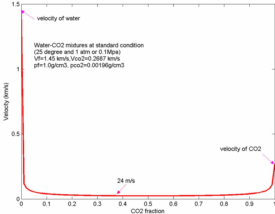
FIG. 10. Sonic velocity of a mixture of water and CO<sub>2</sub> under standard condition.
