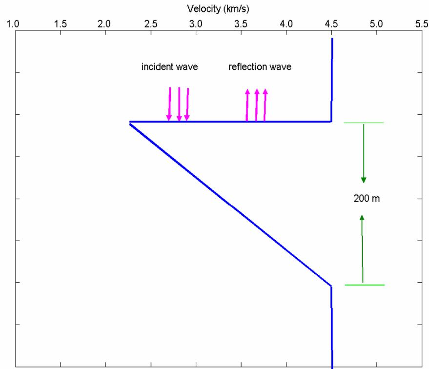
FIG. 1. An up-wedge model. The model is blocked into 20 transitional velocity layers, each 10 m thick (the velocity increases in steps of 0.1125 km/s).
