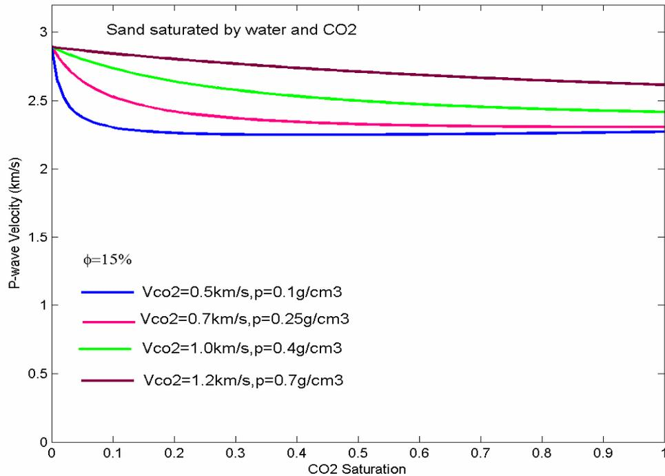
FIG. 11. Gassmann's fluid substitution for four kinds of  $\text{CO}_2$  velocities and densities.
