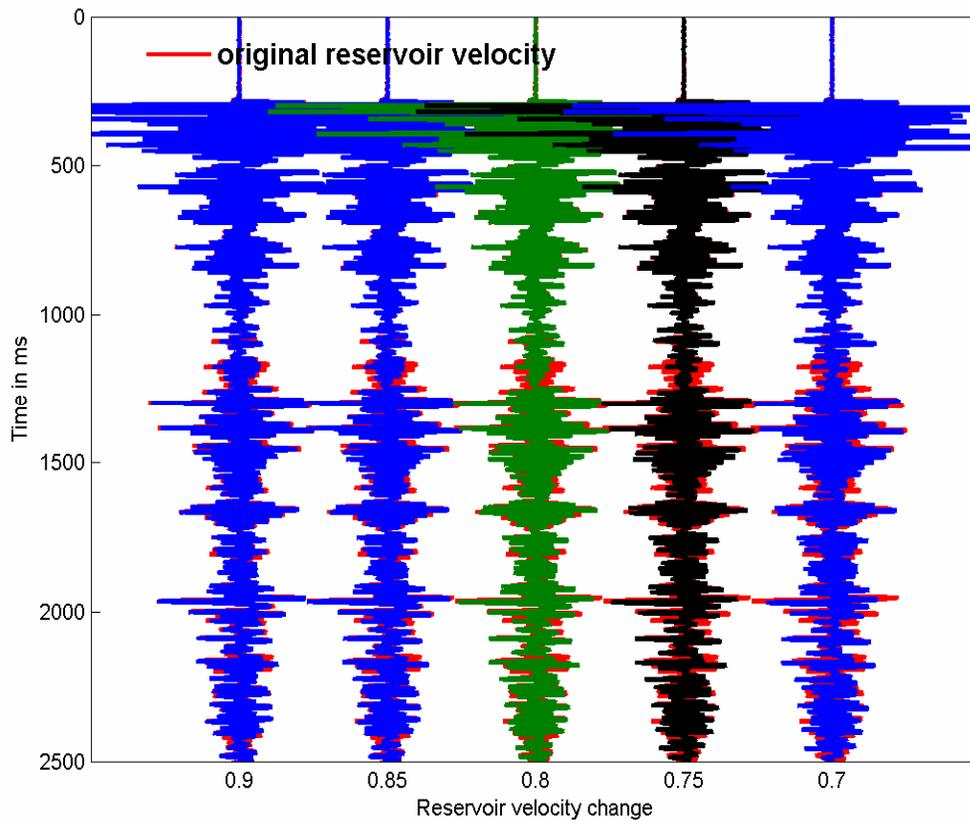
FIG. 12. The influence of reservoir velocity on seismic reflections. The red lines stand for a seismic reflection from the original reservoir velocity and the blue, green, and black lines stand for seismic reflections from five reduced reservoir velocities, respectively.
