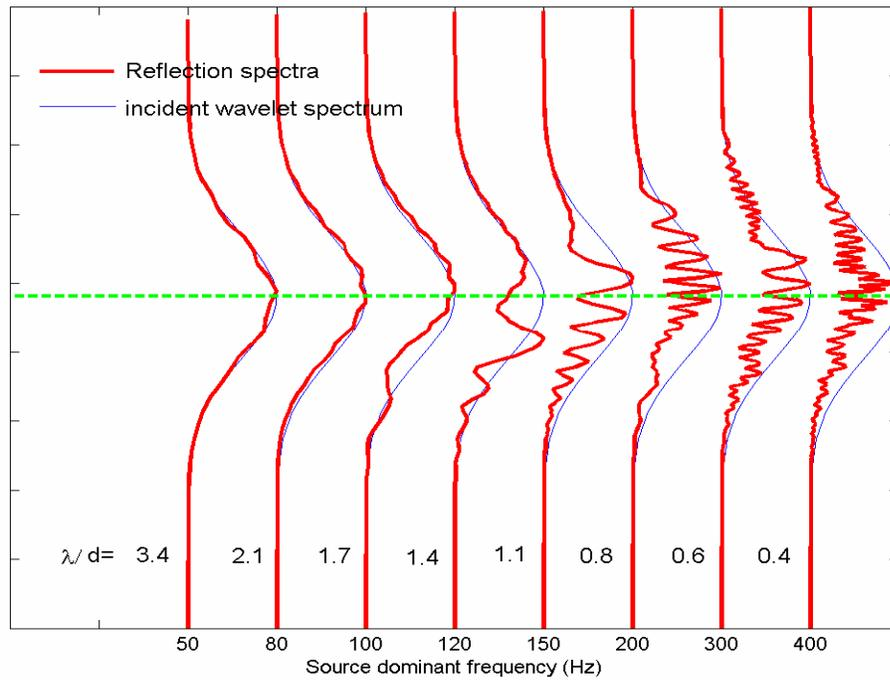
FIG. 3. Seismic reflection spectra of the traces in Figure 2.
