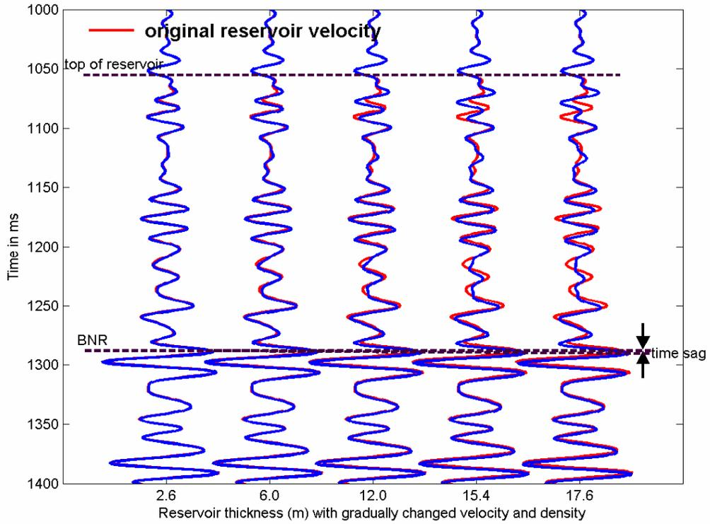
FIG. 15. The difference between seismic reflections increases with reservoir thickness.
