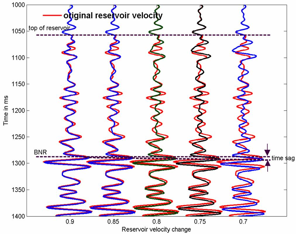
FIG. 13. The difference between seismic reflections increases with reservoir velocity changes.
