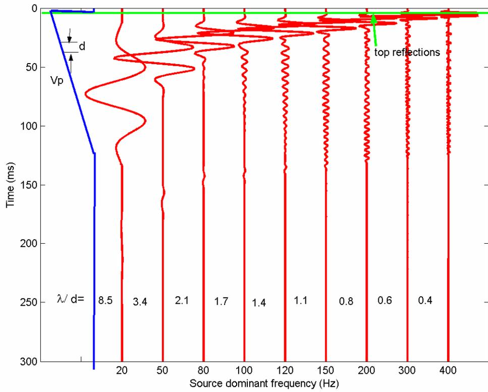
FIG. 2. Seismic reflections for the model in Figure 1.
