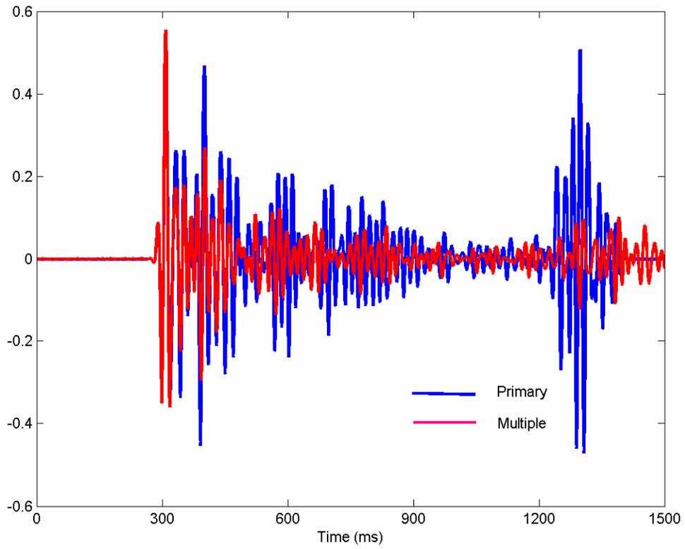
FIG. 7. Primary (blue) and multiple (red) synthetic seismograms.
