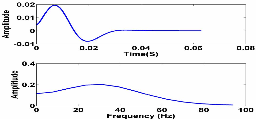
FIG. 2. Source signature and it's amplitude spectrum.
