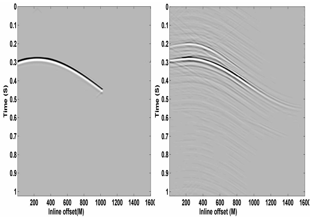
FIG. 7. Upgoing and downgoing shot gathers extrapolated to the depth of 600 m with shot point on the left side.
