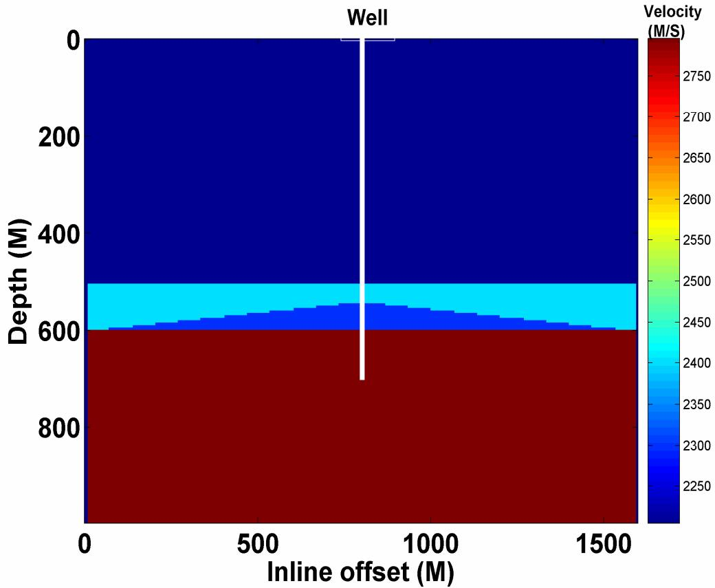
FIG. 1. Velocity field applied to the finite difference modelling.
