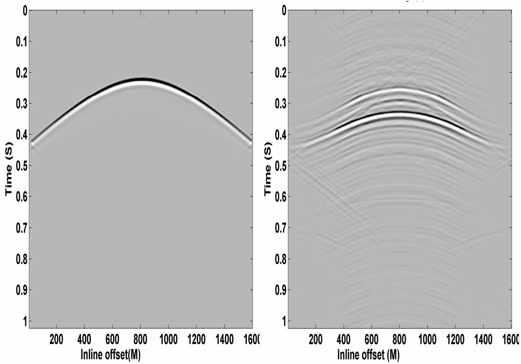
FIG. 6. Upgoing and downgoing shot gathers extrapolated to the depth of 500 m with shot point in the middle of the model.
