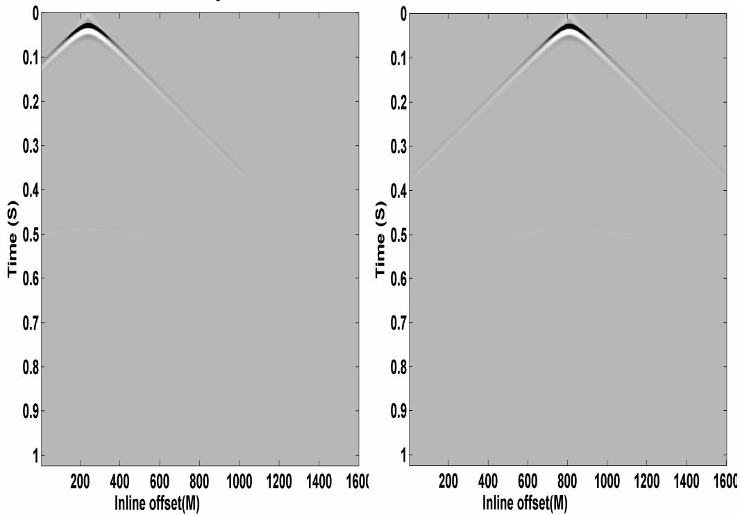
FIG. 5. Simulated downgoing waves at same depth level from two sources .
