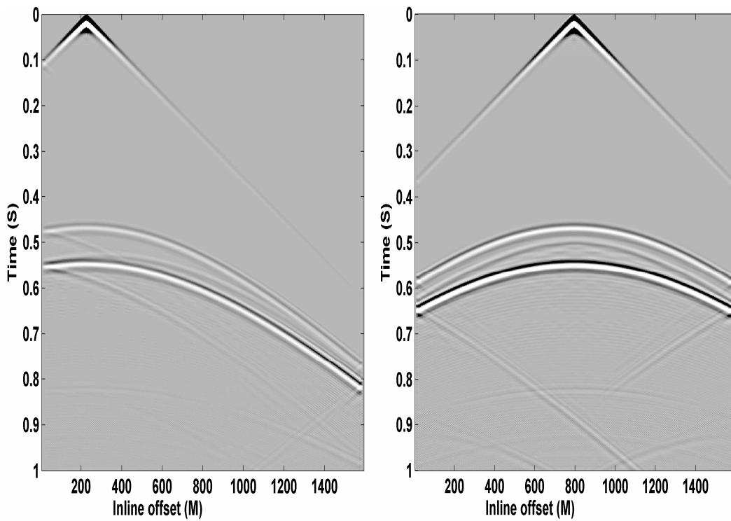
FIG. 3. Two synthetic seismic shot gathers received on the surface.
