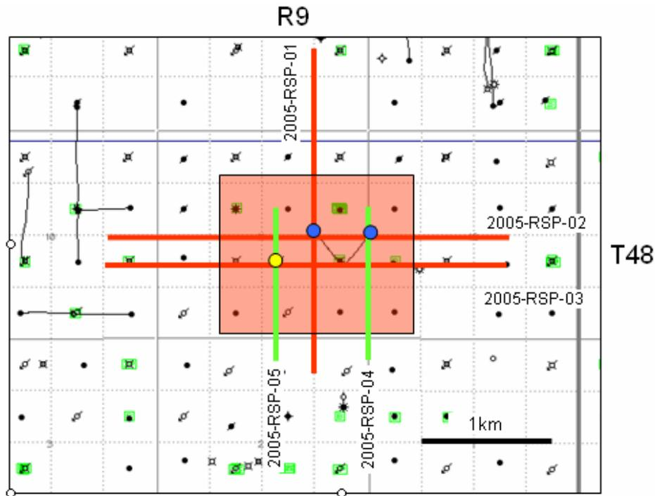
FIG. 1. Map showing the Penn West CO<sub>2</sub> injection site. Multi-component seismic lines are shown in red, receivers-only lines are shown in green. The 3D survey is shown by a semi-transparent red rectangle. The observation (VSP) well location is shown by a yellow circle, and the CO<sub>2</sub> injection well locations are shown by blue circles.
