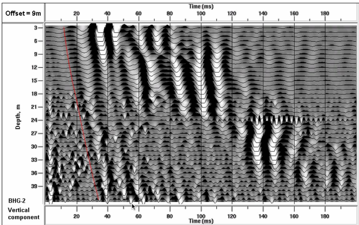
FIG. 8. Geophone-recorded VSP (vertical component) with source offset of 9 m.
