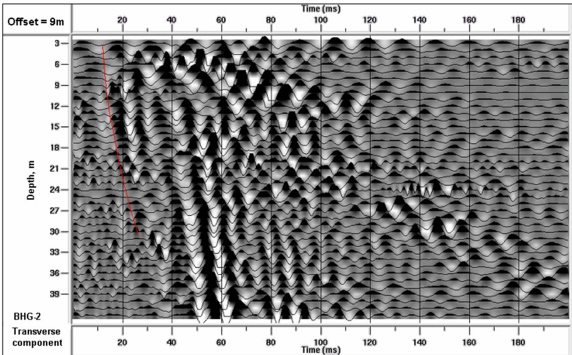
FIG. 10. Geophone-recorded VSP (transverse component) with source offset of 9 m.
