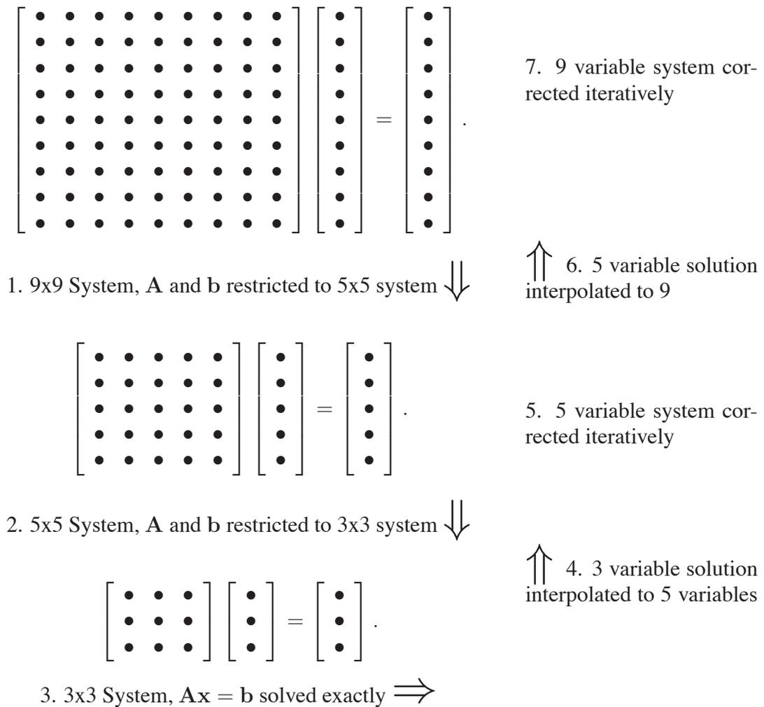
FIG. 4. A basic multigrid algorithm. A  $9 \times 9$  system of equations is reduced to a  $3 \times 3$  system using anti-alias filtering. This  $3 \times 3$  system is solved exactly, and its solution is interpolated to a finer grid. The solution is repeatedly interpolated and corrected until the original sample rate is achieved.
