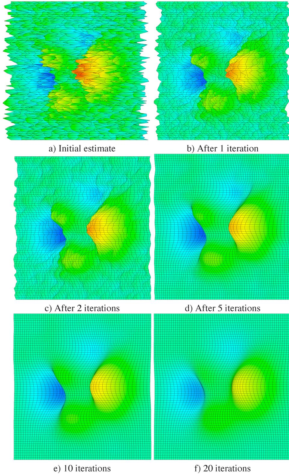
FIG. 3. The Gauss-Seidel solution to the Laplaces example. The Solution is converging to 0 throughout the domain, but the long wavelength errors are persistent.
