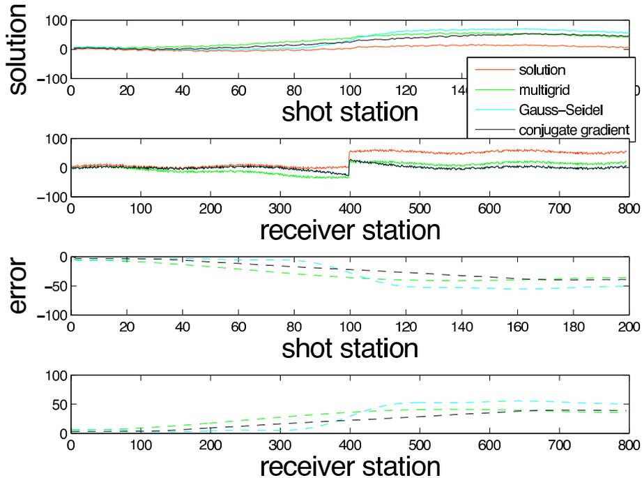
FIG. 6. The results from a 2 term surface consistent reduction. The top two axes show the calculated solutions for the shot and receiver components, the bottom axes show the error.
