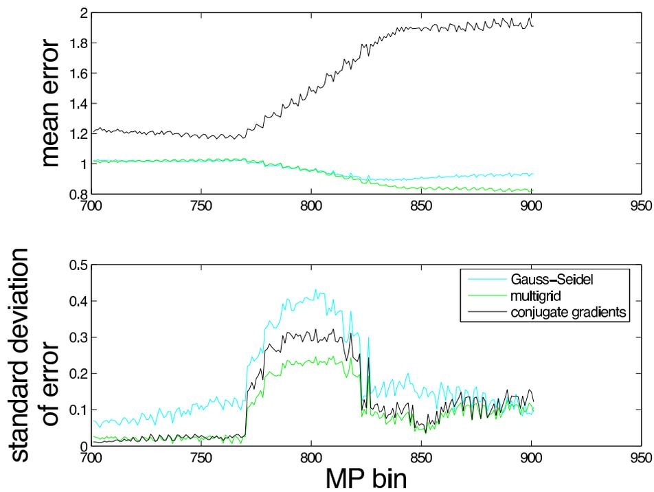
FIG. 11. Mean and standard deviation of the pre-stack variability of the amplitudes generated using the 4 term reduction. A wider standard deviation means a larger AVO error.
