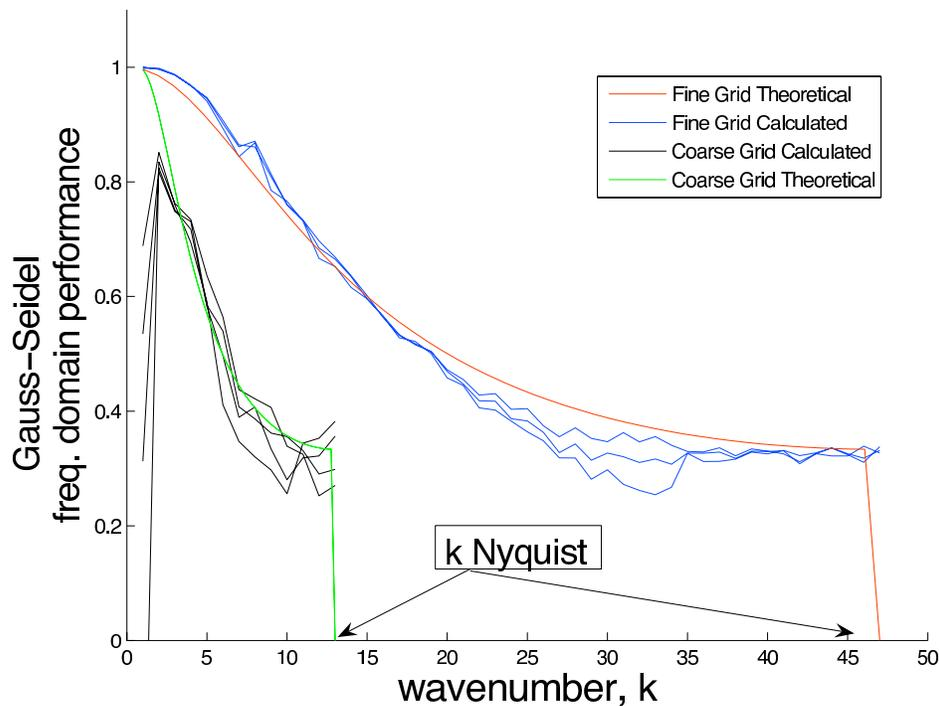
FIG. 2. The spectral efficiency of the Gauss-Seidel operator on different grid sizes for the Laplace equation.
