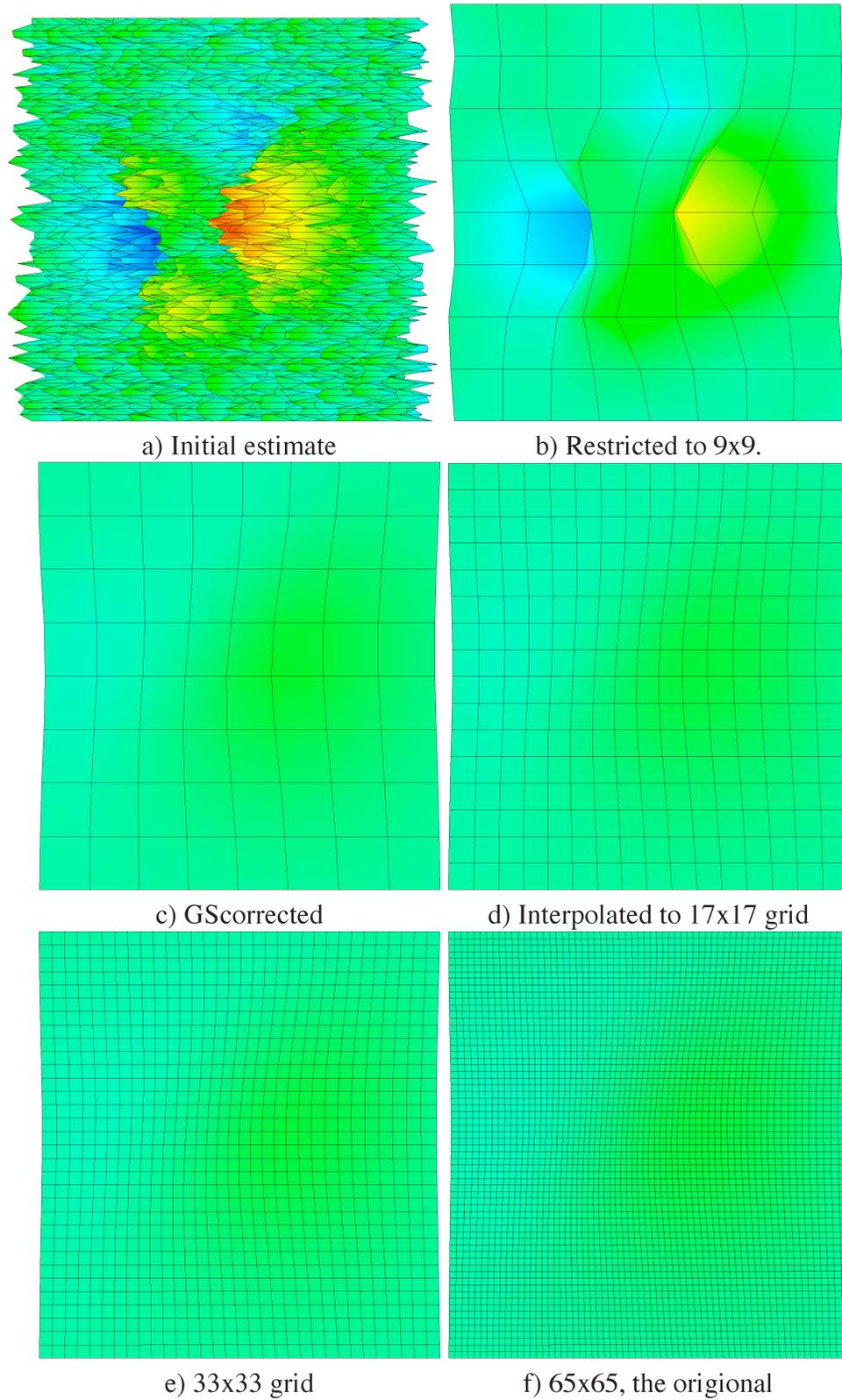
FIG. 5. The coarse grid corrected solution to the Laplace example.
