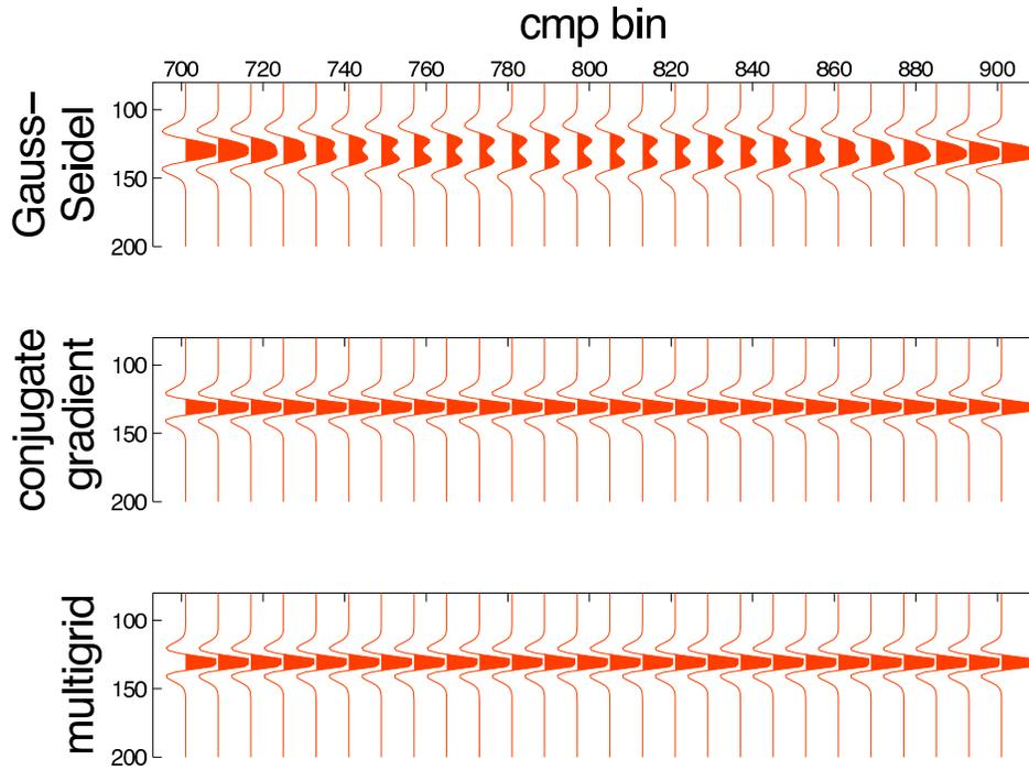
FIG. 7. The predicted stack section arising from using the various methods to solve the surface consistent equations for statics.
