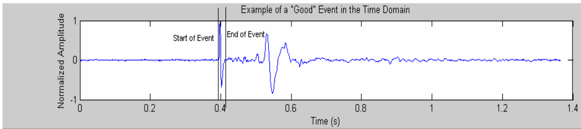
FIG. 14. Time domain plot of an example microseismic “good” event.
