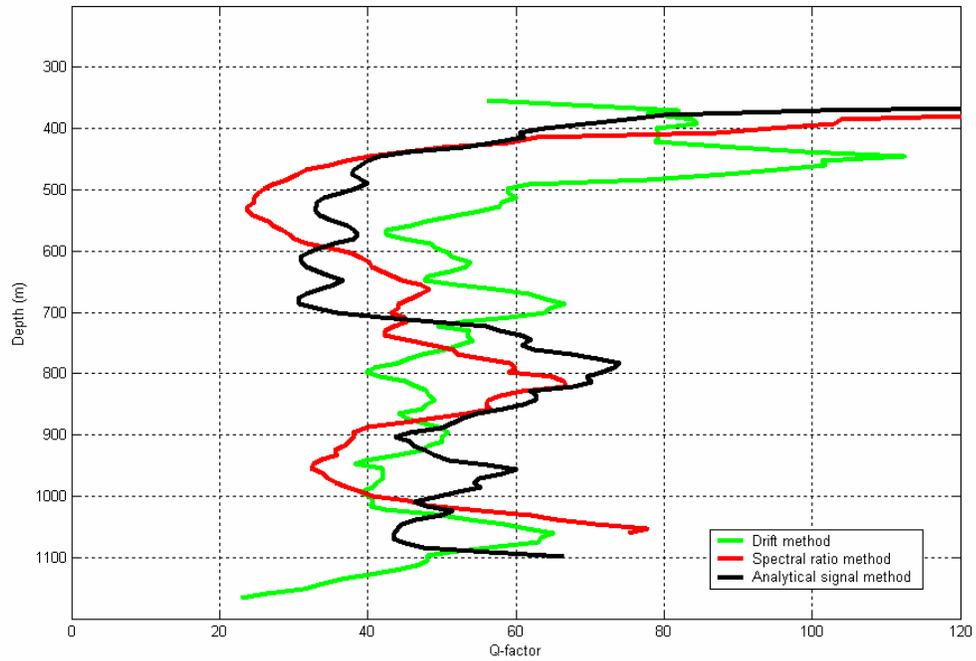
FIG. 4. Q versus depth for zero offset Ross Lake VSP (360 m estimation interval).
