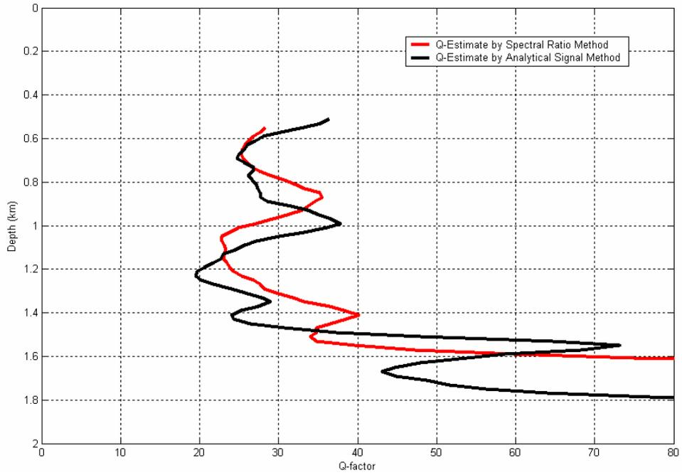
FIG. 2. Q versus depth for zero offset Alberta VSP (360 m estimation interval).
