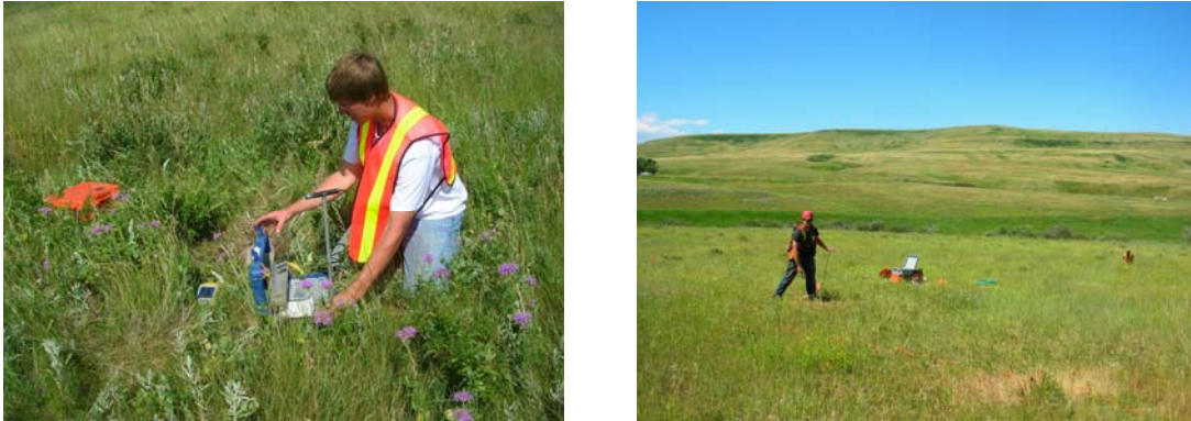
FIG.2. Vibration monitor setup (left) and shooter ready to fire a source point (right).
