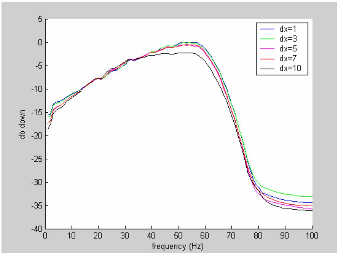
FIG. 5. Average amplitude spectrum of shot records with various grid sizes.
