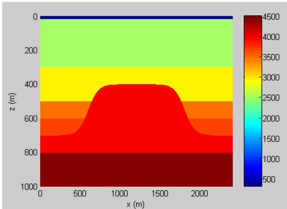
FIG. 3. Reef velocity model used in analysis and modelling.
