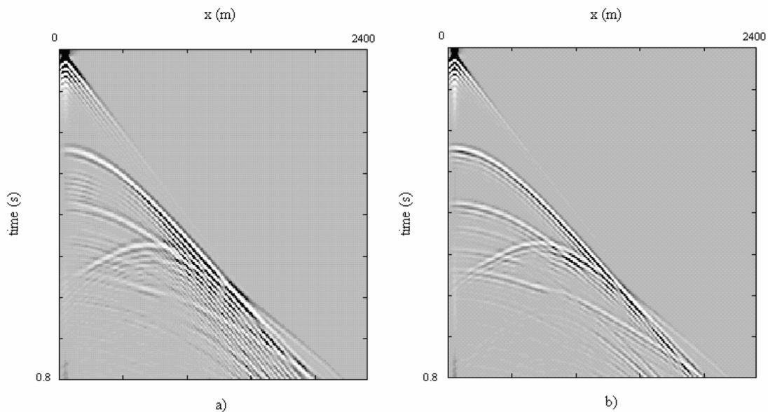
FIG. 4. Shot records for a 10m (a) and 1m (b) spatial sampling grid.
