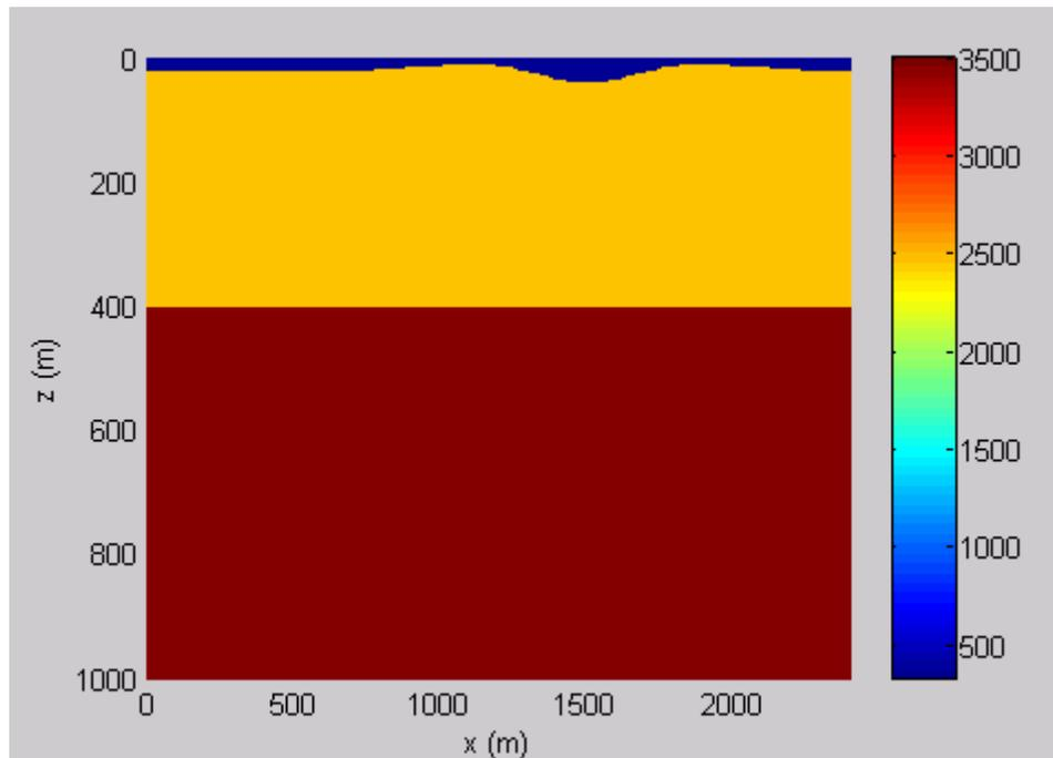
FIG. 1. Two layer velocity model with a varying topographic surface.
