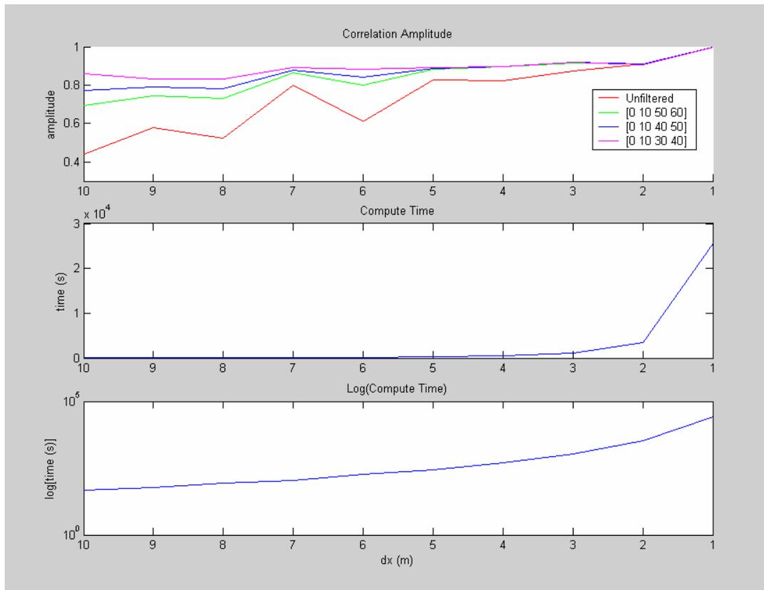
FIG. 6. Correlation amplitude and compute time for various grid sizes and filters.
