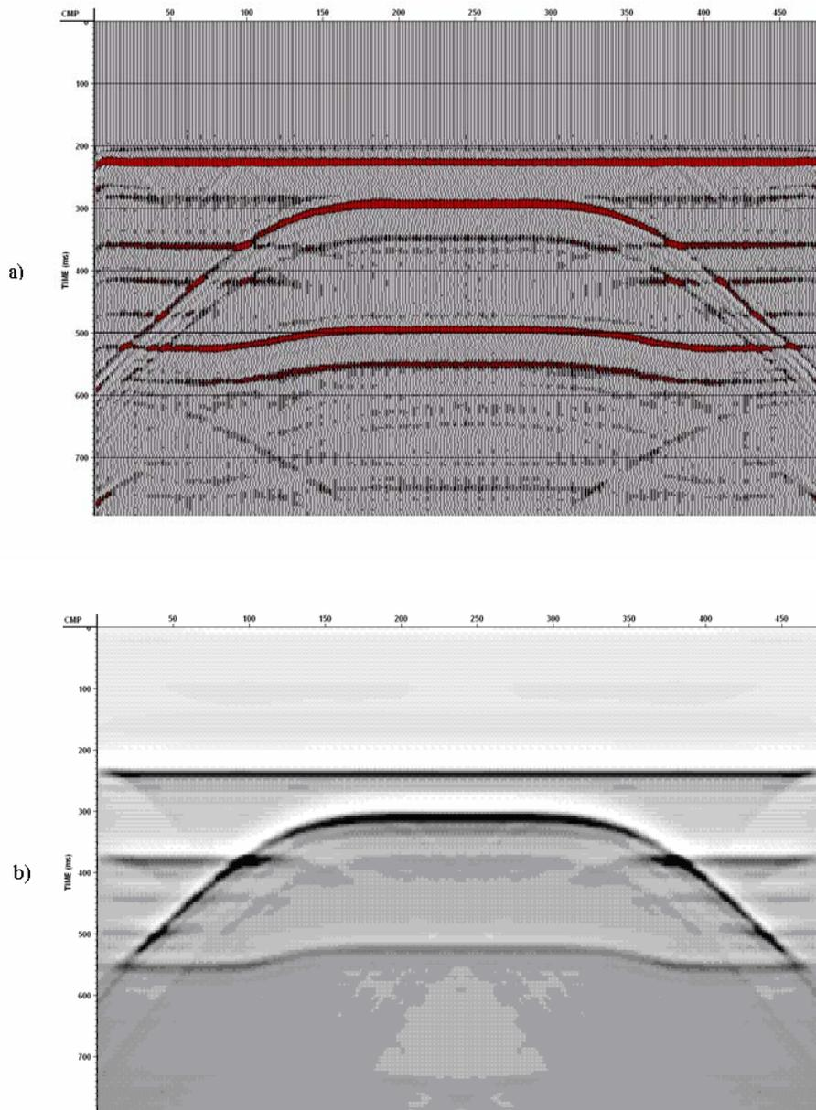
FIG. 8. a) CMP stack processed with VISTA. b) NIS image generated with *afd\_explode*.
