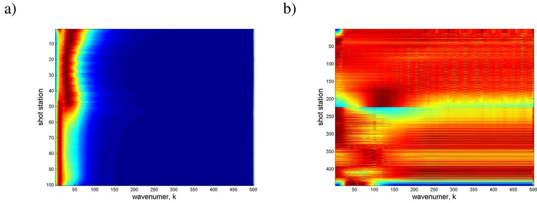
FIG. 16. The frequency spectrum of the shot consistent (a) and receiver consistent (b) solution calculated using the gauss-Seidel method, including ground roll
