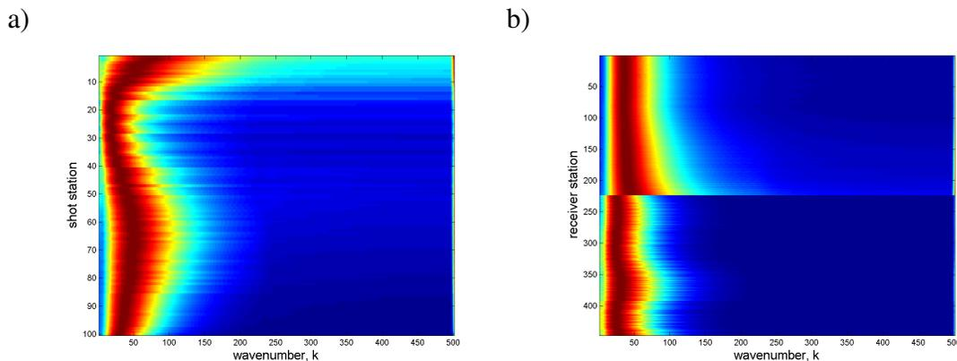
FIG. 10. The frequency spectrum of the shot consistent (a) and receiver consistent (b) solution calculated using the multigrid method
