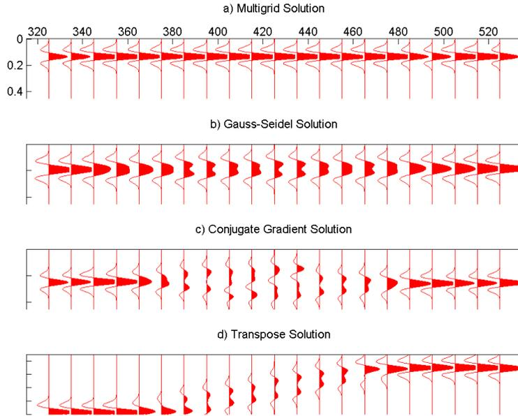
FIG. 6. The effect on the error in our surface consistent static solutions on a midpoint stack section. The  $x$  axis labels denote the midpoint station. Not all midpoints are plotted.
