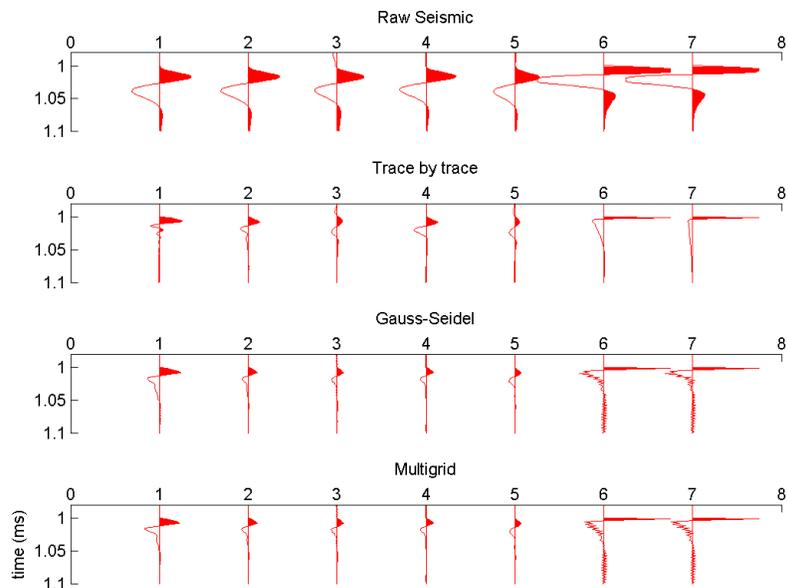
FIG. 18. Midpoint gather showing the results of our 2 term surface consistent deconvolution, when ground roll is added
