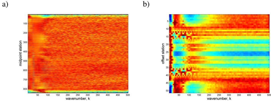
FIG. 25. The midpoint (a) and offset (b) consistent terms, calculated by the Gauss-Seidel method
