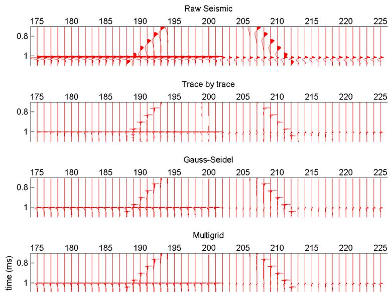
FIG. 15. A shot record, showing the effect of the 2 term surface consistent deconvolution, when ground roll is added to the raw traces.
