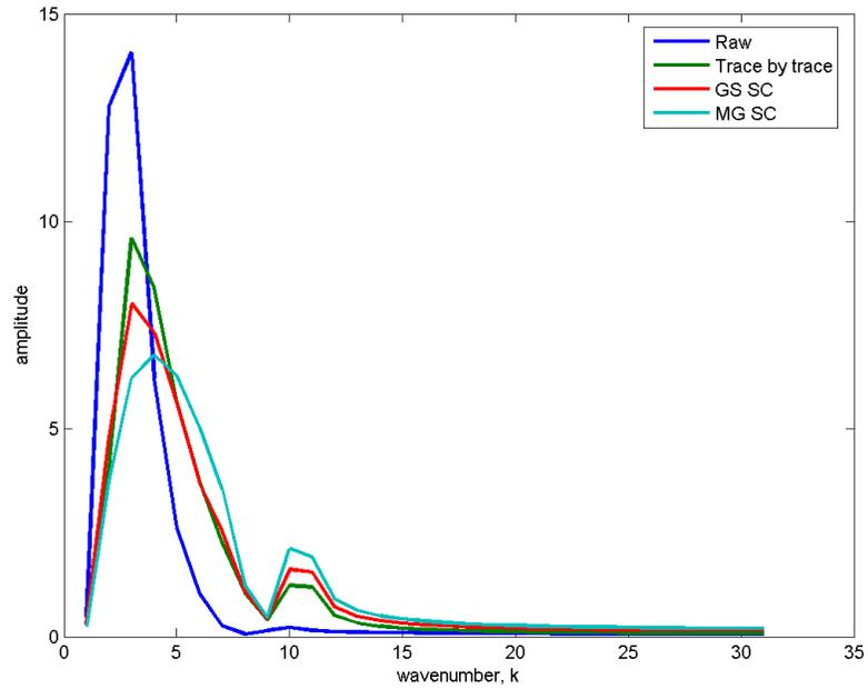
FIG. 28. The Fourier transform of the midpoint stacked trace, including the ground roll, random noise and using the four term surface consistent equations. The surface consistent operators whiten the reflector more than the trace by trace deconvolution, with the multigrid operators boosting frequencies near wavenumber 7 by more than the Gauss-Seidel operators
