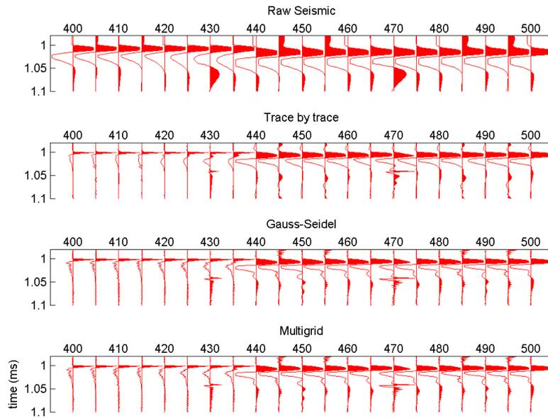
FIG. 19. Midpoint stack section of the example containing ground roll, and the deconvoluted sections using the 2 term surface consistent equations.
