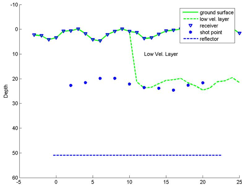
FIG. 1. A diagram of the physical model that we use for the synthetic surface consistent system
