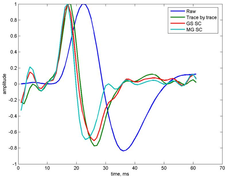
FIG. 27. A stacked trace from midpoint 445 from the synthetic seismic example, deconvolved using the 4 term surface consistent equations
