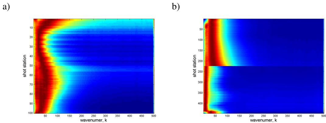
FIG. 17. The frequency spectrum of the shot consistent (a) and receiver consistent (b) solution calculated using the multigrid method, including ground roll
