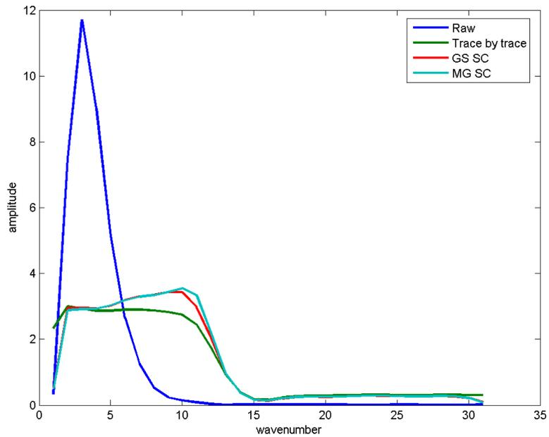
FIG. 14. Amplitude spectrum of the midpoint stacked trace at station 445. The spectrum of the trace by trace deconvolution is more flat than the surface consistent operators.
