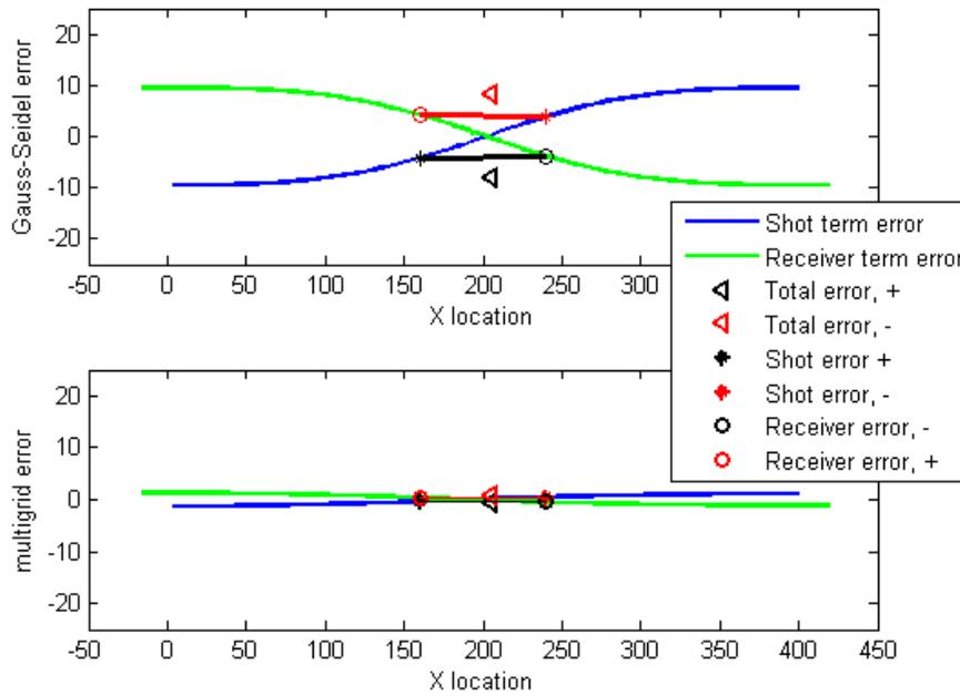
FIG. 5. The shot and receiver error terms for the surface consistent model
