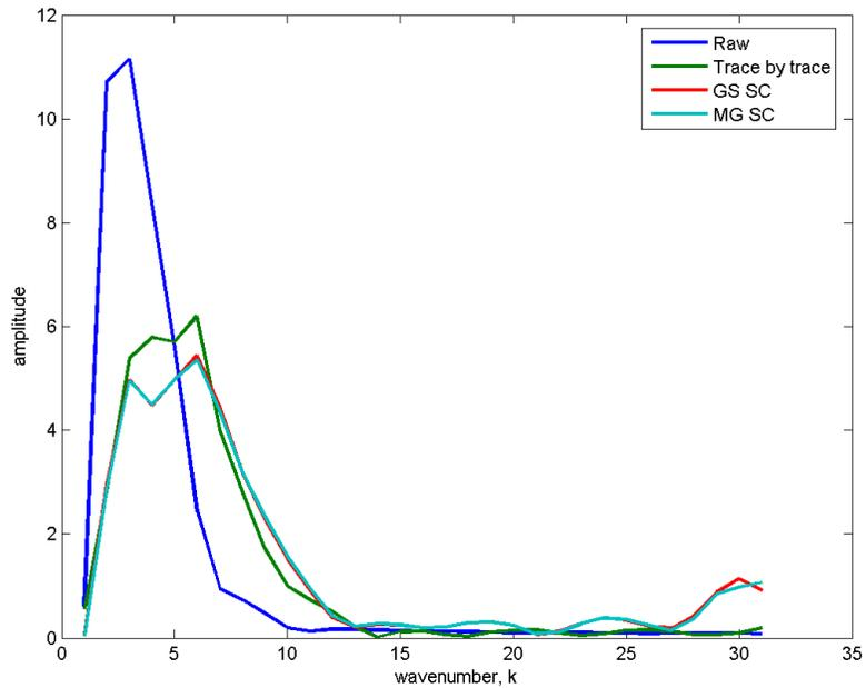
FIG. 21. The amplitude spectrum of the reflector from midpoint 445, including ground roll. The multigrid and Gauss-Seidel surface consistent operators provide a more white spectrum, boosting the frequency content near wavenumber 10 slightly.
