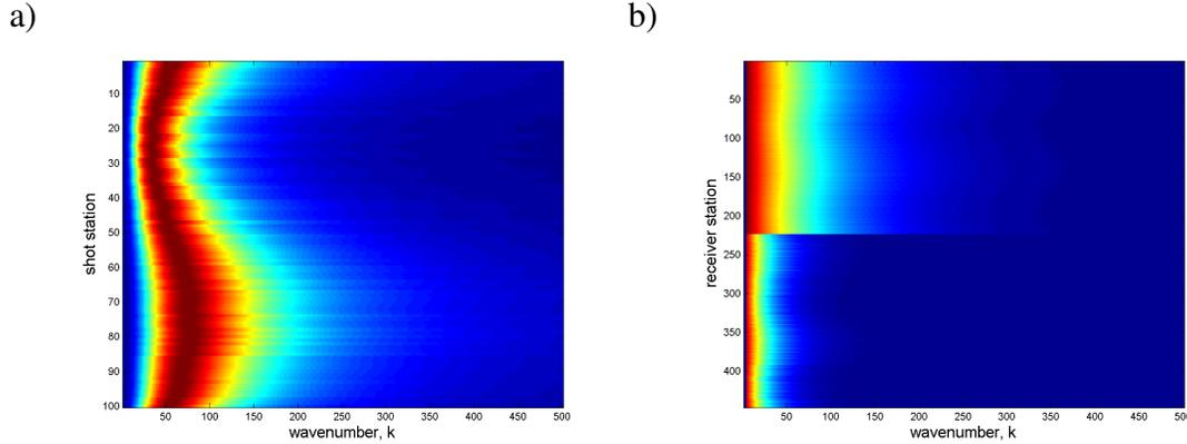
FIG. 7. The frequency spectrum of the shot consistent (a) and receiver consistent (b) solution we use to forward model our surface consistent deconvolution problem
