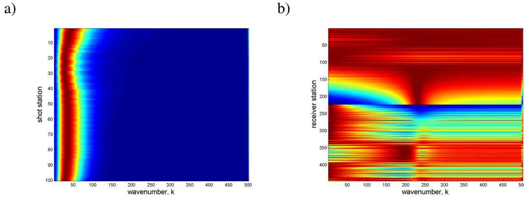
FIG. 9. The frequency spectrum of the shot consistent (a) and receiver consistent (b) solution calculated using the Gauss-Seidel method
