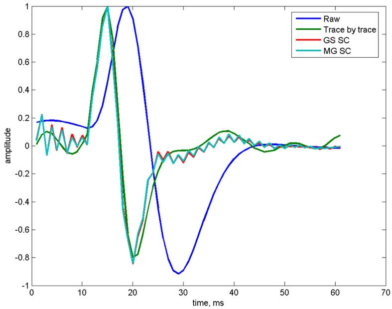
FIG. 20. A stacked trace of midpoint 445, when using a 2 term deconvolution on an example that contains ground roll
