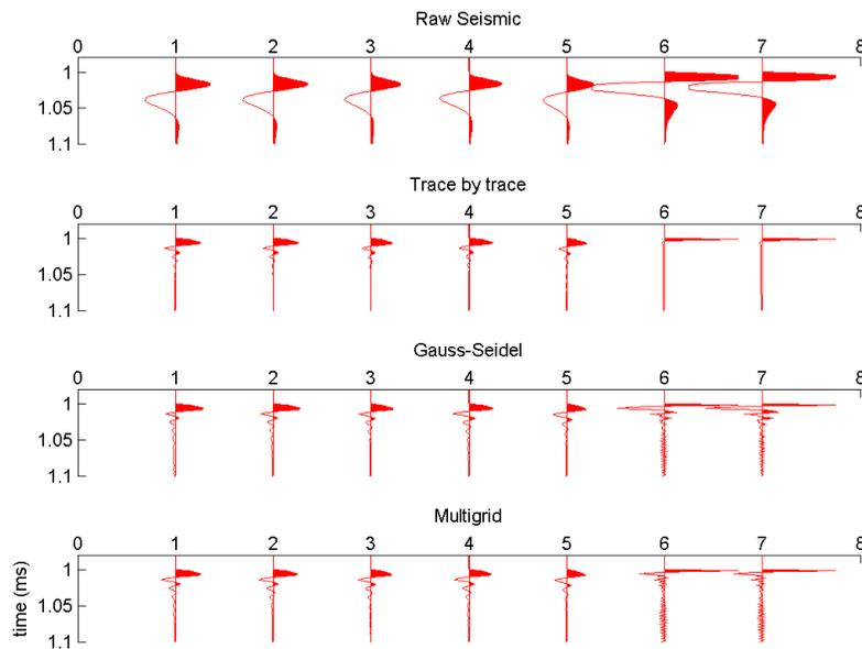
FIG. 11. A common midpoint gather near the receiver consistent anomaly, raw and deconvolved data. The midpoint station number is 445
