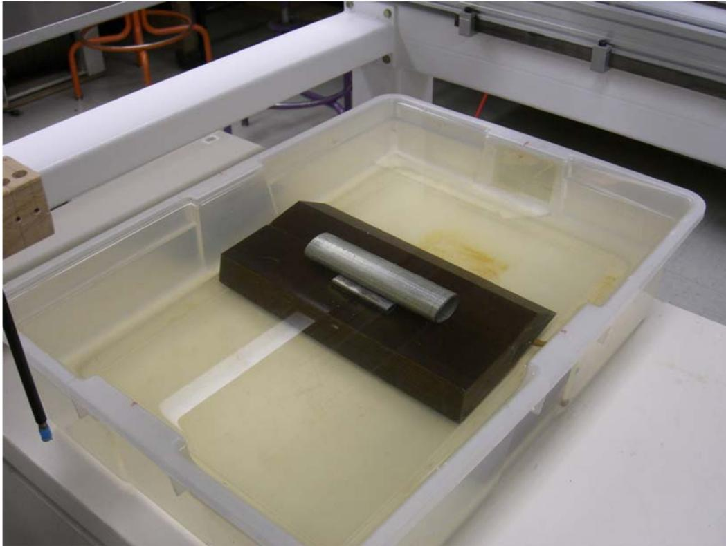
FIG. 5a. Close-up photograph of Model #2 (phenolic body and steel tubes in water).
