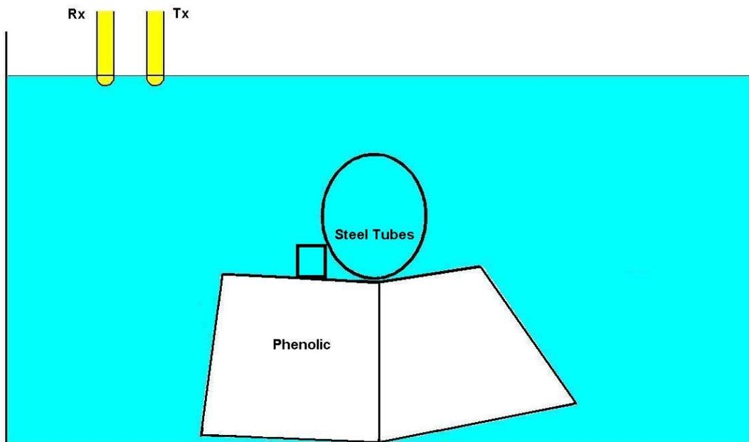
FIG 5b. Schematic diagram showing the geometry of the 2D survey over Model #2.
