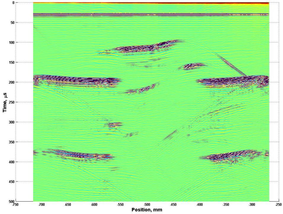
FIG. 4a. Common offset gather for Model #1. Note the presence of multiples.
