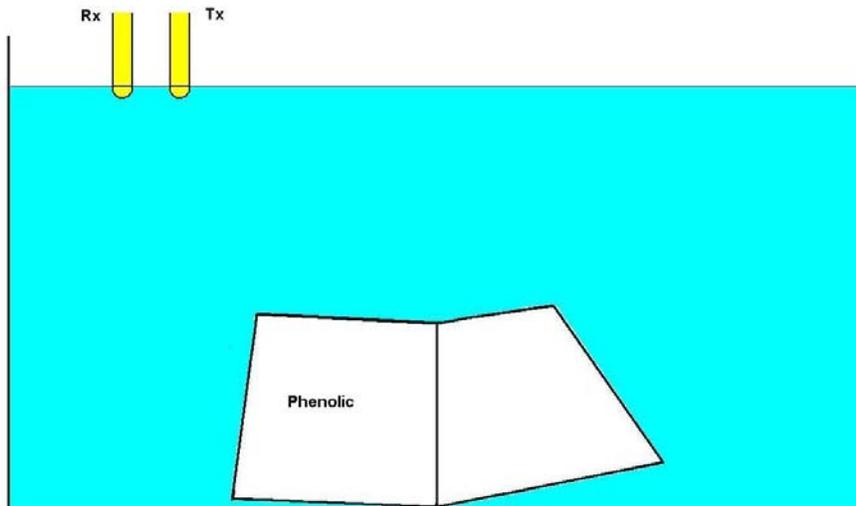
FIG. 3b. Schematic diagram showing the geometry of the 2D survey over Model #1.
