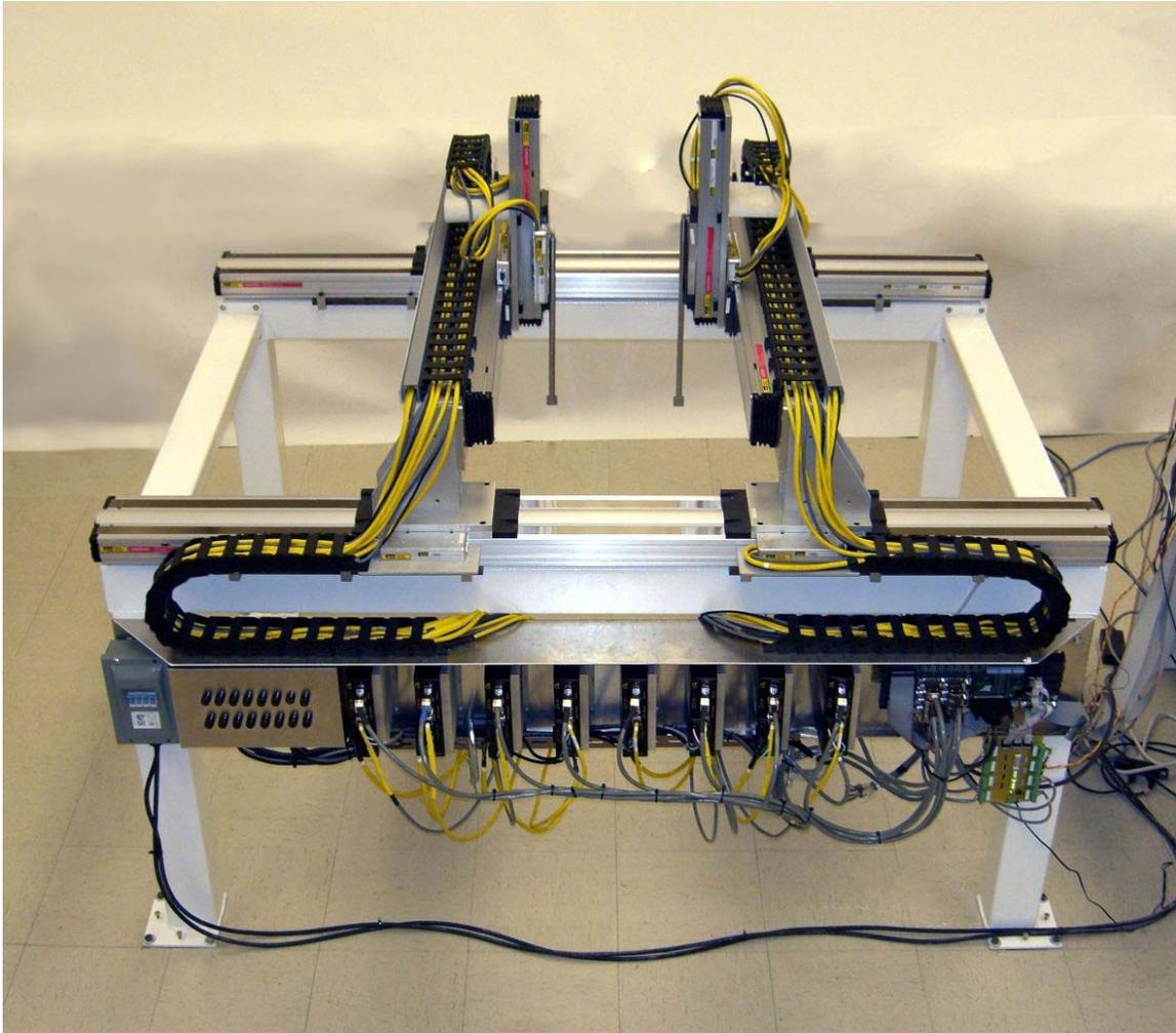
FIG. 1. Positioning system with 8 linear motors for the Physical Seismic Modelling Facility (From Bland et al., 2006).
