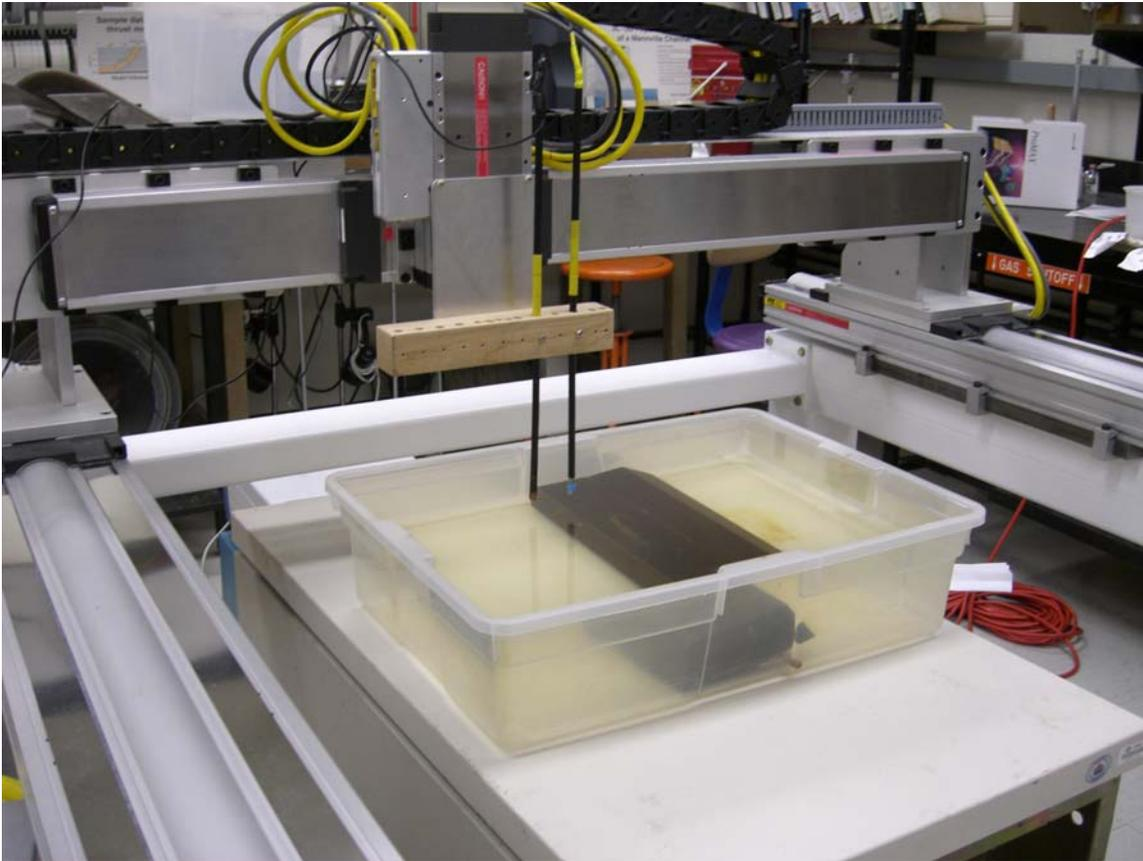
FIG. 2. Rx and Tx transducers mounted over a phenolic model in water.
