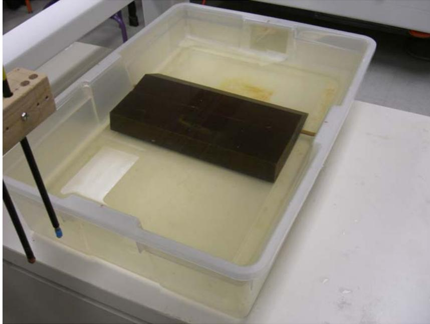
FIG. 3a. Close-up photograph of Model #1 (phenolic body in water).
