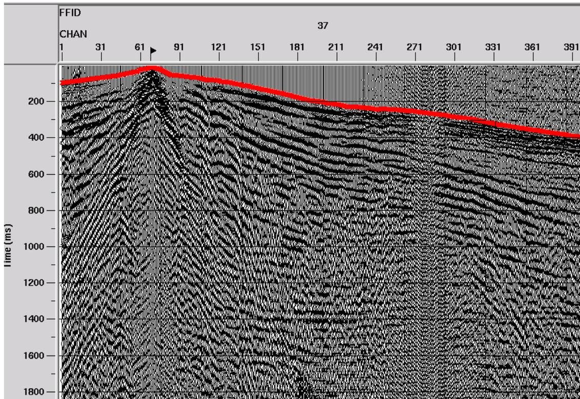
FIG. 2. Example shot gather from near the south end of the line. Good reflectivity can be seen down to 1400 ms. The noise at channels 271-301 is due to a diesel generator on the recording truck.
