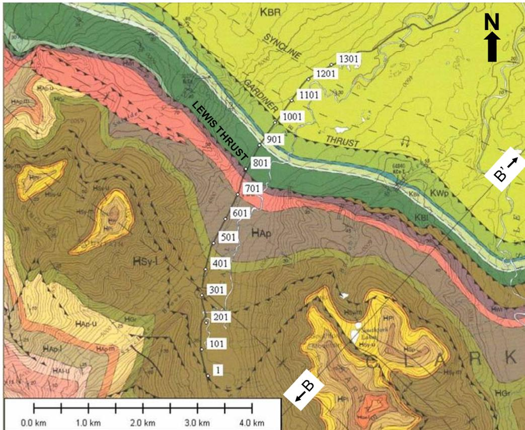
FIG. 1. Part of geology map (Norris, 1993) with every hundredth CDP location posted. Seismic survey crosses the Akamina syncline (CDP 301), Lewis thrust (801), Gardiner thrust (1001) and Lost Creek syncline (1250). Cretaceous rocks are northeast of the Lewis thrust (green), Proterozoic rocks are southeast.
