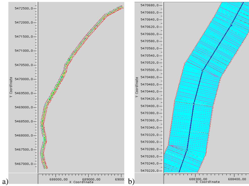
FIG. 4. Crooked-line CDP binning for the Castle mountain survey (a) and a close-up (b) showing detail of some of the corner bins.
