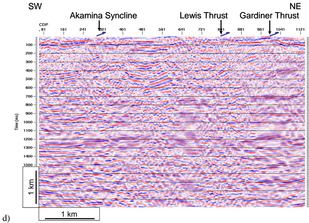
FIG. 6. Final post-stack phase-shift migrated sections. Figures 6a (SW), 6b and 6c (NE) show close-ups with a horizontal exaggeration of about 3.2:1; Figure d shows the entire section with a horizontal exaggeration of about 1.5:1. Time to depth conversion assumes 5000 m/s.
