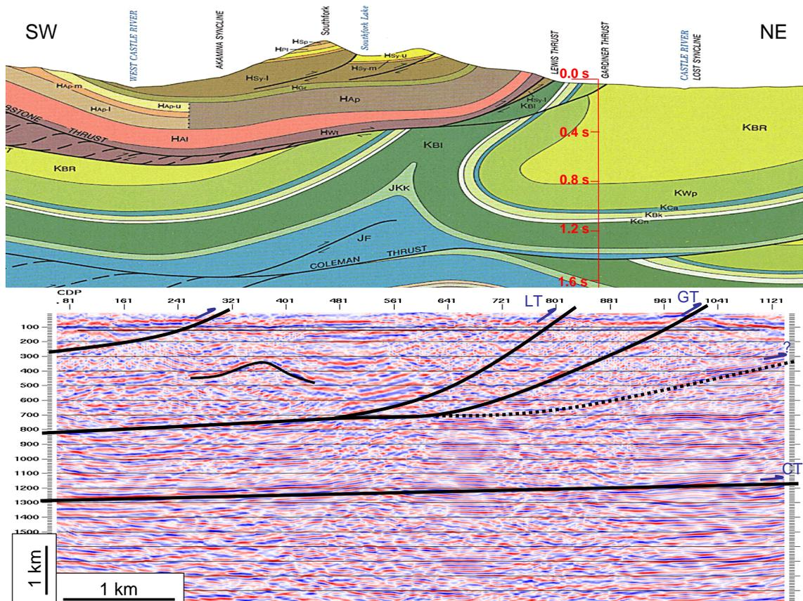
FIG. 7. Comparison of part of B-B' cross-section (top; Norris, 1993) to migrated section. LT = Lewis Thrust, GT = Gardiner Thrust; CT = Coleman Thrust. Section tied to cross-section at Akamina syncline and Lewis thrust. Horizontal exaggeration 1.5:1. Measured dips at the surface near the seismic line are 30-50 degrees (Norris, 1993).
