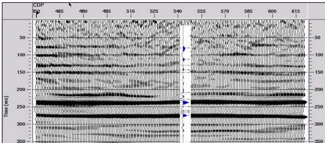
FIG. 10. Time migrated vertical component section showing a synthetic tie. The Ardley Coals are between 220 and 280 ms.
