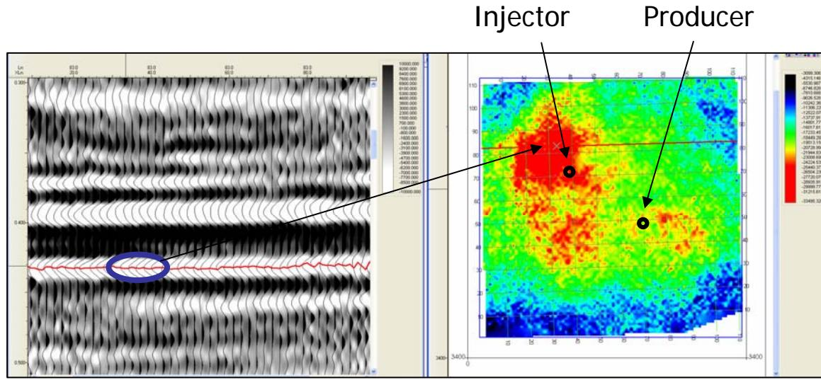
FIG. 14. Vertical component data. On the left is the pick of the target coal event. On the right is the amplitude map of the picked event. The line displayed on the left is the east-west (inline) line just north of the injector well. The blue circle on the left highlights the high amplitude anomaly that is shown by the red colour on the right hand side.
