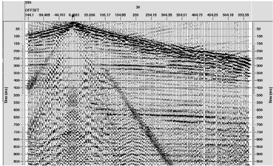
FIG. 5. A vertical component shot record after three passes of radial trace filtering.
