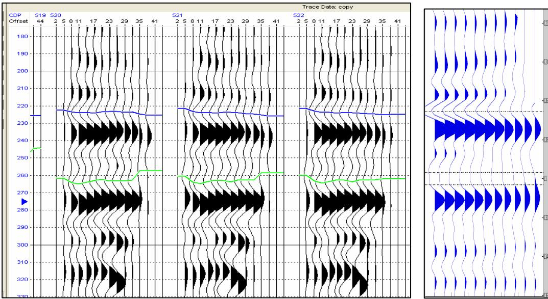
FIG. 11. CDP gathers of the vertical component data. The blue event correlates to the Upper Ardley Coals and the green event correlates to the upper seam of the Lower Ardley Coals. The AVO synthetic seismogram on the right is for comparison.
