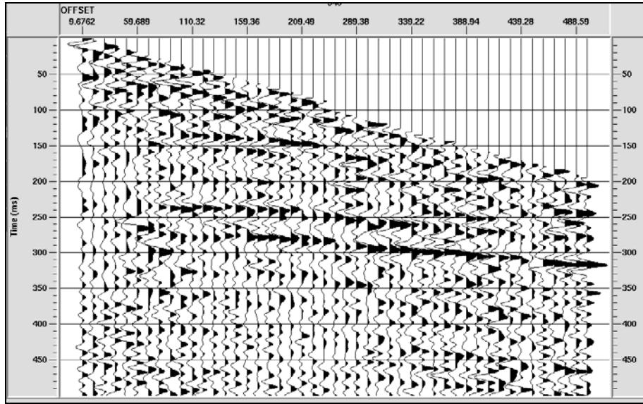
FIG. 7. Seismic record showing the coal event after Gabor deconvolution is applied in the xt and the rt domain. The figure shows vertical component data.
