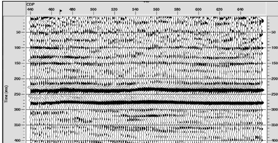
FIG. 9. Stacked vertical component data with Gabor deconvolution applied in the *xt* and *rt* domains.
