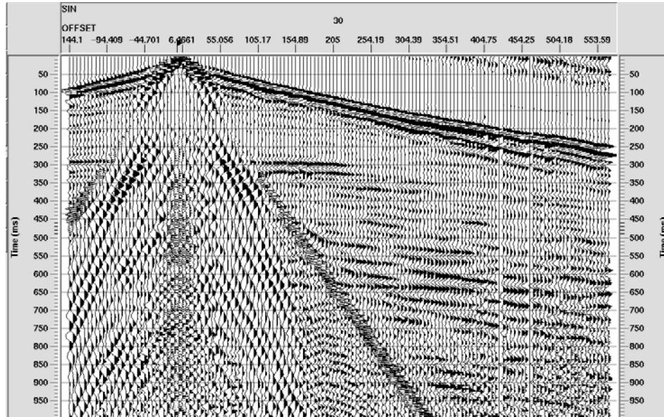
FIG. 4. A vertical component raw shot record. The coal events are between 250 and 400 ms.
