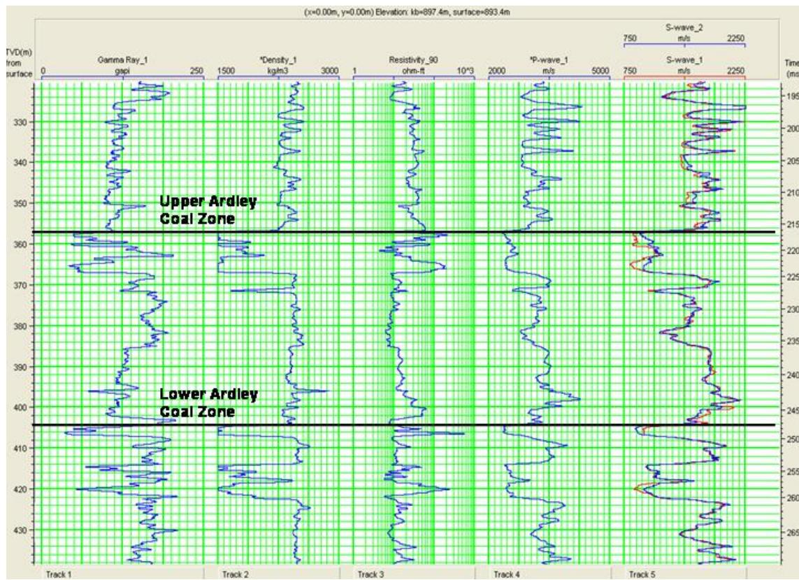
FIG. 2. The petrophysical logs from the injection well showing the Ardley Coal Zones. CO<sub>2</sub> injection will be into the Lower Ardley Coal Zone.
