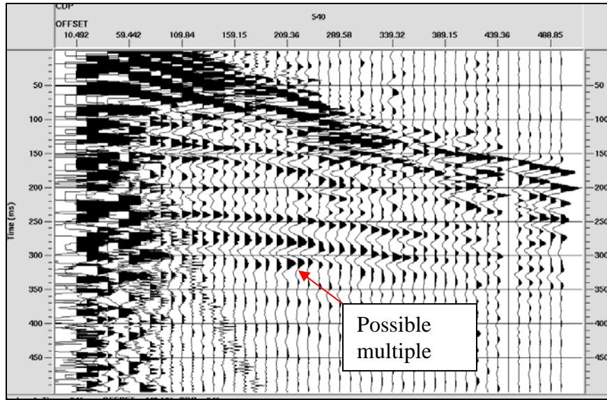
FIG. 6. Seismic record showing the coal events in a shot record after radial trace filtering. Note the possible inter-bed multiple just after 300 ms. The figure shows vertical component data.
