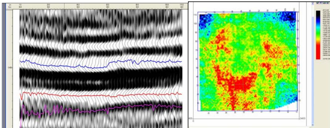
FIG. 16. On the left is an N-S section. The amplitude extracted from the blue horizon is shown on the right.
