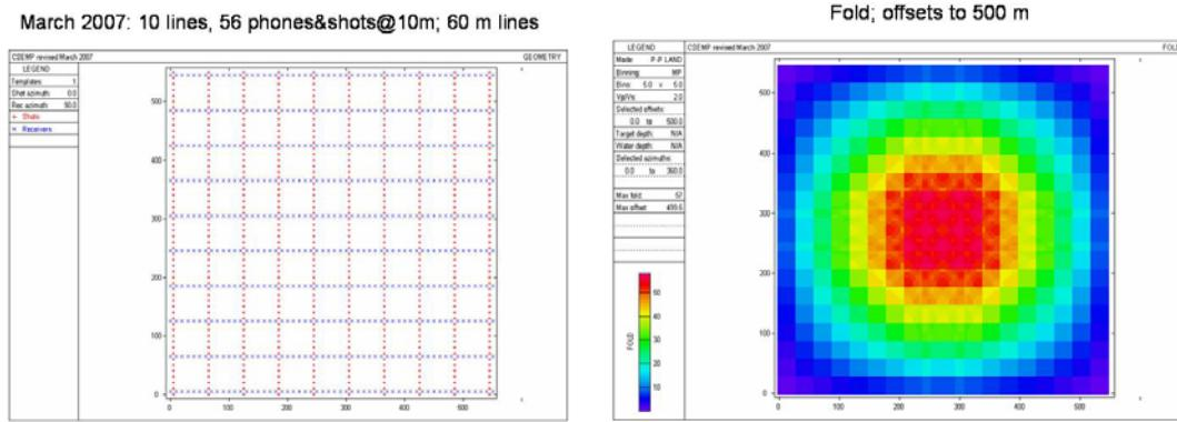
FIG. 13. On the left is the layout design for the vertical component 3D baseline 3D survey. Receiver lines run east-west and source lines run north-south. On the right is the expected fold for the PP survey.
