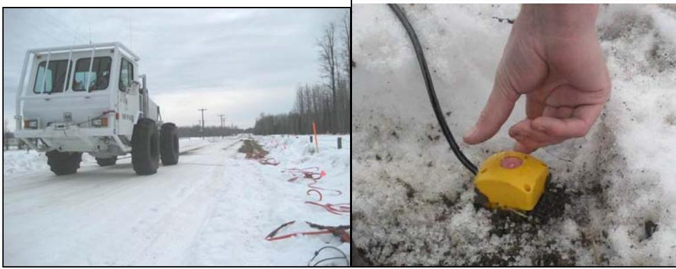
FIG. 3. Alder Flats 3C-2D survey. Vibe in action on the left and a tap test in progress on the right.
