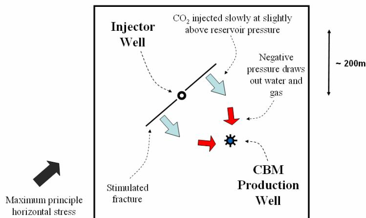
FIG. 1. Conceptual design of the ECBM and CO<sub>2</sub> storage pilot project.
