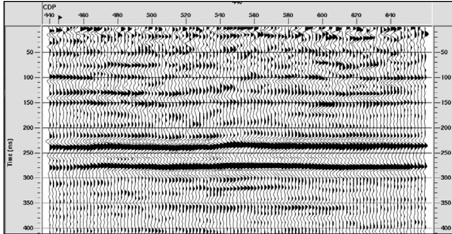
FIG. 8. Stacked vertical component data with Gabor deconvolution applied in the xt domain alone.
