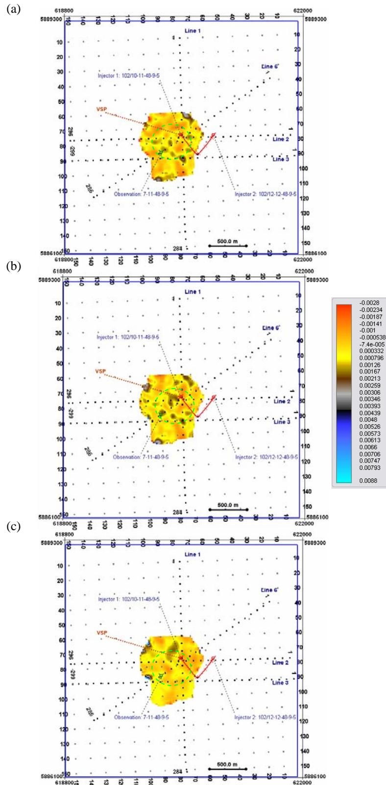
FIG. 13. The interval traveltim difference (scale bar in seconds) between the Ardley and the Viking horizons: (a) Phase II - Phase I, (b) Phase III - Phase I, and (c) Phase III - Phase II.
