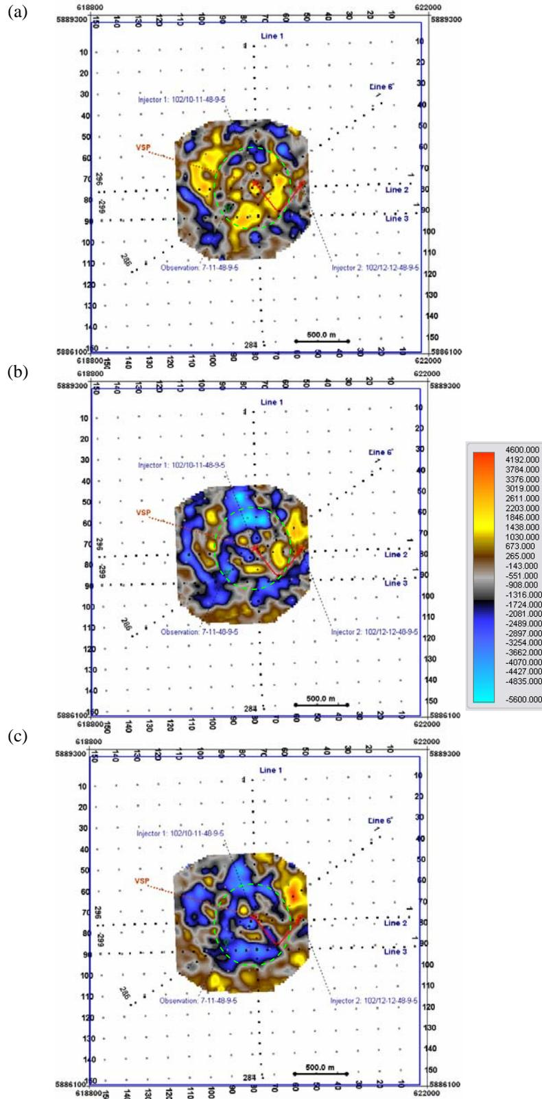
FIG. 11. The difference in the Cardium horizon amplitude (scale bar) between: (a) Phase II and Phase I, (b) Phase III and Phase I, and (c) Phase III and Phase II.
