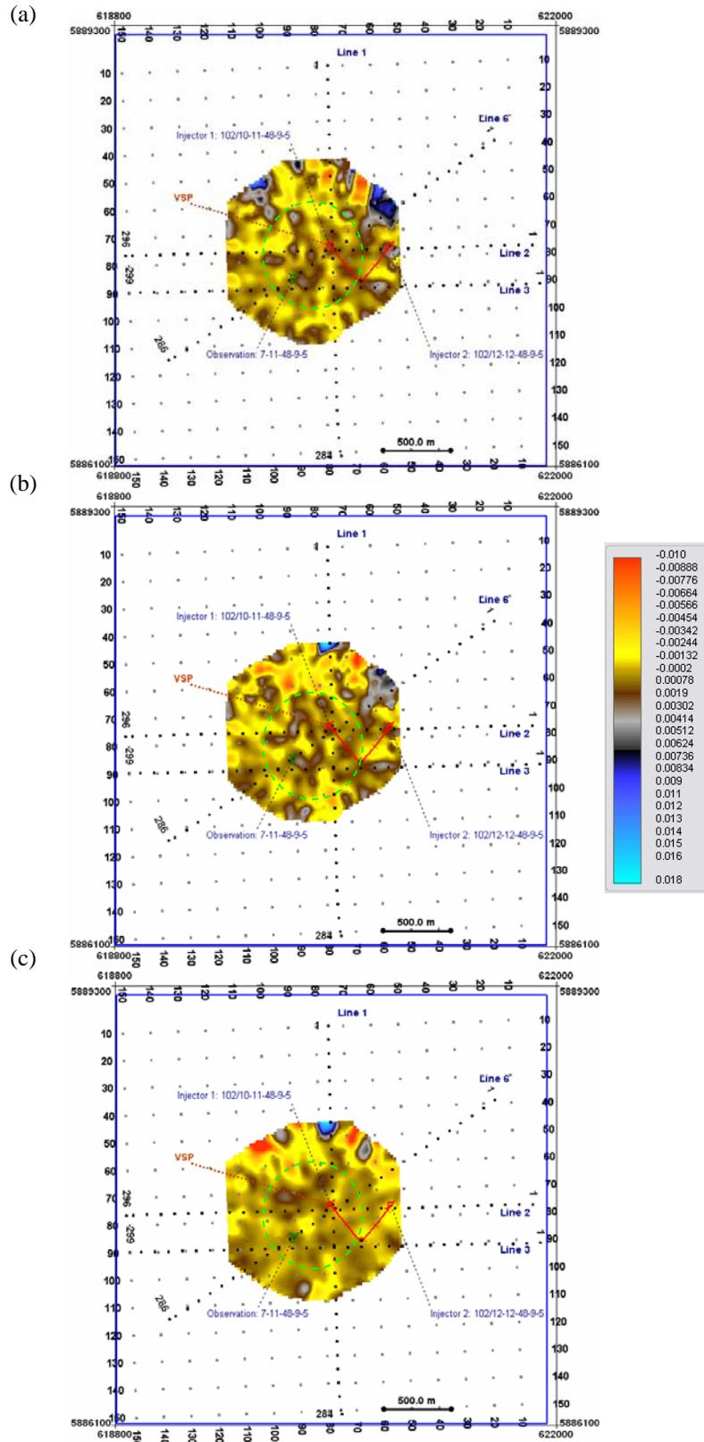
FIG. 14. The interval traveltim difference (scale bar in seconds) between the Lea Park and the Viking horizons: (a) Phase II – Phase I, (b) Phase III - Phase I, and (c) Phase III – Phase II.
