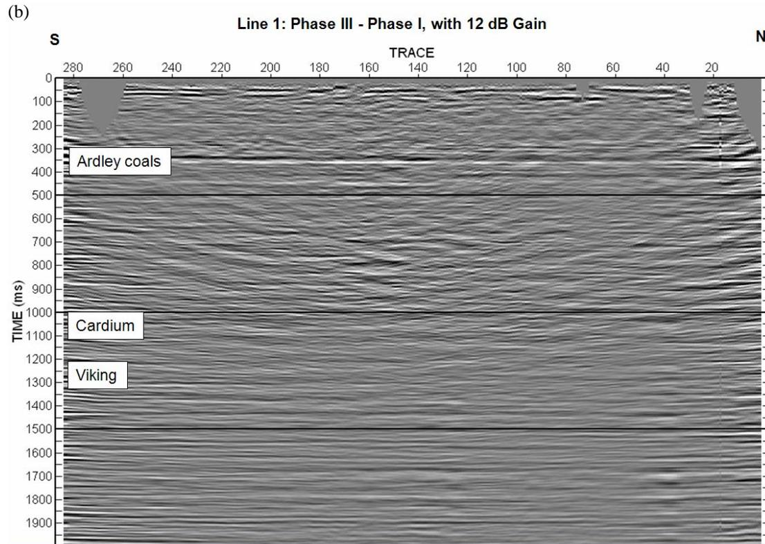
FIG. 6. The difference in Line 1 between Phase III and Phase I before (a) and after (b) applying 12 dB gain.
