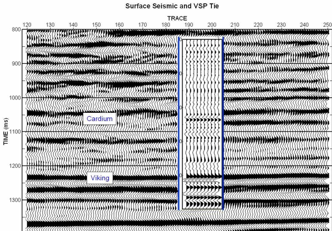
FIG. 8. Tie between surface seismic and VSP. Notice the better resolution capabilities of the VSP compared to surface seismic.
