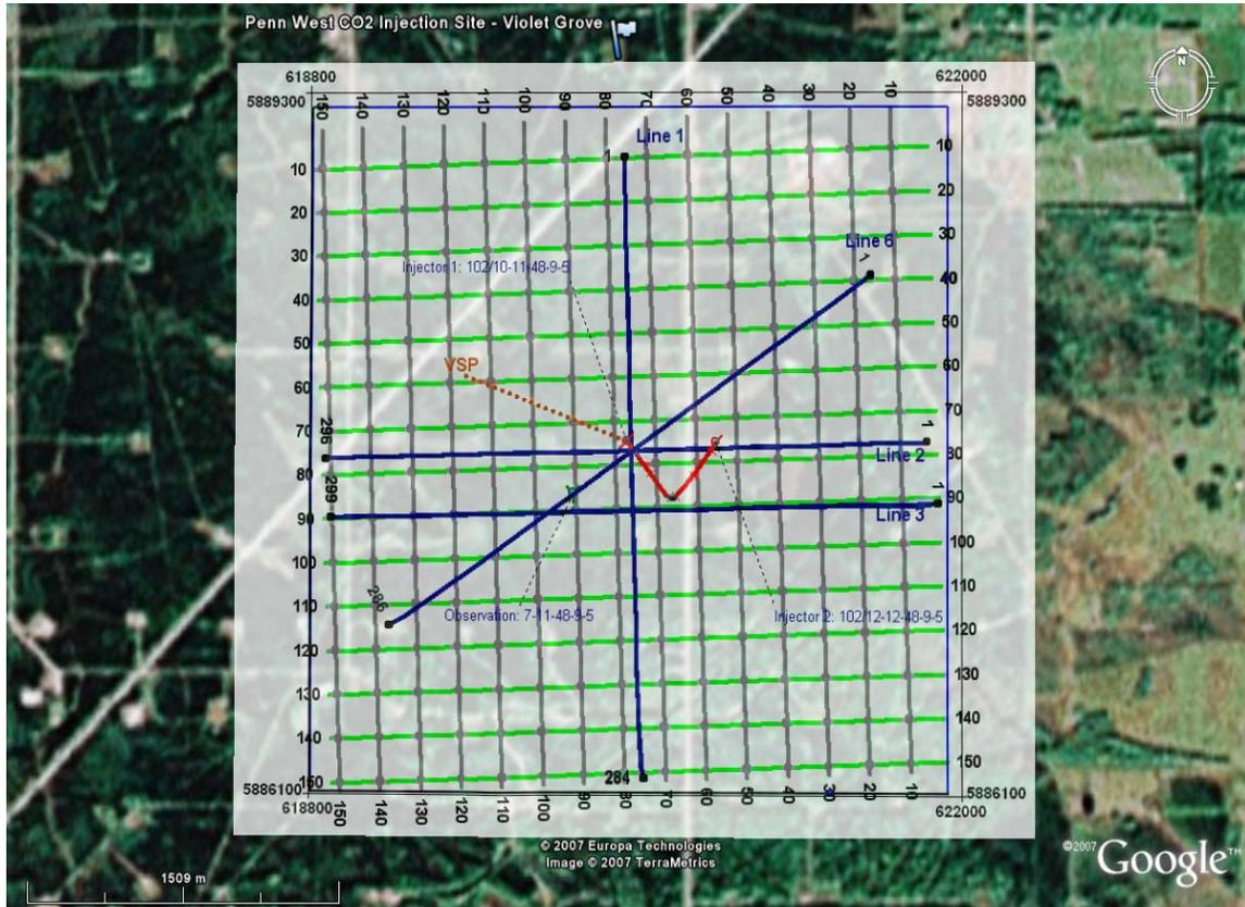
FIG. 2. Overview of the study area showing the seismic grid with locations of the 2D lines (dark blue) and the VSP (brown). The map, also, shows the injection and the observation wells. The map coordinates are UTM's (zone N11) with Northing along the vertical axis and Easting along the horizontal axis (aerial photo is courtesy of Google Earth®).
