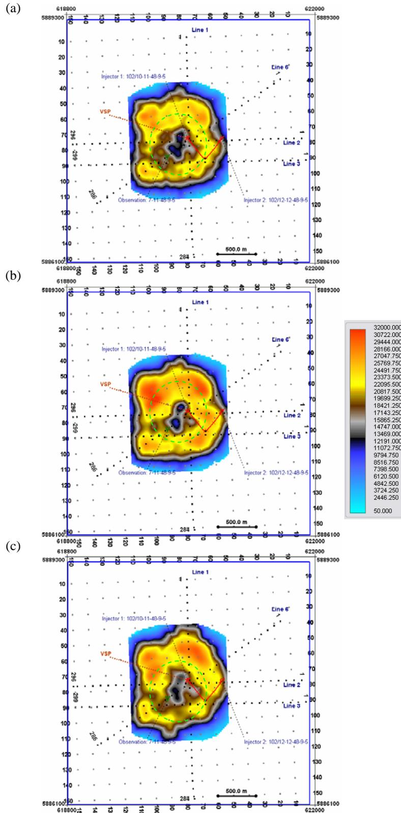
FIG. 12. The Viking horizon amplitude (scale bar) from: (a) the baseline survey (Phase 1), (b) the first monitoring survey (Phase II), (c) and the second monitoring survey (Phase III).
