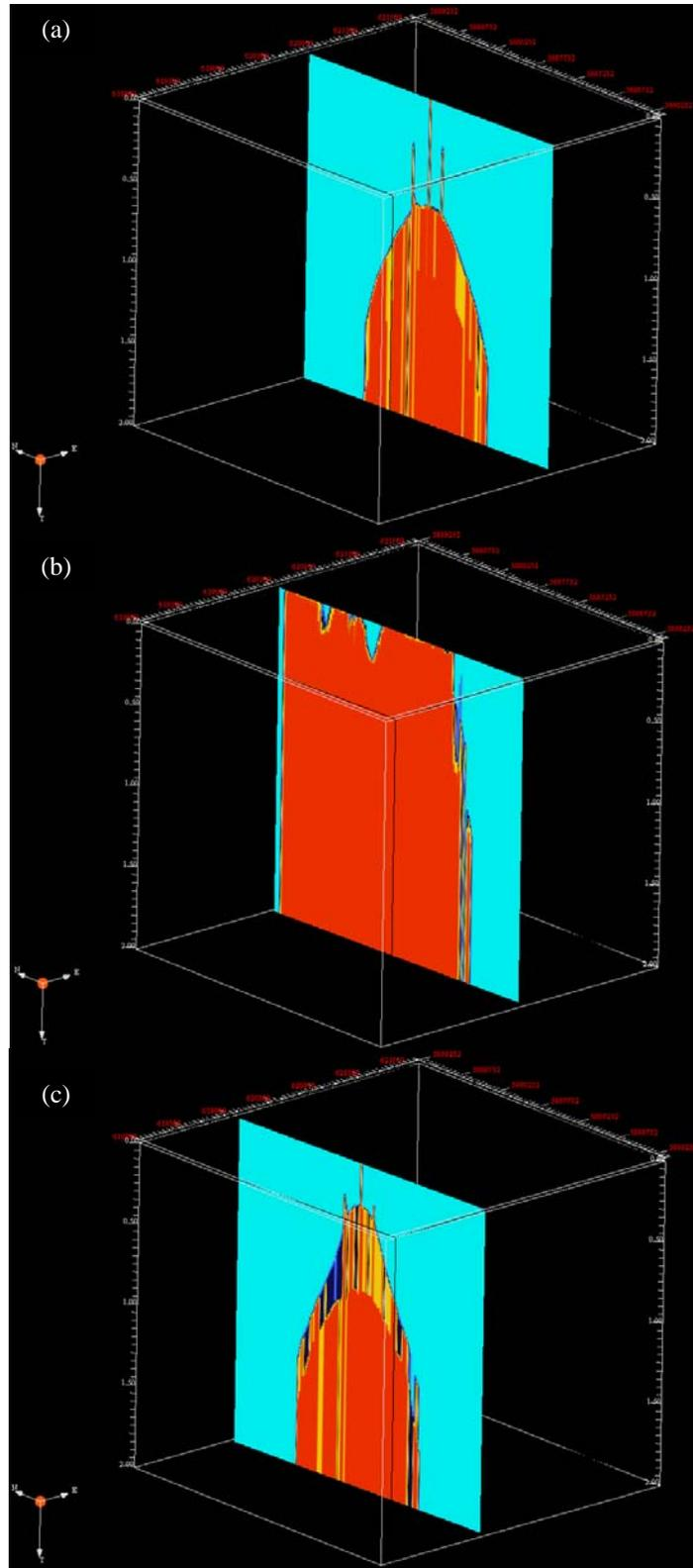
FIG. 4. Snapshots of the fold of the surface seismic data at the Penn West site: (a) inline 58, (b) inline 77 and (c) inline 100. Red color indicates high fold (60) whereas turquoise indicates low fold (0).
