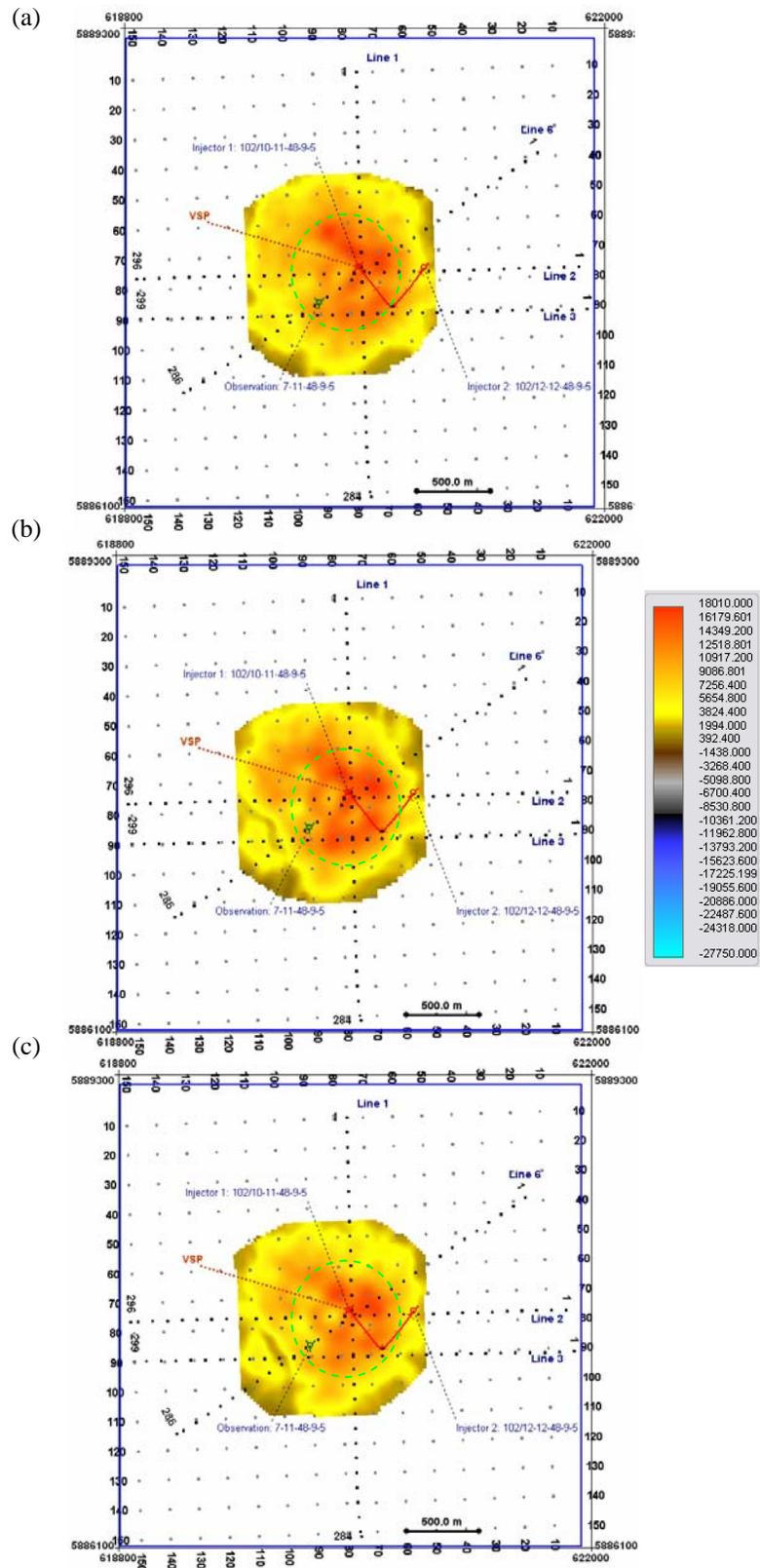
FIG. 10. The Cardium horizon amplitude (scale bar) from: (a) the baseline survey (Phase 1), (b) the 1<sup>st</sup> monitoring survey (Phase II), and (c) the 2<sup>nd</sup> monitoring survey (Phase III). Vertical scale is Northing and the horizontal scale is Easting in meters.
