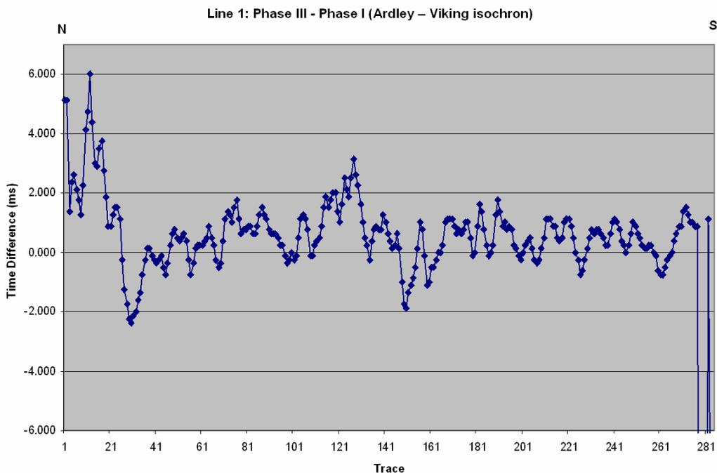
FIG. 7. The difference in the interval traveltimes (isochron) between the Ardley and Viking horizons between Phase I and Phase III (Line 1). Notice the increase in the interval traveltimes near trace 126.
