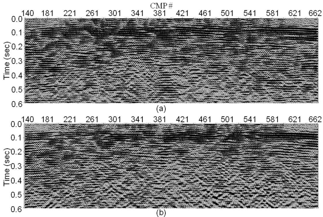
FIG. 5. Comparison of stacked sections in the radial channel for the conventional line data (top) and for the land streamer data (bottom). Zoom of the first 0.6 seconds.
