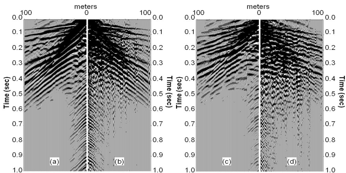
FIG. 3. Comparison of two raw shot gathers. In (a), half of a split spread record from the vertical component conventional line. The same shotpoint from the vertical component land streamer is shown on (b) with the lateral coordinate reverse to ease the comparison. The same comparison is done for the same record for the radial component of (c) the conventional line and of (d) the land streamer line.
