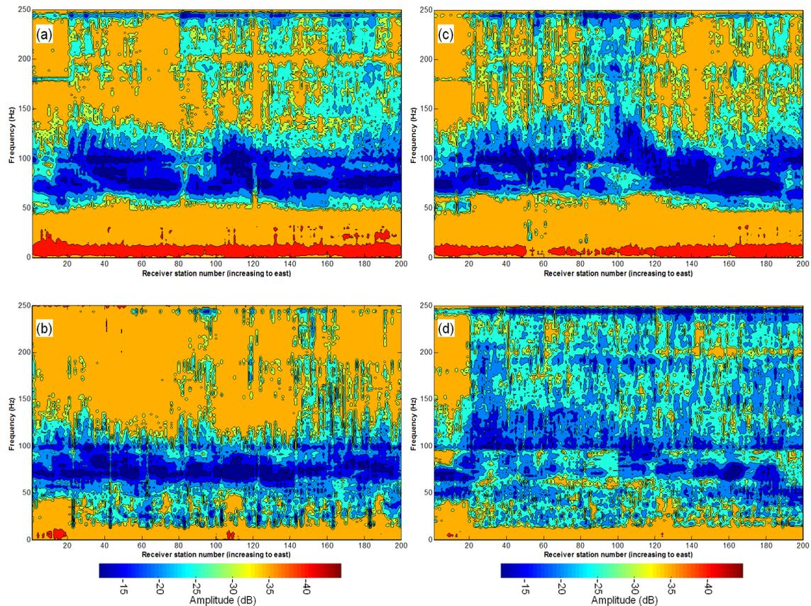
FIG. 9. Frequency Analysis of the common receiver gathers for both lines. In (a) and (b) is shown the resulted contour plot of the vertical channel conventional line and land streamer, respectively. In (c) and (d) is shown the same analysis but for the radial channel of the conventional line and land streamer data, respectively.
