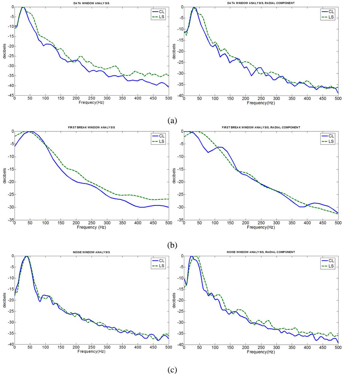
FIG. 6. Average Fourier amplitude spectrum of a raw shot gather for the vertical channel (left) and radial channel (right) of the conventional (CL) and land streamer line (LS), with windows corresponding to: (a) signal only area, (b) first break area and (c) groundroll/noise area.
