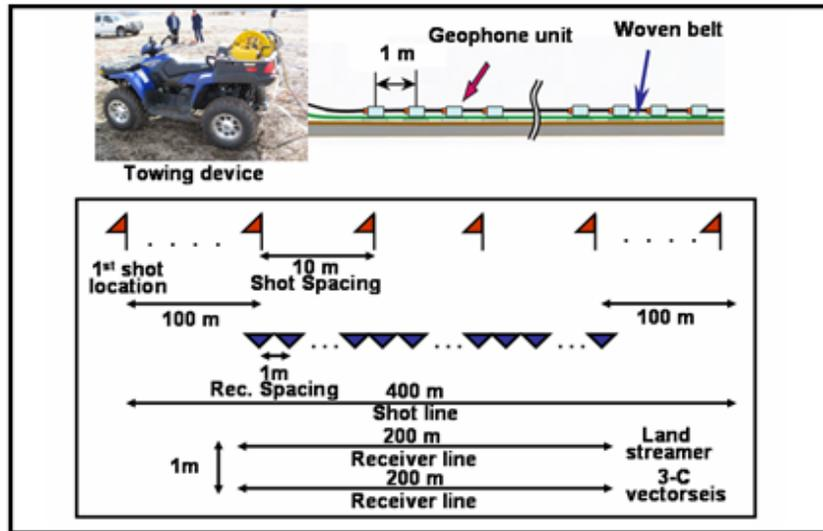
FIG. 2. Illustration of the land streamer configuration used on second (bottom) land streamer seismic experiment: a 20 m streamer with 3-C geophones separated 1 m, with a sledge hammer P-wave source located at 1 m off the cable (test 1) and a vibroseis source (test 2) (modified after Inazaki, 2006).
