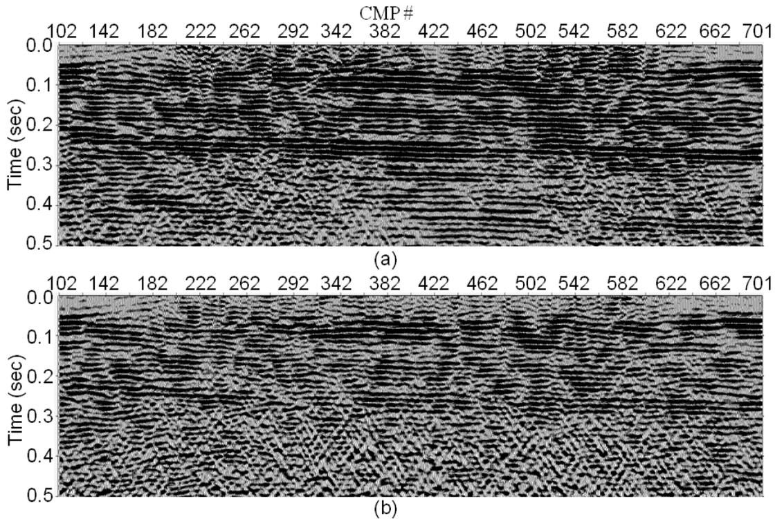
FIG. 4. Comparison of stacked sections in the vertical channel for the conventional line data (top) and for the land streamer data (bottom). Zoom of the first 0.5 seconds.
