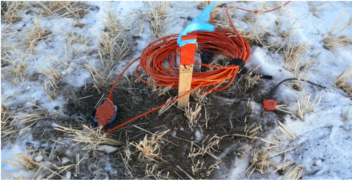
FIG. 2. DSU3 MEMS sensor on left, SM7 geophone on right (Photo courtesy Glenn Hauer).
