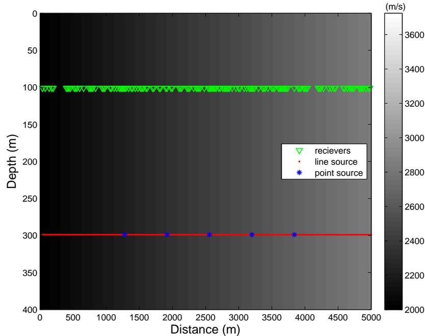
FIG. 1. The model setup used in the synthetic example. It simulates a line source (diamonds) and five point sources (large diamonds) and a highly irregular receiver array (triangles), (Ferguson, 2006).
