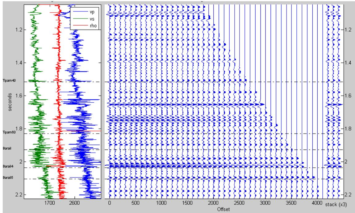
FIG. 9. PP synthetic seismogram for well B (Deohal field).
