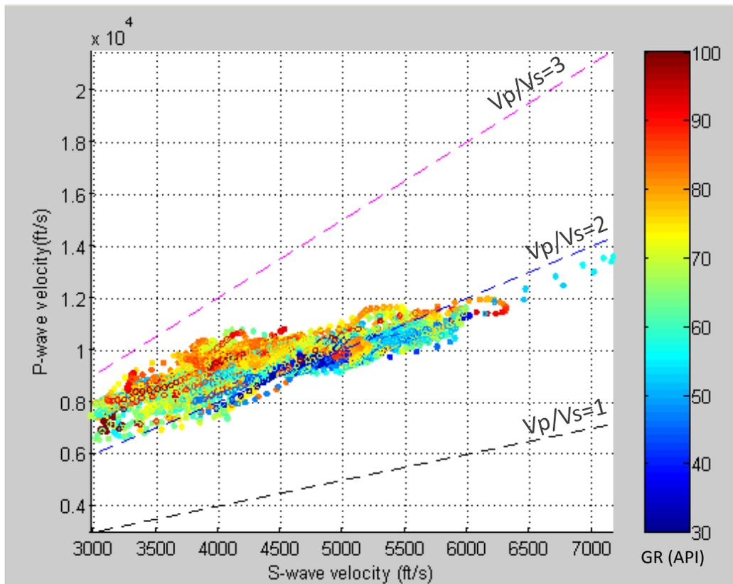
FIG. 8. Vp versus Vs cross plot for well B.
