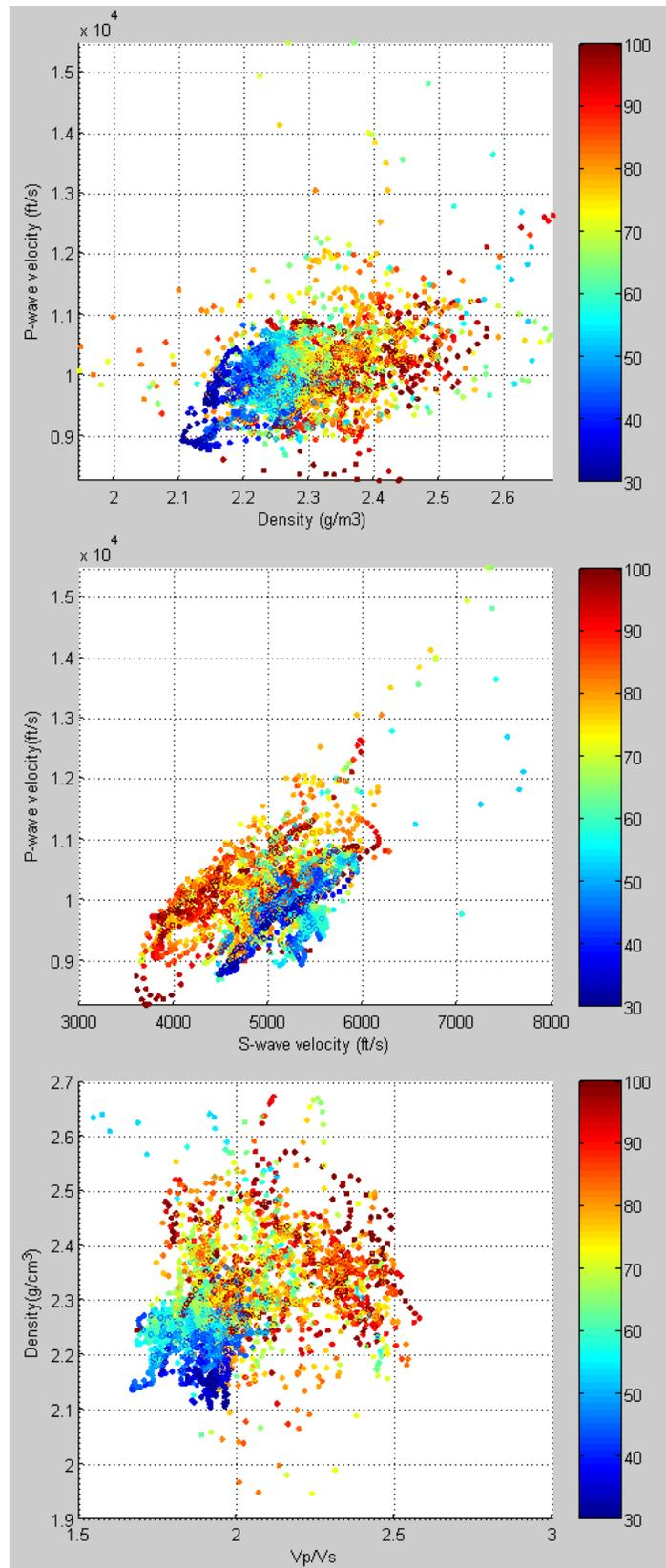
FIG. 6. Cross-plots for well A within the reservoir interval (2500-2800 m). Color bar indicates GR values.
