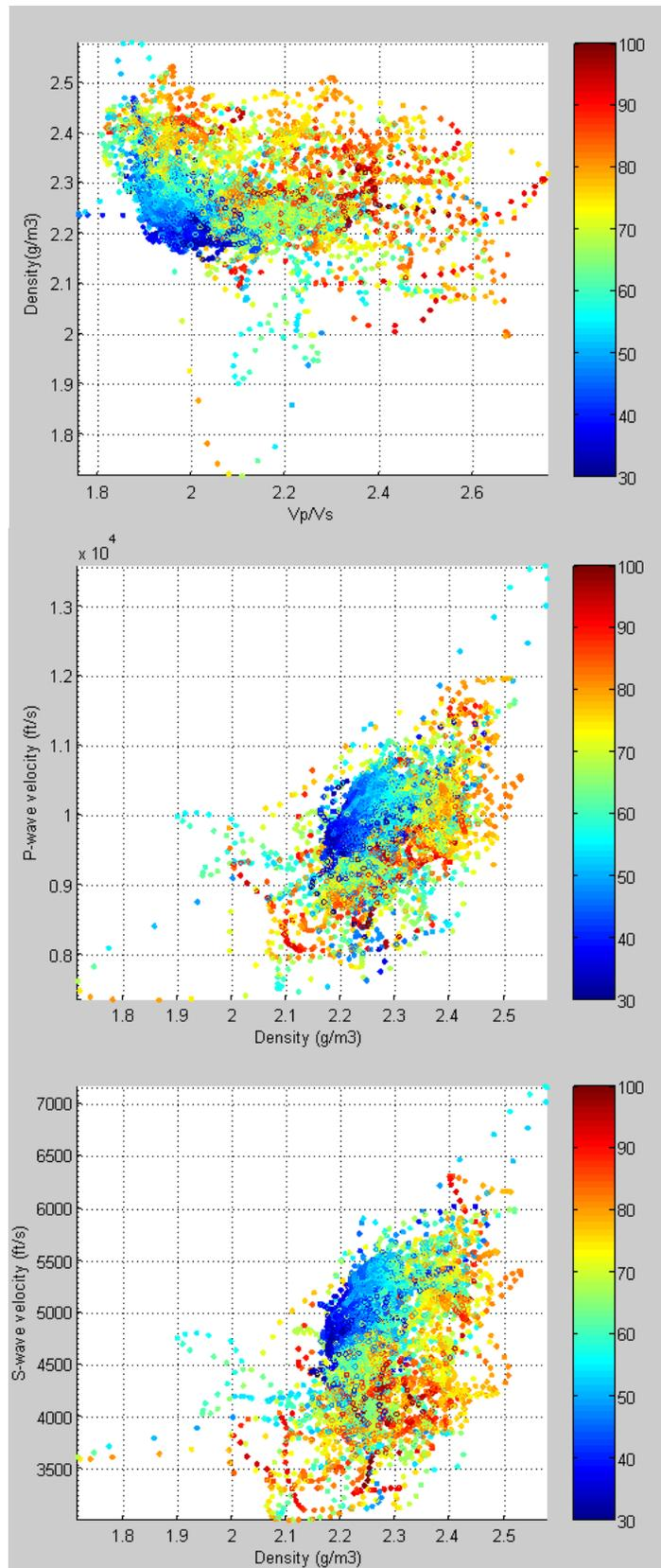
FIG. 7. Cross-plots for well B from 2200-2800 m depth. Color bar indicates GR values.
