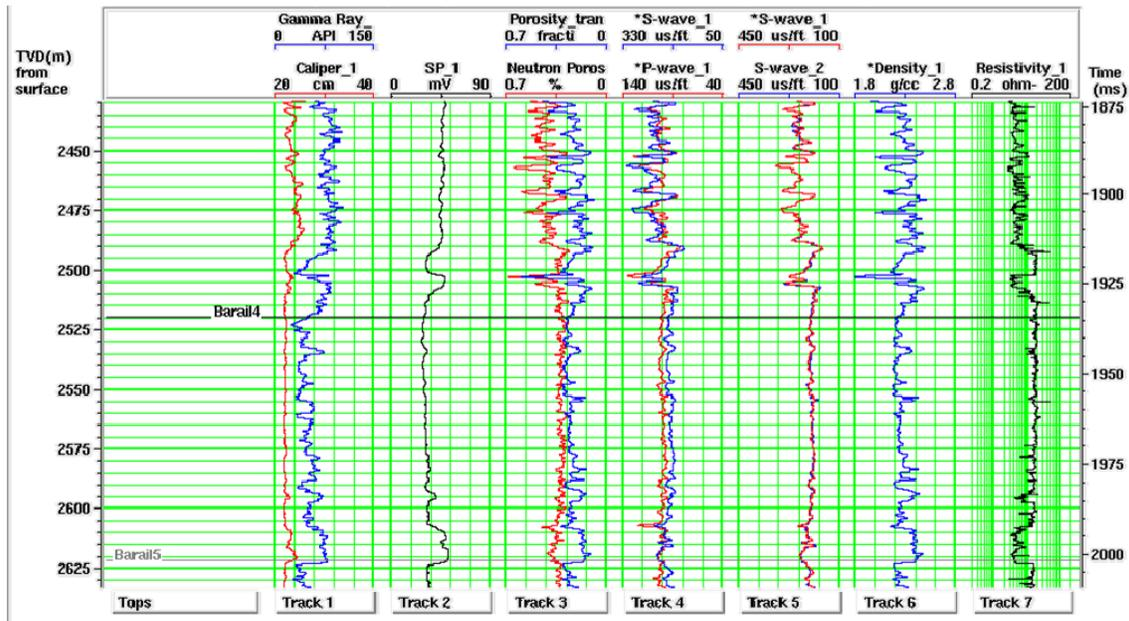
FIG. 4. Suite of logs for well B (Deohal field) at the Barail4 productive interval.
