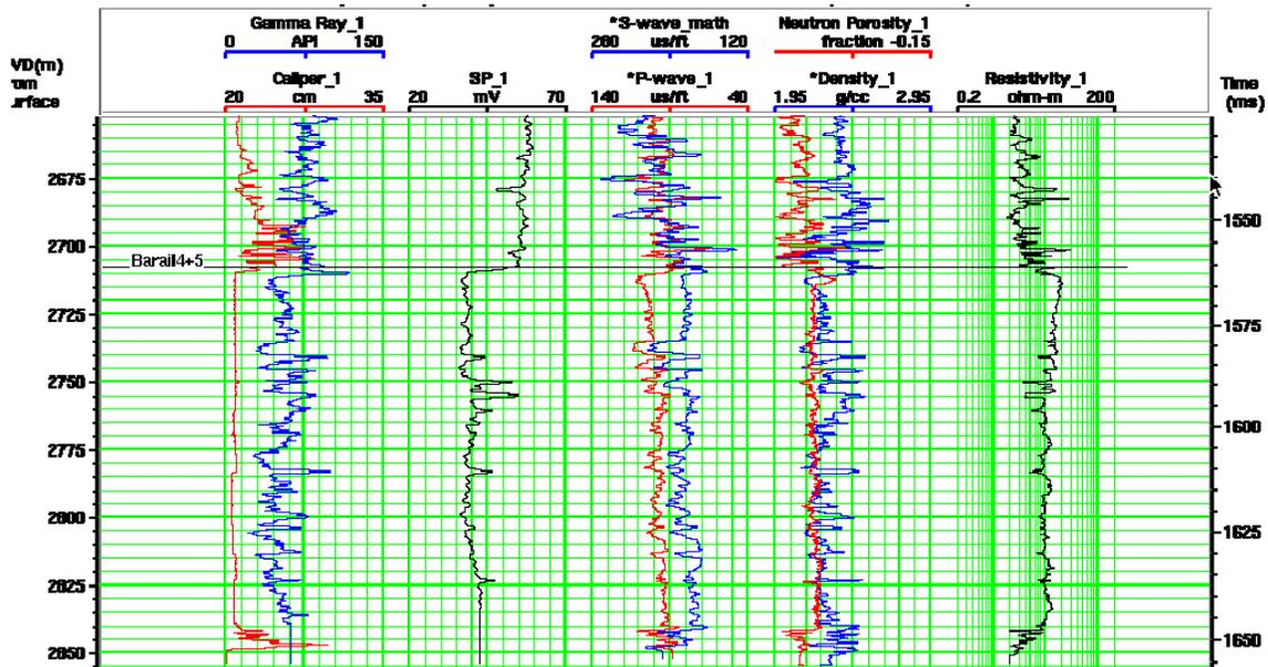
FIG. 5. Suite of logs for well A (Makum field) at the Barail4 and 5 productive interval.
