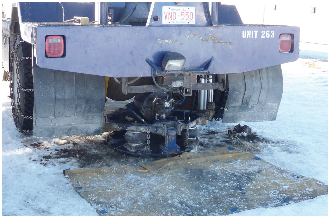
FIG 1. The MiniVibe unit belonging to the University of Alberta set in SV mode.
