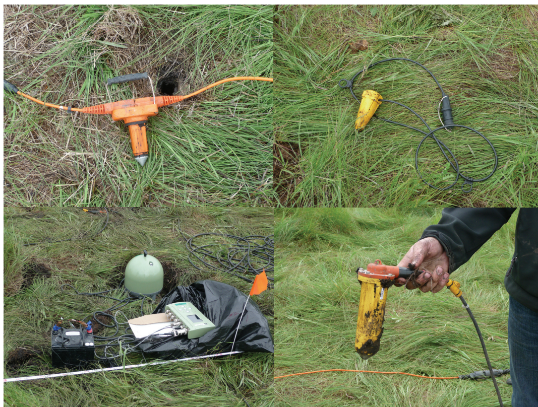
FIG 7. The four sensors used for the low frequency tests. From top left Sercel DSU3, Sensor SM24 three component geophone, ION Vectorseis, Nanometrics Trillium 240 seismometer.
