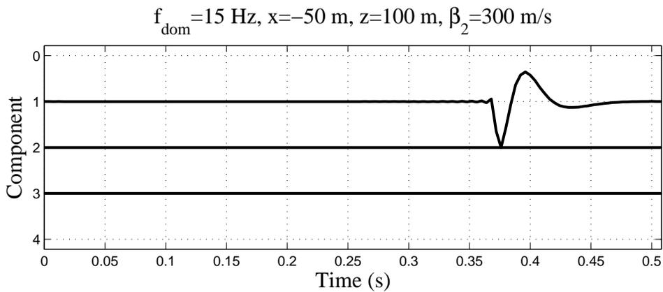
FIG. 2. Source waveform for an ideal S-wave source. Particle motion is in the X-line direction (component 1). No energy is present on the In-line and vertical components (components 2 and 3 respectively).
