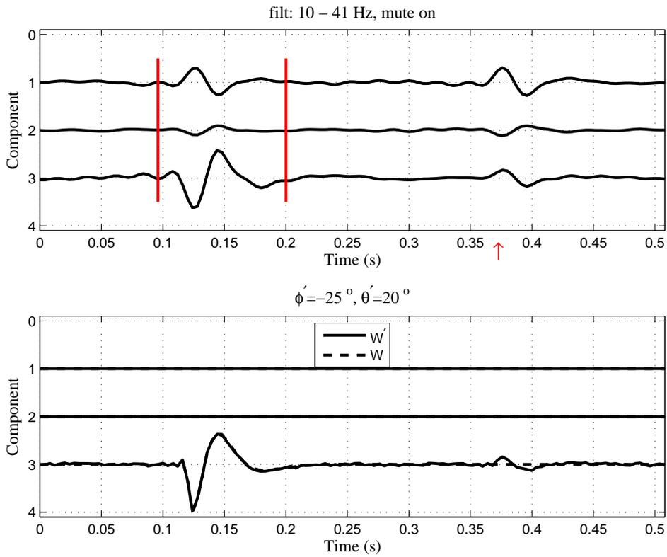
FIG. 7. Filtered version of the geophone recording in Figure 6a. a) 3C input. Red lines indicate the analysis window. b) The unfiltered inversion estimate.
