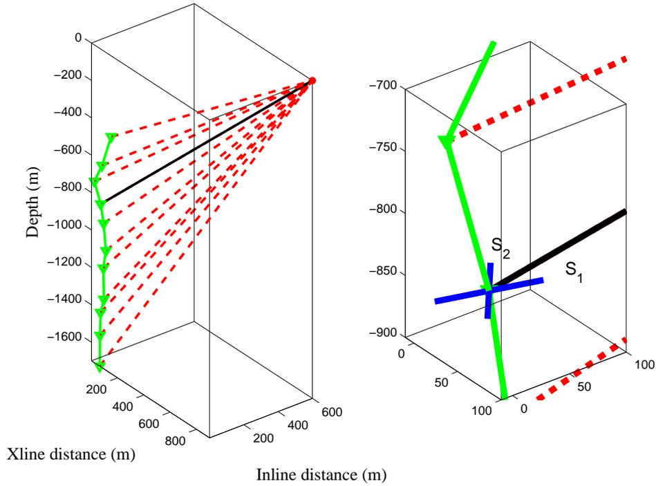
FIG. 1. An offset VSP into a deviated well. a) The deviated well is indicated by a green line, and geophones are indicated by green triangles. Source-receiver ray paths are indicated by dashed lines, and the source is indicated by a red asterisk. b) Close up of a tilted geophone. The orientation of the  $S_1$ , and  $S_2$  components are indicated by the blue lines. The  $Z$  component points along the well deviation.
