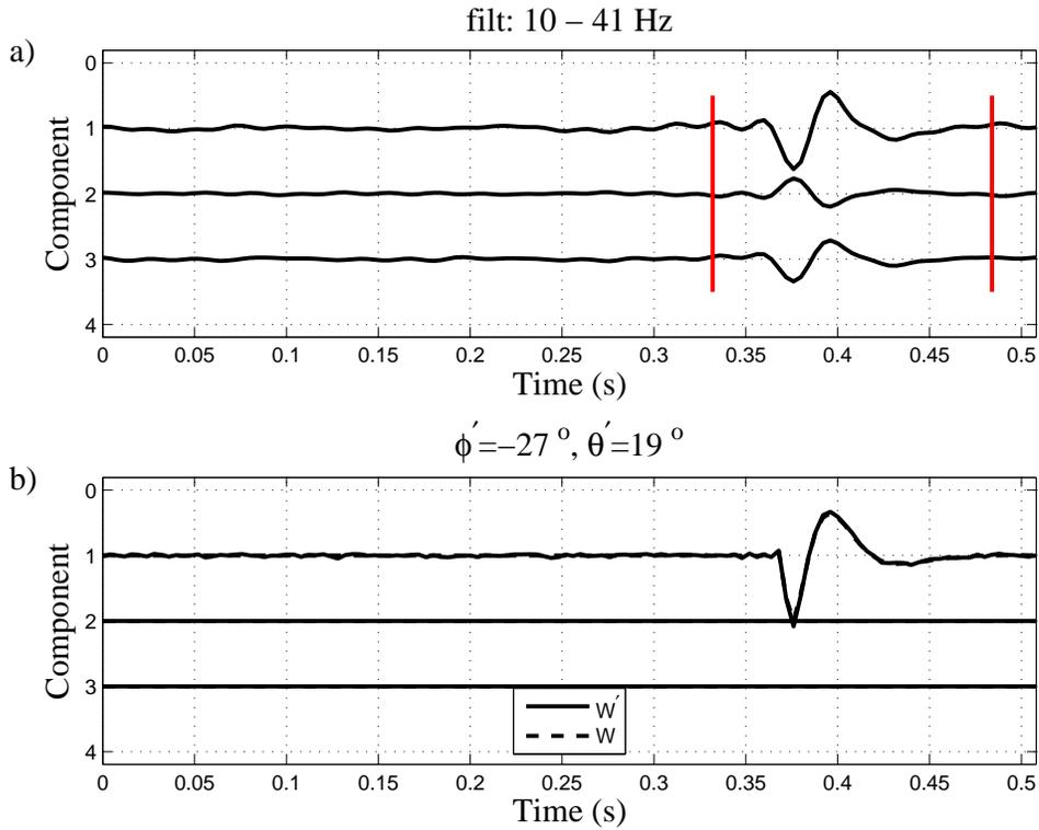
FIG. 4. Filtered version of the geophone recording in Figure 3a. a) 3C input. Red lines indicate the analysis window. b) Inversion estimates  $\phi = -27^\circ$  dip and  $\theta = 19^\circ$  ( $0^\circ$  and  $1^\circ$  error respectively) are much better than those from unfiltered inversion (Figure 3).
