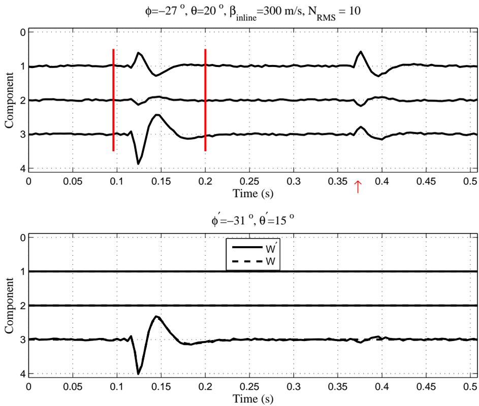
FIG. 6. Geophone recording corresponding to the P-wave source (Figure 5) plus random noise plus mode conversion. a) 3C input. Red lines indicate the analysis window, and the red arrow indicates the arrival time of the converted S-wave. b) The inversion estimate.
