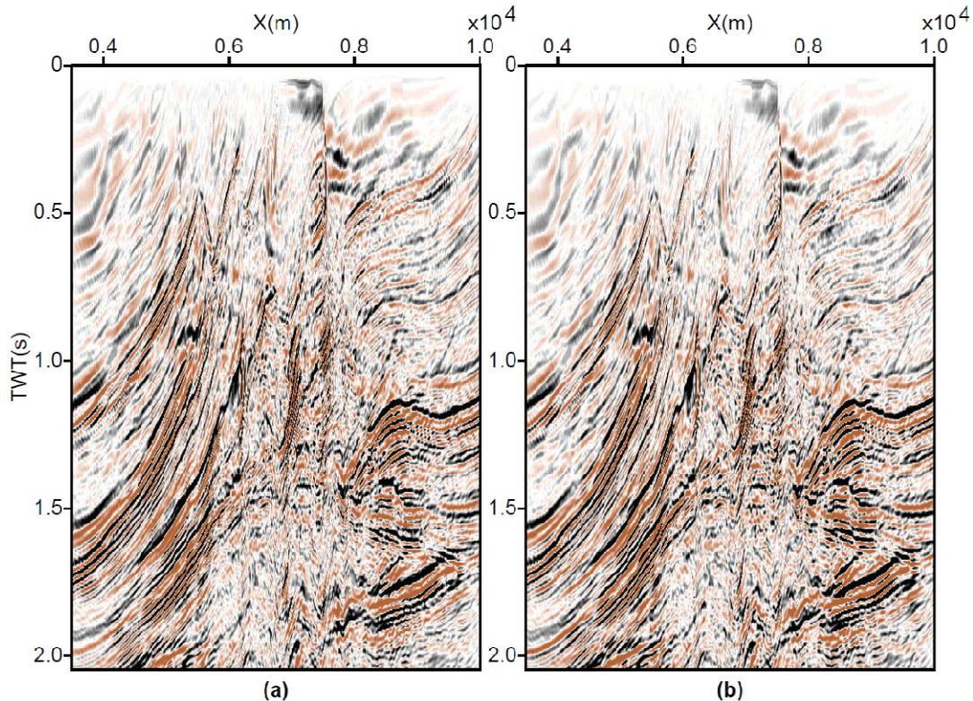
FIG. 12. Comparison between LSCG and multigrid LSCG to solve regularized LSPSTM of the Marmousi data set with 5 iterations on each grid. a) LSCG, b) Multigrid CG.
