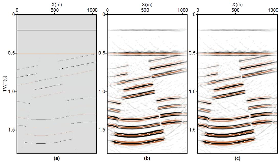
FIG. 10. Comparison between LSCG and multigrid LSCG for the synthetic model of figure 1, a) model, b) LSCG, c) Multigrid CG.
