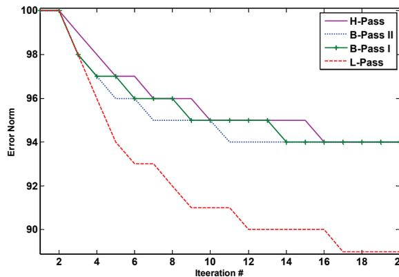
FIG. 9. Convergence of LSCG to solve LSPSTM for the filtered version of the Marmousi data set. L-Pass:  $f < 15\text{Hz}$ , B-Pass I:  $15\text{Hz} < f < 30\text{Hz}$ , B-Pass II:  $30\text{Hz} < f < 45\text{Hz}$ , H-Pass:  $45\text{Hz} < f$ .
