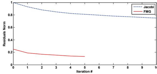
FIG. 5. The residuals norm error versus number of iterations is plotted for the weighted Jacobi iterations and full multigrid iteration in the last cycle. The FMG converges to %13 of the starting point in the residuals norm where Jacobi reaches %75 after 10 iterations.
