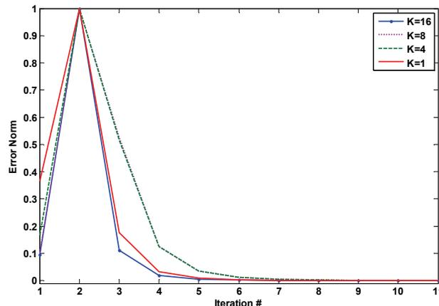
FIG. 7. The maximum norm error versus number of iterations is plotted for the CG iterations with different initial values. No relationship between rate of convergence and frequency content of initial value is visible.
