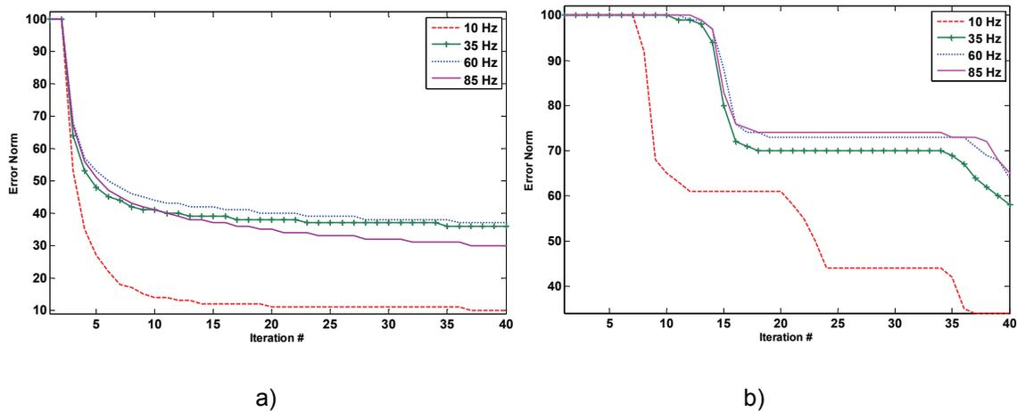
FIG. 8. a) Convergence of LSCG to solve damped LSPSTM for synthetic data of figure 1a with wavelets with different dominant frequencies: 10, 35, 60 and 85 Hz. b) Same result with regularized LSPSTM (smoothing in the offset direction).
