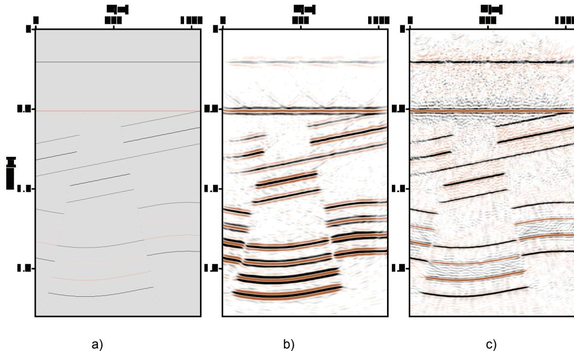
FIG. 1. a) Synthetic reflectivity model, 1.2 km length and 2 seconds depth. Background velocity linearly increases from 1300m/s at the top to 2300m/s at the bottom. b) Kirchhoff PSTM of the synthetic data from model in a). c) Kirchhoff LSPSTM after 20 iterations in the LSCG. Image of LSPSTM has higher resolution than standard migration.
