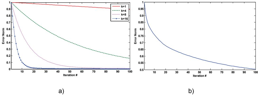
FIG. 3. a) The maximum norm error versus number of iterations for the weighted Gauss-Seidel method with different initial values. b) Convergence when initial values are superposition of the four Fourier modes with both low and high frequencies.
