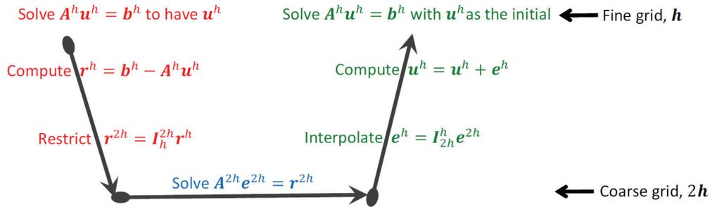
FIG. 4. Schematic v-cycle multigrid. Main problem is solved on the fine grid and residuals which are restricted to the coarse grid with two grids are used to solve equation in the coarse grid. Solutions are interpolated to the fine grid and used as the initial value for iterations on the main grid.
