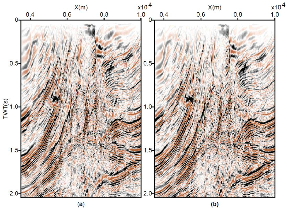
FIG. 11. Comparison between LSCG and multigrid LSCG to solve LSPSTM of the Marmousi data set with 2 iterations on each grid. a) LSCG, b) Multigrid CG.
