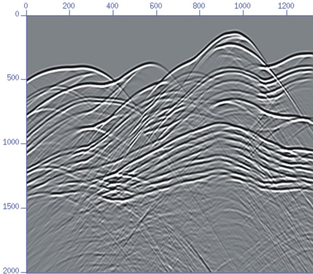
**Fig. 1.** The exploding reflector for the Grech-Spratt model represents an idealized stacked section. The section has 1350 traces with 2000 samples. Trace spacing is 25m and time sample interval is 2ms.
