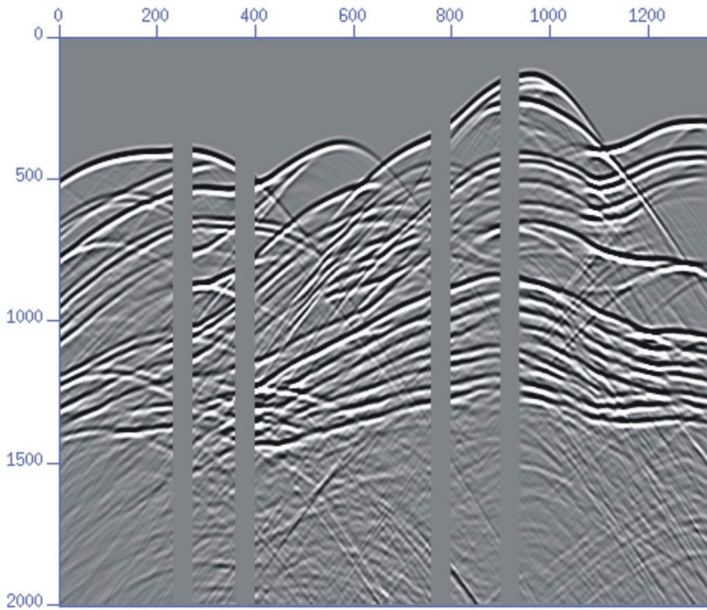
**Fig. 3.** Synthetic seismogram of model 1 with decimation for traces 233-272, 360-399, 760-799, and 930-999.
