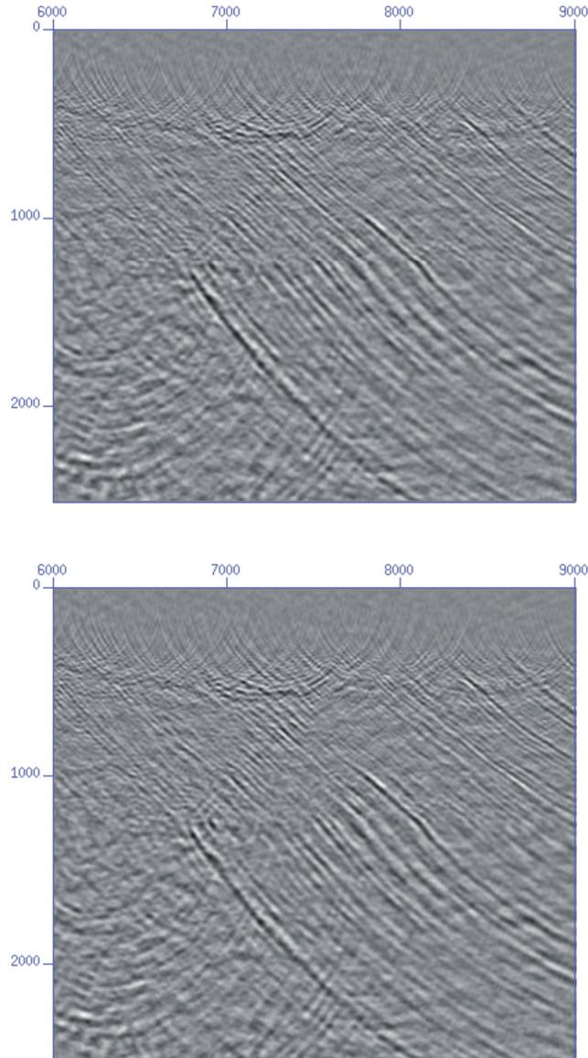
**Fig. 10.** Reverse-time migrations of the Shaw-Basing data for the highlighted zone. The top figure shows the migrated data for closely spaced samples in Figure 9. The bottom figure shows the migration of the same data with missing traces in the interval  $8125m-8312.5m$ .
