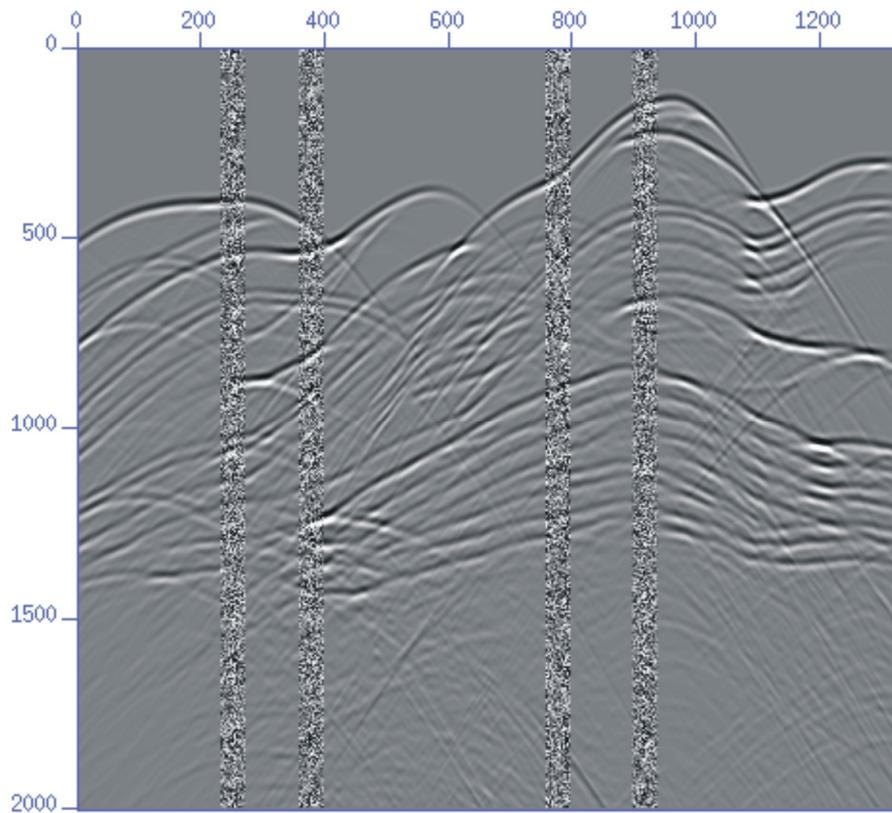
**Fig. 6.** Synthetic seismogram of model 1 with noise added to traces 233-272, 360-399, 760-799, and 930-999. Noise to signal ratio is 6.4 for these 160 traces.
