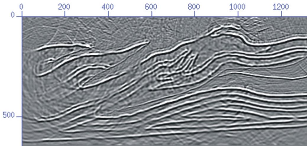
**Fig. 4a.** The reverse-time depth migrations of the data in Figure 3. We note blurring of reflections for footwall cutoffs beneath traces 233-272 and 360-399 and blurred anticlinal reflections between traces 900-939. Otherwise, the image is comparable to Figure 2.
