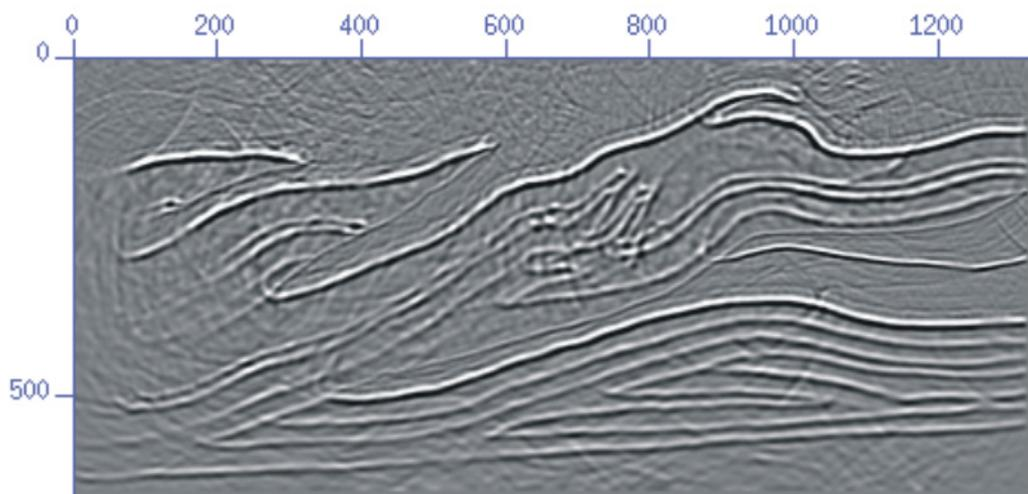
**Fig. 2.** Reverse-time depth migrated section of the stacked data in Figure 1. Spatial samples are separated by 25m intervals.
