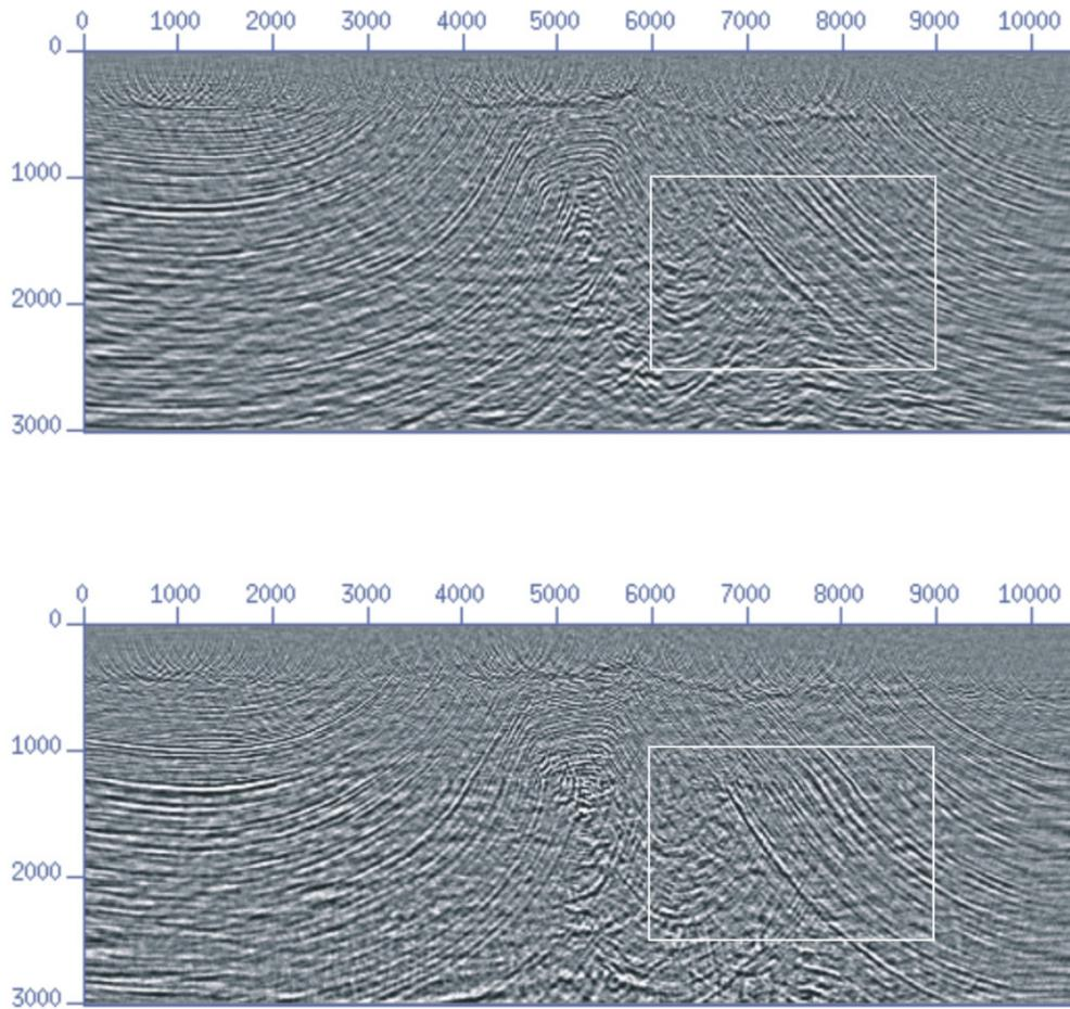
**Fig. 9.** Reverse-time migrations of the Shaw-Basing data with two different grid spacings. The upper section is migrated with grid spacing of  $12.5m$  and the lower section is migration with  $6.25m$ . The slopes on the backthrust (in the box) are more clearly defined and less aliased in the lower section.
