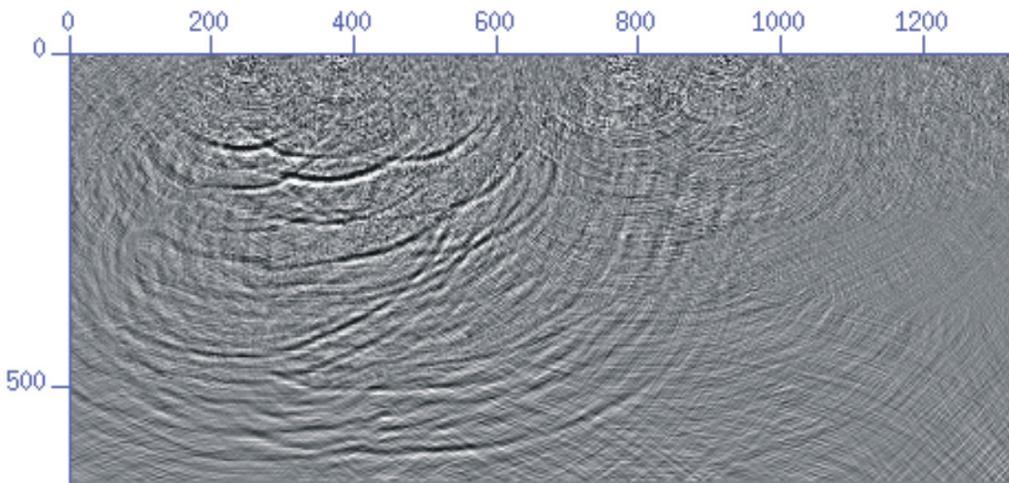
**Fig. 8.** The difference between the optimum RTM of Figure 2 and the RTM of the section with noisy traces, as shown in Figure 7.
